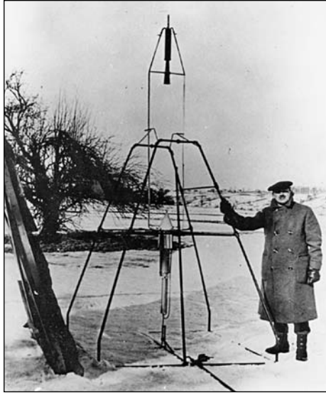
Figure 112. Robert Goddard posing with his liquid-propellant chemical rocket just before its first flight in March 1926. His first flight traveled only 184 feet across his Aunt Effie's farm to land in a cabbage patch, but it was as seminal as the Wright brothers' flight at Kitty Hawk.
