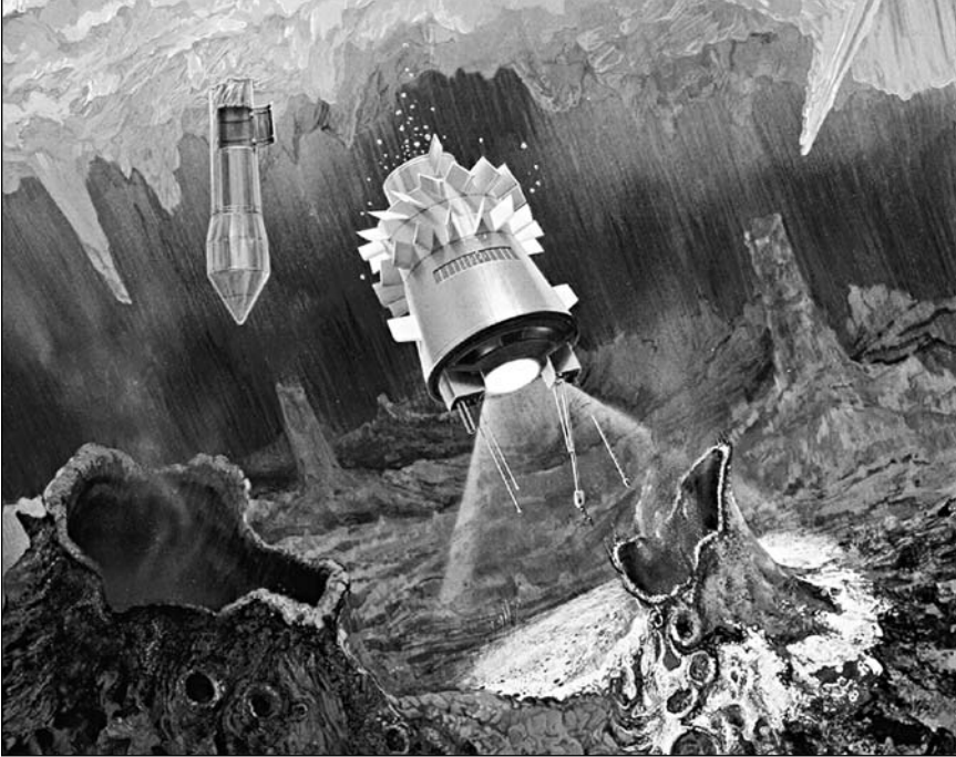
Figure 95. A hydrobot searches for life under the ice pack of Europa, in an artist's impression. A probe to Europa would land a cryobot, which would use nuclear power to melt its way through the ice pack. Then it would release an instrument-laden hydrobot that would search for life. The mission can be tested on the Earth using the analog environment of Antarctica's underground Lake Vostok.
