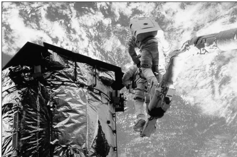
Figure 19. The Hubble Space Telescope during a routine servicing mission with the Space Shuttle. Astronauts work on the telescope while tethered to a robotic arm. Even though the 2.2-meter aperture of the HST is far exceeded by a dozen telescopes on the ground, the sharp images and low background levels of the space environment ensure it remains the most powerful tool in astronomy.
