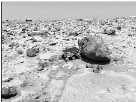
Figure 81. A close-up of the Martian surface, with the Sojourner rover, the "Little Rover That Could." The Sojourner rover was no bigger than a backpack, and it could travel at a speed of only two feet per minute. What it lacked in speed, it made up for in agility and endurance. Sojourner's power lasted twelve times longer than expected, and it took more than five hundred pictures of the rock-strewn surface. Scientists drove the rover from 120 million miles away using a computer screen, a joystick, and 3-D goggles.
