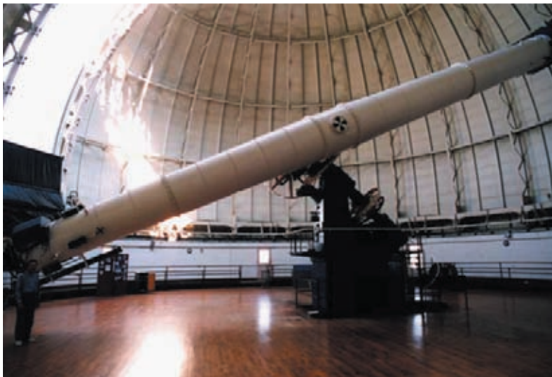
Fig 4.6. The 1 m refracting telescope at the Yerkes Observatory. Note the long distance over which the observer must move to keep up with the eyepiece. [Yerkes Observatory photograph]
