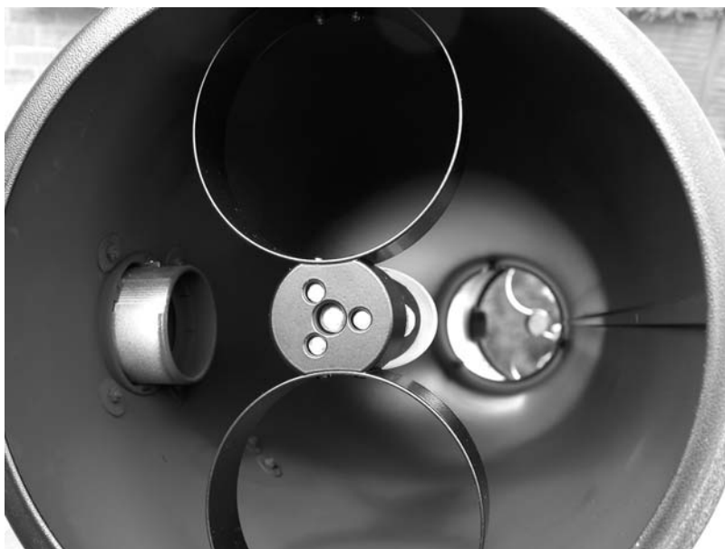
Figure 3.18. The unusual secondary mirror (spider) on the author's Orion Optics Newtonian. This design eliminates diffraction spikes around bright stars. Image: Martin Mobberley.
