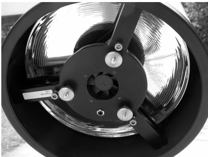
Figure 3.10. The cooling fan on the rear of the author's 250-mm f/6.3 Orion Optics Newtonian. The mirror is just over three centimeters thick and cools to within a fraction of a degree of the night air in under one hour of fan cooling. Image: Martin Mobberley.
