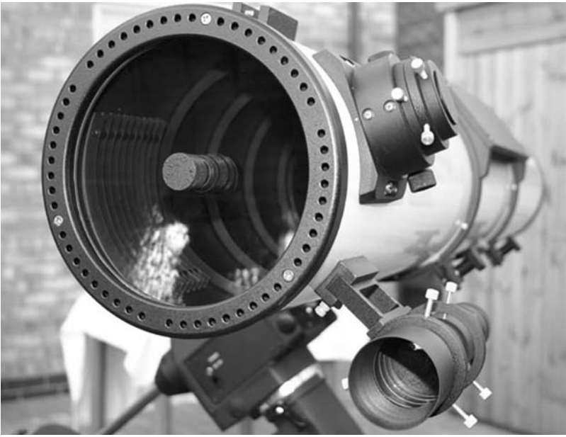
Figure 3.16. Another excellent planetary telescope: Intes Micro’s MN78, an 18-cm f/8 Maksutov Newtonian with a tiny secondary obstruction and closed tube. Image: Jamie Cooper.
