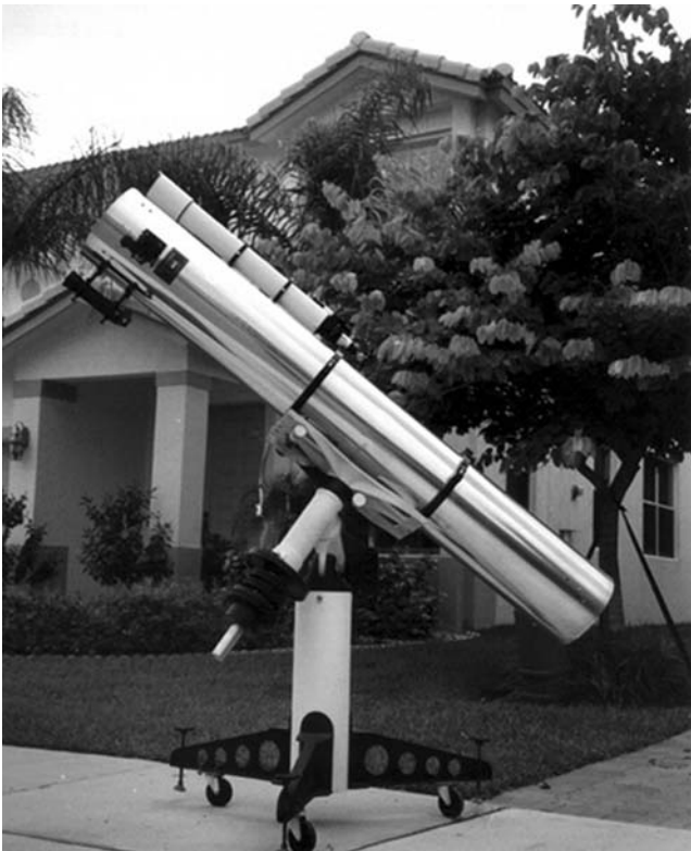
Figure 4.8. A telescope that raised the planetary imaging bar. Maurizio Di Sciuillo's 250-mm f/8 Newtonian featured excellent optics, a cork-lined tube, and a highly reflective outer skin. Image: Maurizio Di Sciuillo.
