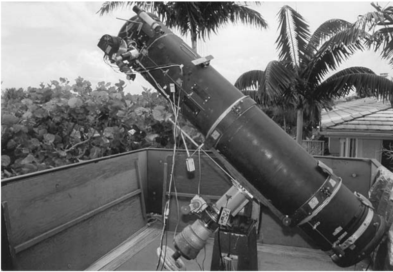
Figure 4.1. The 40-cm f/6 Newtonian of Donald Parker of Coral Gables, Florida. Possibly the most productive planetary telescope of all time and, rarely, it spans the eras of photographic, CCD, and webcam imaging! Image: Don Parker.
