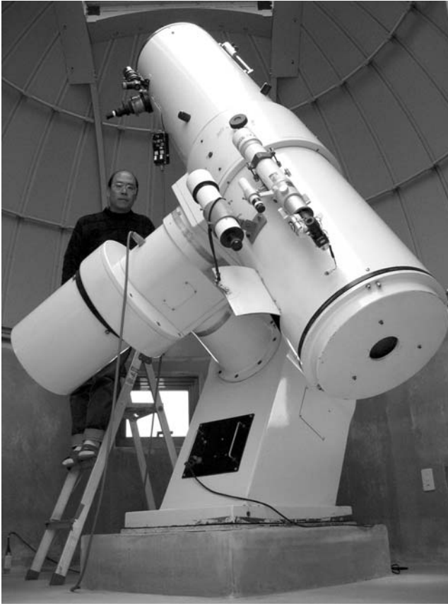
Figure 4.2. The magnificent 40-cm f/6 Newtonian of Isao Miyazaki of Okinawa, Japan. Miyazaki is one of the world's most experienced planetary observers. The telescope was built by Yasuyuki Nagata in 1988. The optics are by Ichirou Tasaka. Image: Isao Miyazaki.
