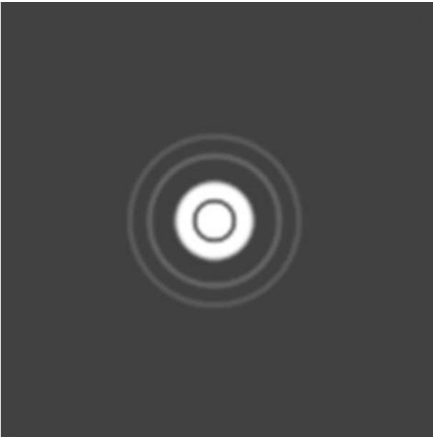
Figure 3.8. A perfectly focused star in a perfect telescope, with perfect collimation! A very high magnification is needed to see this view, along with a night of excellent seeing.
