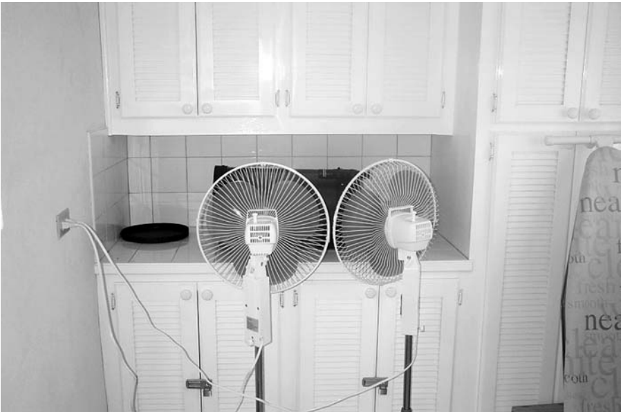
Figure 5.4. High daytime temperatures can necessitate some drastic cooling techniques on an optical tube that has become too hot. In this case, a Celestron 9.25 tube is being fan cooled indoors after getting too hot in Barbados. Image: Damian Peach.
