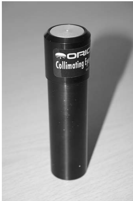
Figure 3.3A. The Orion (USA) Collimating eyepiece is, essentially, an accurately machined tube with a central sighting hold mounted within a bright metal disc. Image: Jamie Cooper.
