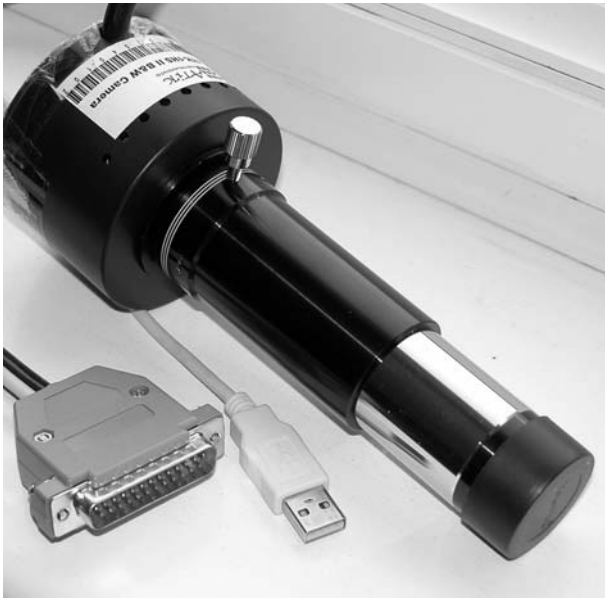
Figure 6.2. The author's monochrome ATiK 1HS super sensitive webcam. A low-cost way of taking planetary (USB) and Deep Sky (Parallel port) images. Image: Martin Mobberley.
