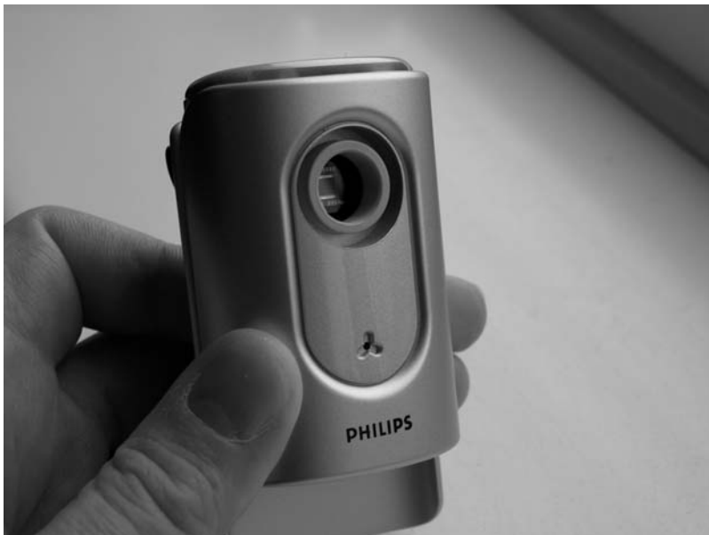
Figure 7.1. The Philips ToUcam Pro II with the supplied lens removed. The tiny CCD chip can just be seen. Image: Martin Mobberley.
