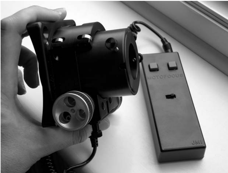
Figure 3.12. One of JMI's excellent motorized focusers. This one is an NGF DX designed for Newtonians. Focusing "shake" is eliminated with this design. Image: Martin Mobberley.
