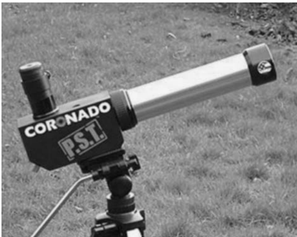
Figure 16.6. The Coronado PST. A 40-mm aperture f/10 H-Alpha telescope for under $500! Image: Maurice Gavin.
