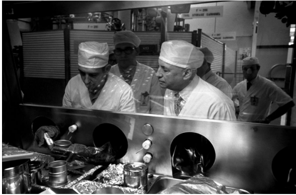
Figure 8.10 The Lunar Receiving Laboratory was built at NASA's Johnson Space Center as a containment facility in which to store and analyze the lunar samples without cross-contamination. Similar laboratory designs are being evaluated for the return of samples from Mars. (NASA/JSC.)
