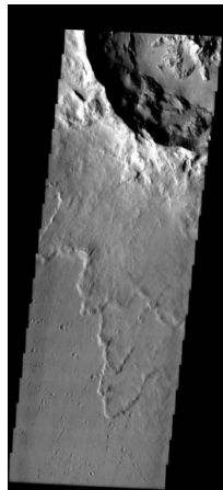
Figure 5.10 Ejecta blankets can be divided into continuous and discontinuous parts. This image of the ejecta blanket associated with a 28.3-km-diameter crater located at 23.2°N 207.8°E shows the layered continuous ejecta blanket extending outward from the rim. Beyond the edge of the layered ejecta blanket, small secondary craters are seen, which constitute the discontinuous ejecta blanket. (THEMIS image V01990003, NASA/ASU.)
