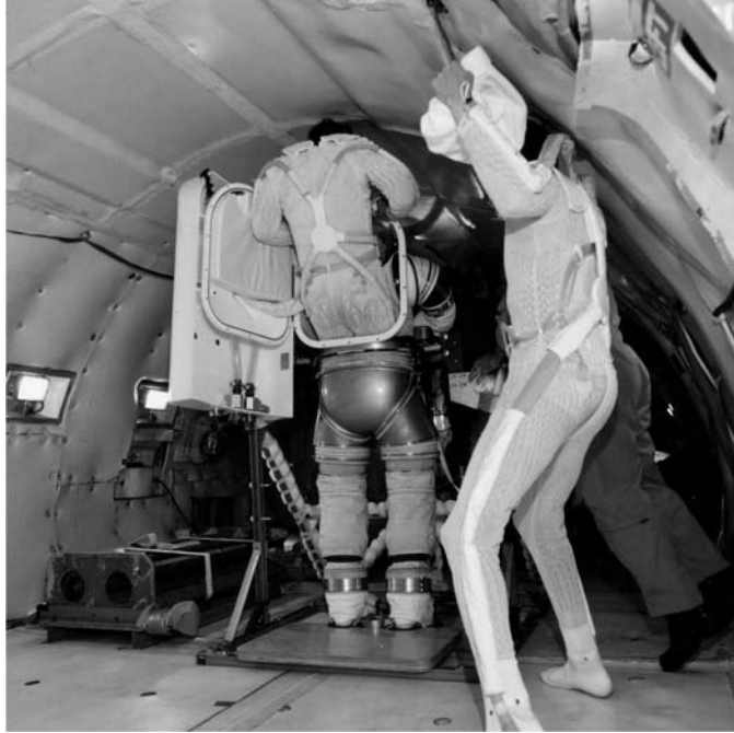
Microgravity evaluation, in the KC-135 aircraft, of a rear entry pressure suit.
