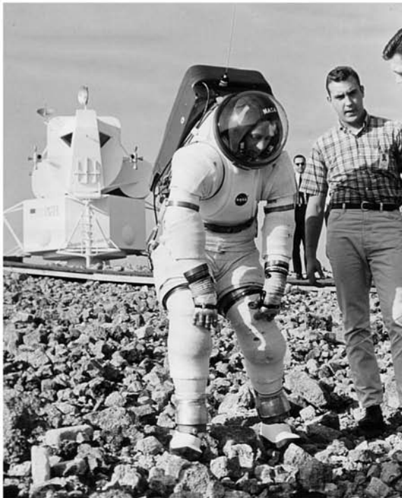
Designs for an advanced Apollo suit undergoing simulated EVA tests in the 1960s.
