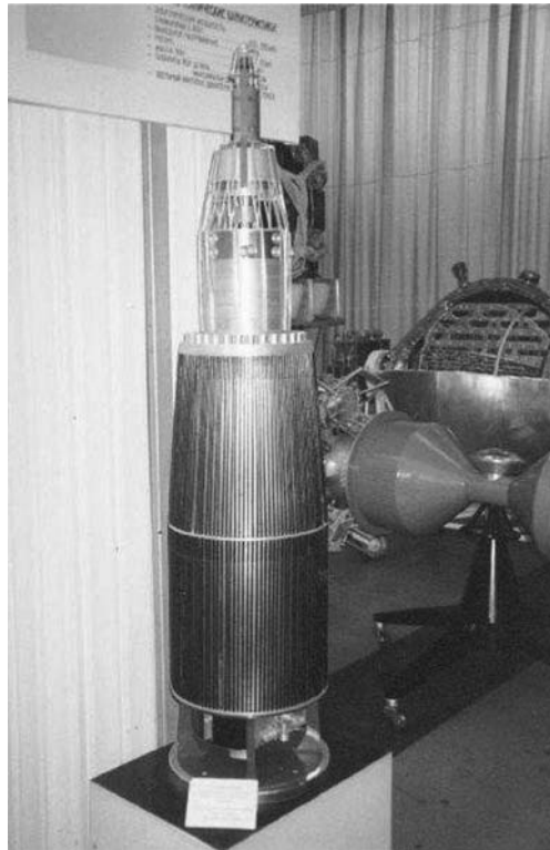
A nuclear-ion engine proposed by Korolev’s OKB-1 design bureau for use on a Soviet manned mission to Mars. (Model at TsNII Mash, Korolev; photograph by Andrew Salmon.)
