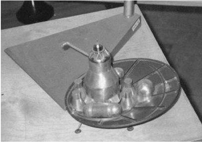
Aerobraking design for a Mars shuttlecraft to travel from the interplanetary craft into the martian atmosphere for a surface landing. (Model at TsNII Mash, Korolev; photograph by Andrew Salmon.)
