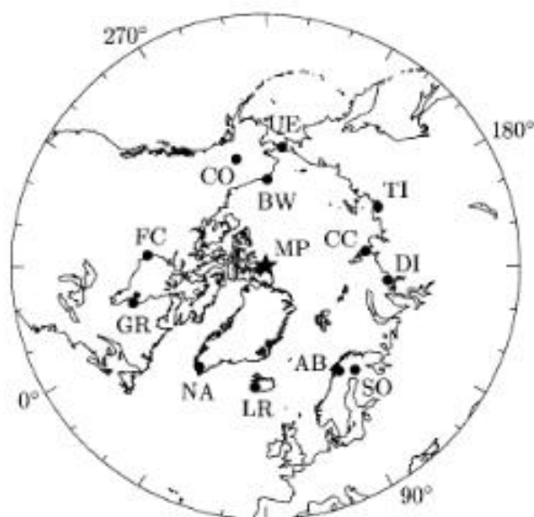
Fig. 8.7. Locations of the magnetic observatories contributing to the auroral electrojet indices (1974). Abbreviations: NA = Narsarsuaq, LR = Leirvogur, AB = Abisko, SO = Sodankyla, DI = Dixon Island, CC = Cape Chelyuskin, TI = Tixie Bay, UE = Cape Ulen, BW = Barrow, CO = College, FC = Fort Churchill, and GR = Great Whale River. The position of the magnetic pole (MP) is marked by a star and the magnetic longitude is denoted around the perimeter of the circle.
