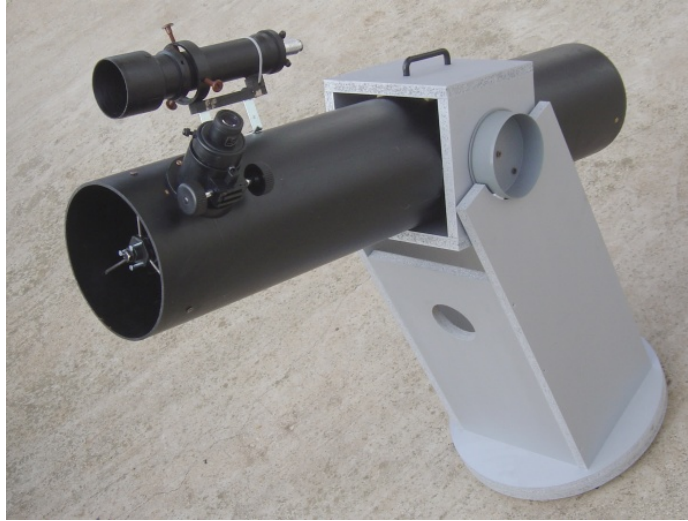
The finished 150 mm Dobsonian telescope
