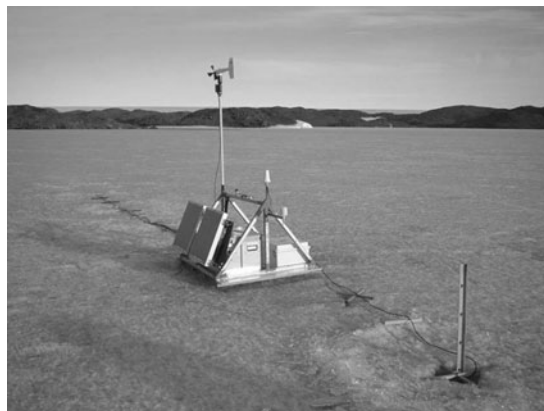
Figure 17.1 Wireless remote-sensing platform on Crooked Lake, Antarctica. Note the cables running out from the platform that support light and temperature sensors suspended in the water column (Palethorpe et al. 2004).
