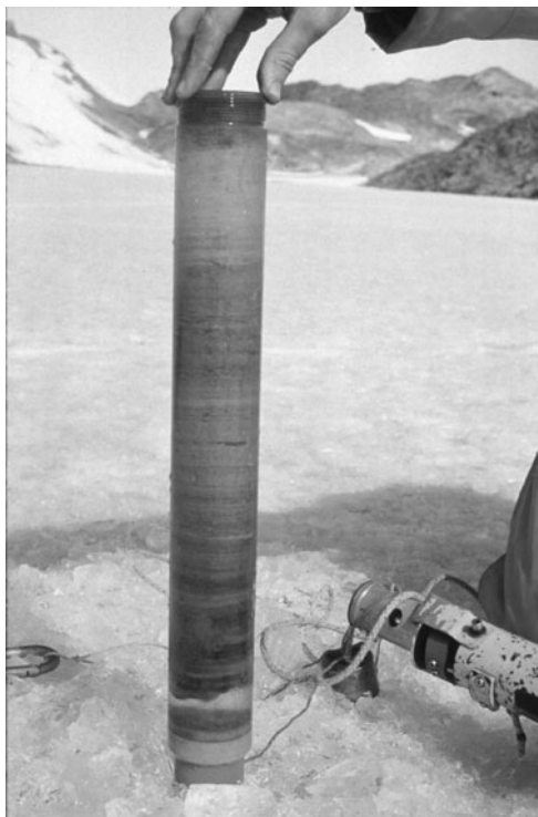
Figure 3.1 This 1600-year-old lake sediment core from the Larsemann Hills, East Antarctica, has intact layers of sediments that have accumulated year on year preserving a remarkably detailed record of environmental change. This core includes the remains of filamentous cyanobacterial mats and green algae that are strongly pigmented. These pigments help scientists to reconstruct which phototrophs were present and the growing conditions at the time of deposition. Photograph: D. Hodgson. See Plate 14 for the colour version.
