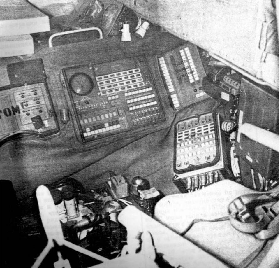
The flight engineer's side of the main control panel.
