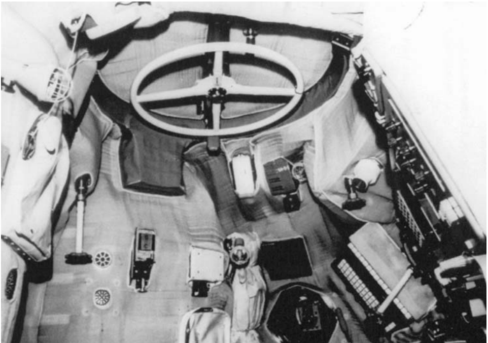
At the top of the Soyuz cabin is the hatch, with one of the ventilation valves visible under its ring on the right, next to a black box. (From the book Soyuz – A Universal Spacecraft , courtesy Rex Hall)
