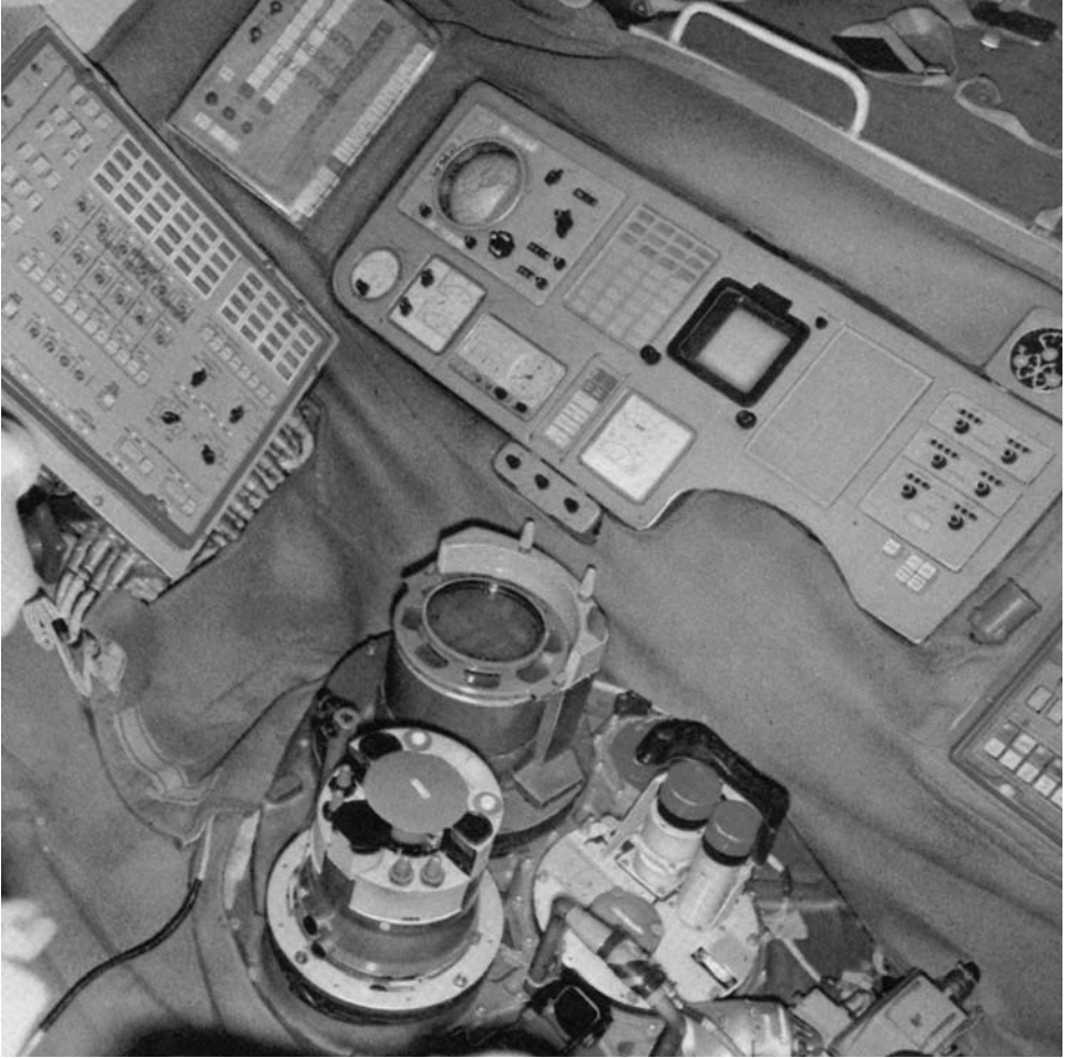
This section of the main control panel on the commander's side shows a globe for navigation and (bottom row, left to right) voltage, current, pressure and temperature, as well as the time, range and approach speed.
