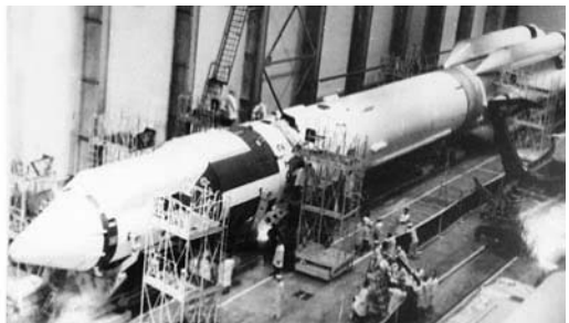
Left: Almaz-1 with a large solar panel on each side of the passive docking cone at the rear. On the right, Almaz-1 is mated with its Proton launch vehicle. Notice the sign Salyut 2 on upper stage's support ring.
