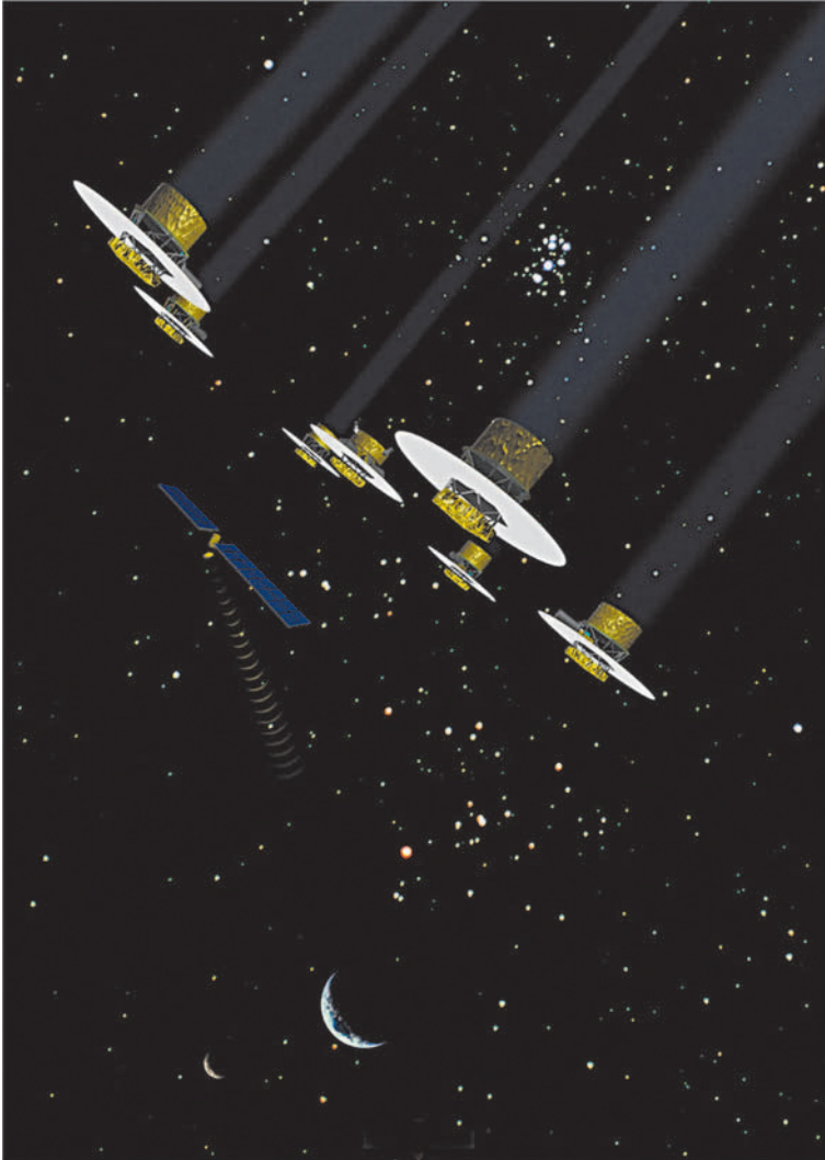
Figure 8.10. An artist's impression of the Darwin mission, consisting of a flotilla of six telescopes – each with an aperture of more than 1 metre – in an orbit beyond 5 AU from the Sun. Working as an interferometer, they will be able to image exoplanets in the vicinity of nearby stars.
