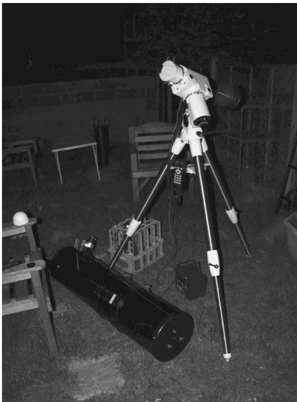
Figure 10.11. A photo of the aftermath of an actual incident in which a telescope (with camera) fell out of a dovetail fixing.
