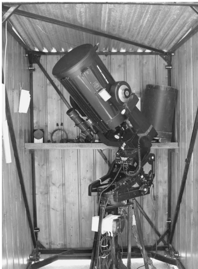
Figure 9.13. The inside of the SCT run-off shed.
