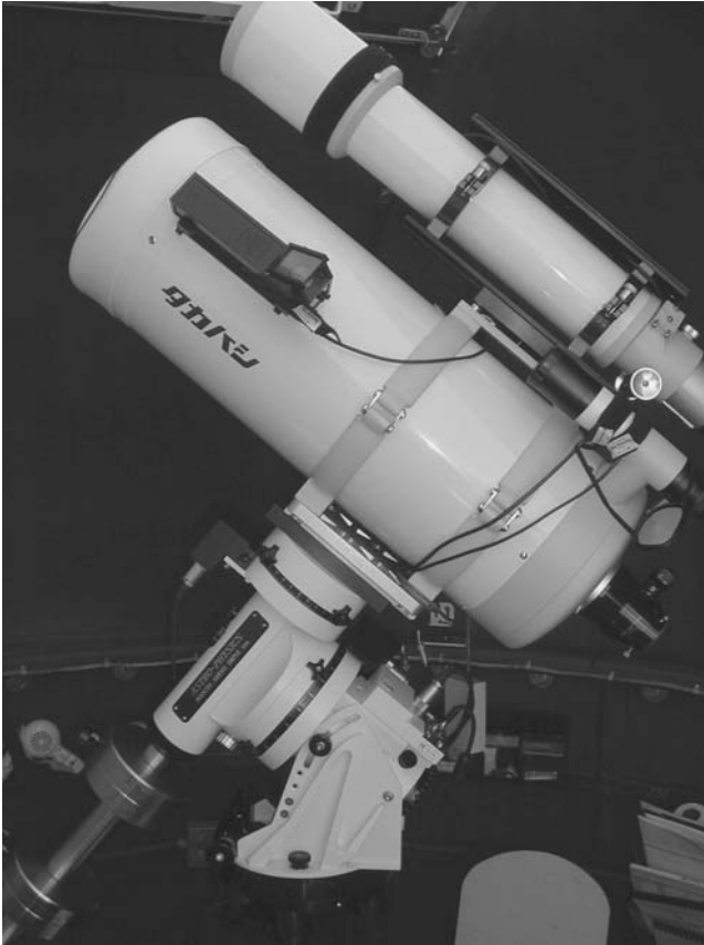
Figure 9.45. The Takahashi Mewlon reflector and Takahashi refractor on an Astro-Physics mount.
