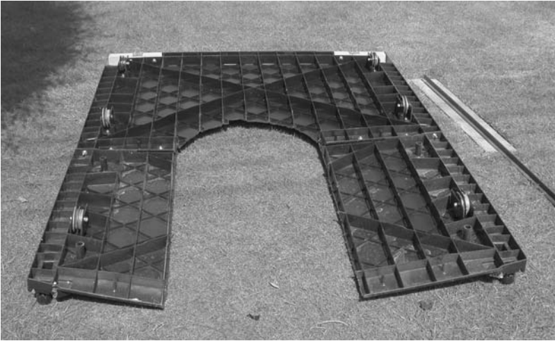
Figure 9.8. Adaptation of the plastic shed floor, also showing one of the slabs and rails on the lawn.
