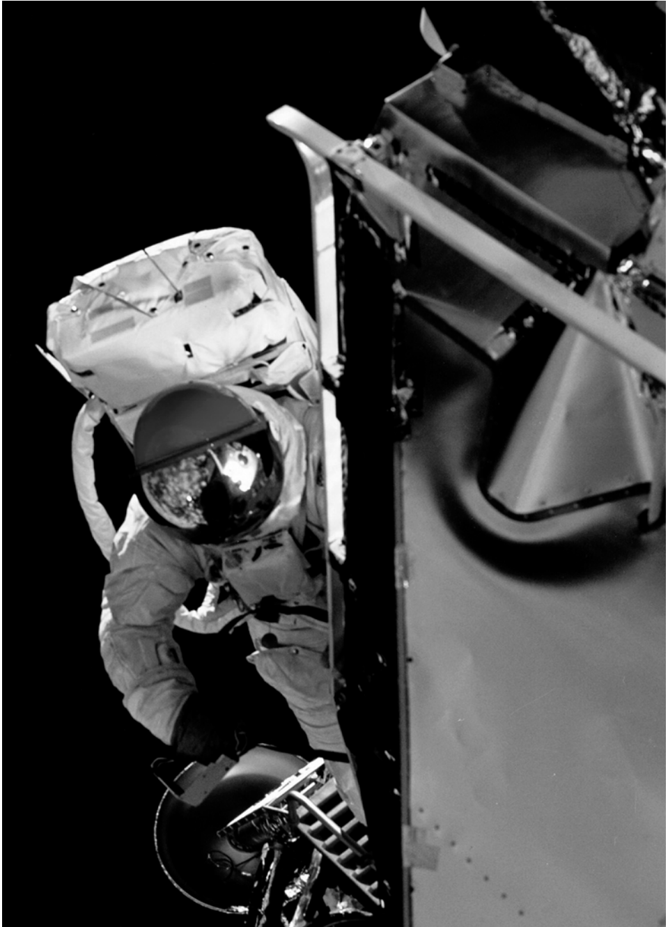
Rusty Schweickart tests the PLSS after exiting the forward hatch of LM-3 during Apollo 9.
