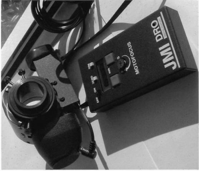
Figure 8.13. The superb JMI NGF-S Motofocus unit, which allows accurate focusing, with a digital position read-out. Photo by the author.
