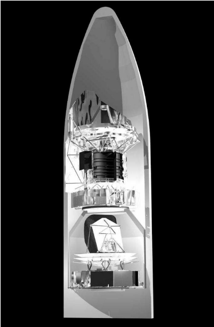
Figure 11.5. The Planck and Herschel spacecraft, depicted in their joint launch configuration atop an Ariane 5 booster. Herschel sits on top with Planck acting as a carrier during launch. Both are destined for the L2 region. (European Space Agency.)
