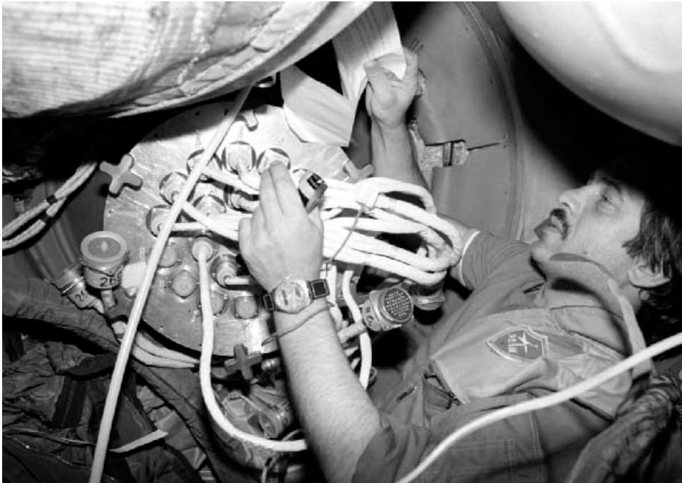
Vinogradov adjusts the hermaplate hatch leading to Spektr
