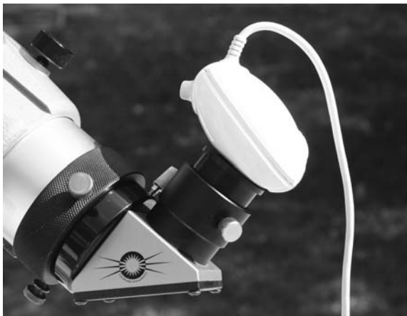
Figure 8.6. Phillips Toucam Pro Webcam mounted for imaging. Steve Rismiller.
