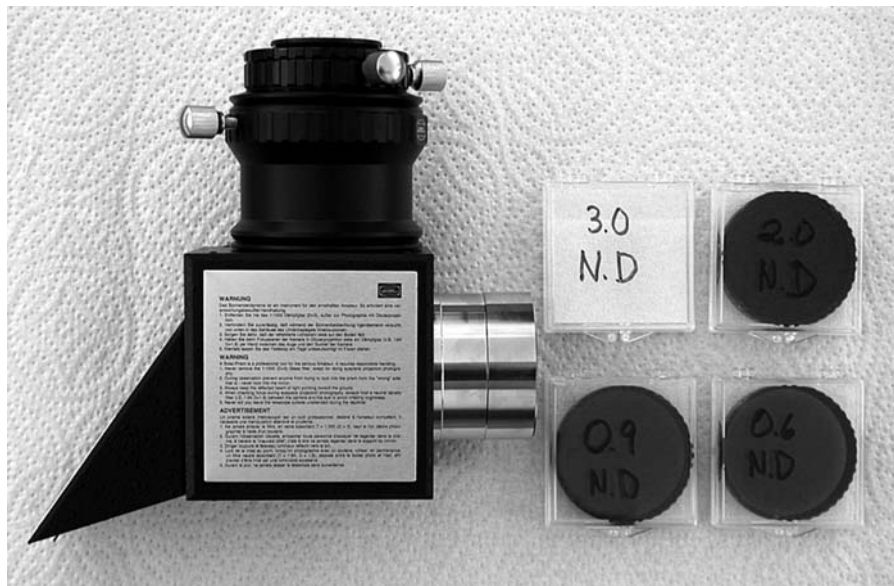
Figure 3.6. Herschel wedge by Baader Planetarium. The supplementary neutral density filters are supplied to control excess brightness of the view through the prism assembly. Eric Roel.
