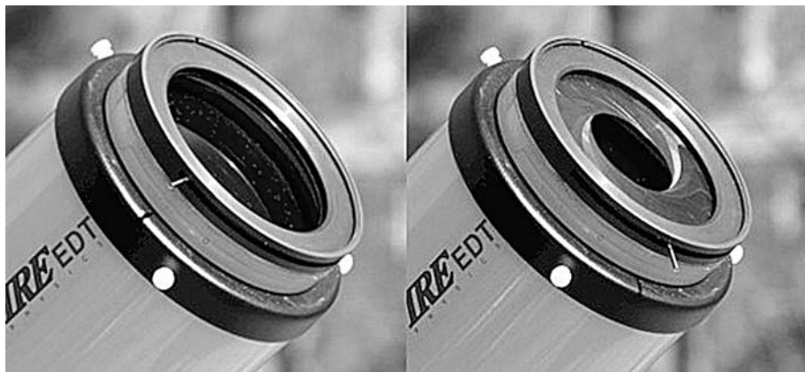
Figure 6.9. Adjustable iris diaphragm. Greg Piepol.
