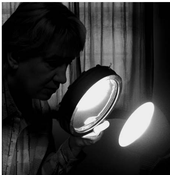
Figure 3.5. Check for defects such as pinholes, scratches, or a nonuniform coating on a solar filter before attaching it to a telescope.
