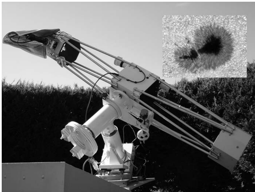
Figure 3.8. Art Whipple's 203 mm photographic Newtonian. The inset is an image of AR0908 obtained on September 10, 2006, under seeing conditions of 1 arc second. Art Whipple.
