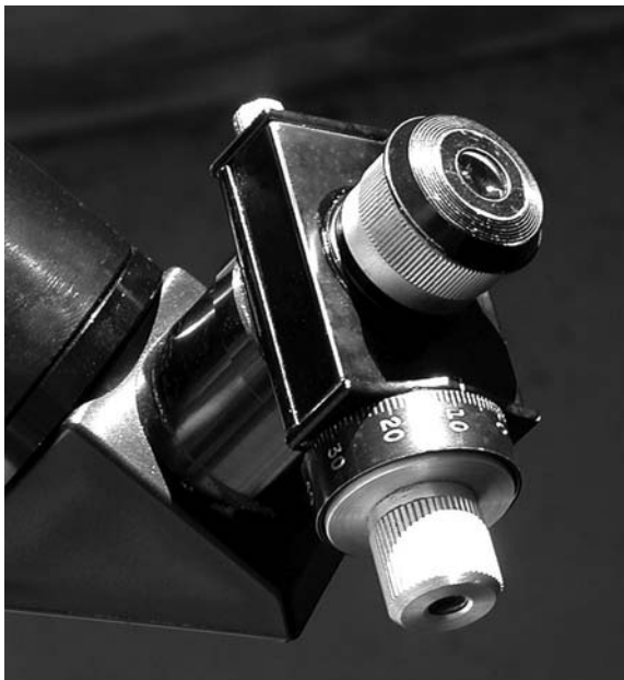
Figure 7.10. Filar micrometer used for prominence measurements. Jamey Jenkins.
