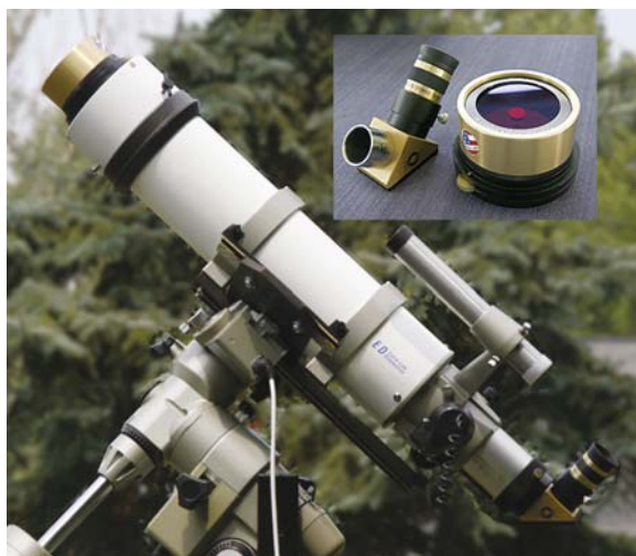
Figure 6.8. Coronado front loading 60 mm H alpha filter set mounted on a Vixen 102ED telescope. Steve Rismiller.
