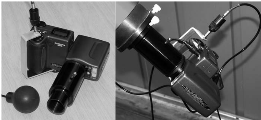
Figure 8.3. Nikon Coolpix 990 digital camera setup for afocal photography.
