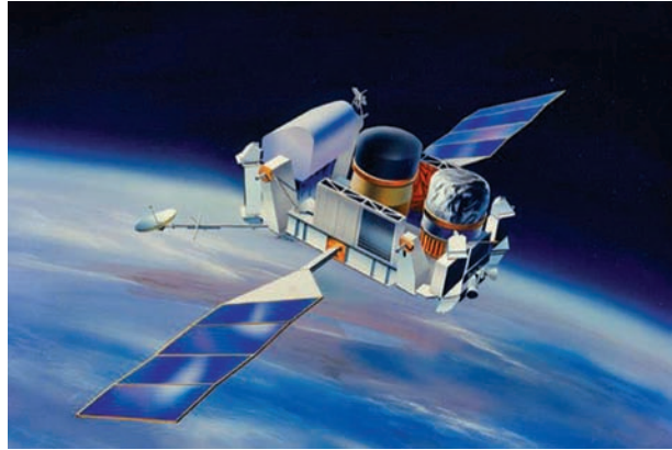
CGRO, launched in 1991. The two cylinders are the scintillation detectors. Credit: NASA.
