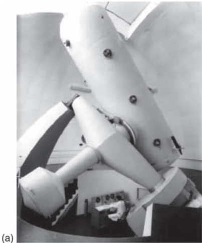
(a) A telescope with an equatorial mount (Haute Provence Observatory). Note the counterweight balancing the weight of the tube. (b) An example of an alt–az mount (ESO VLT).
