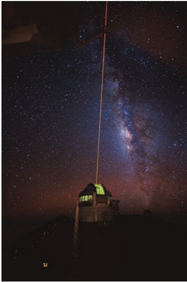
Laser beam creating an artificial star in the atmosphere. Credit: Gemini Obs.
