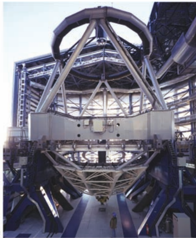
(a) A telescope with an equatorial mount (Haute Provence Observatory). Note the counterweight balancing the weight of the tube. (b) An example of an alt–az mount (ESO VLT).
