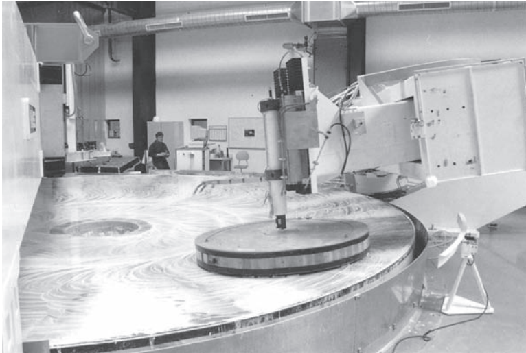
Polishing an 8 m mirror using a small computer-controlled tool. The optician in the background gives an idea of the scale. Credit: REOSC.
