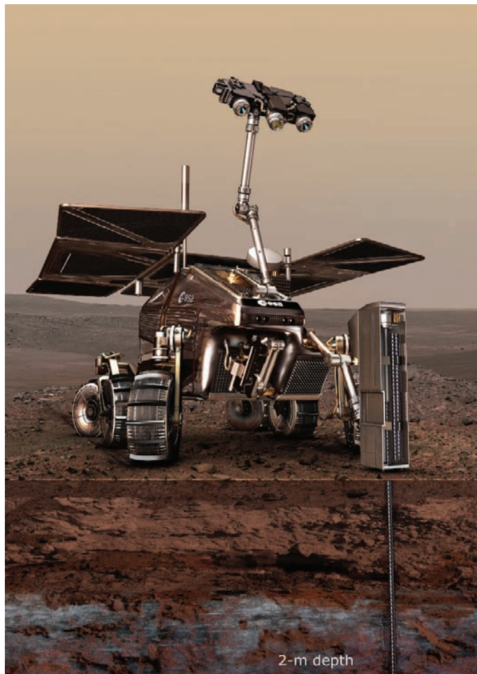
Fig. 9.10 Artist's impression of the ExoMars Rover drilling into the Martian surface. The vehicle will be able to travel a few kilometres with its 16.5 kg exobiology payload. Surface and subsurface samples of Mars will be subjected to chemical analysis in a miniaturized laboratory onboard the Rover. Here, chiral organic molecules can be separated into their enantiomers, identified, and quantified with the help of (a) enantioselective gas chromatography by MOMA and (b) enantioselective capillary electrophoresis by UREY to search for signs of past or present life. Credits of ESA – AOES Medialab
