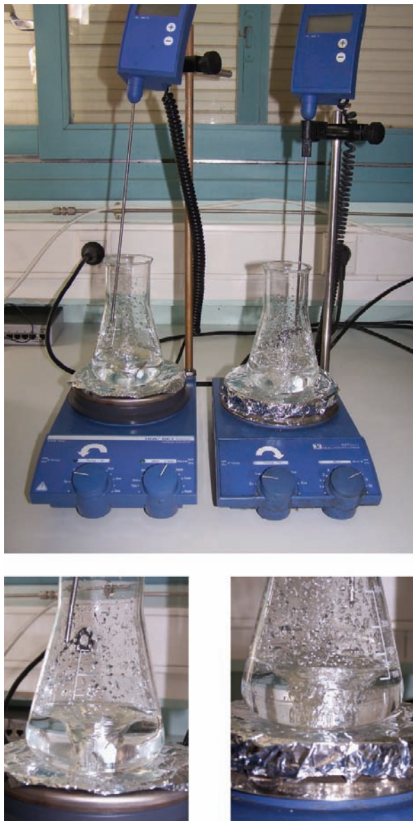
Fig. 4.6 Stirred not shaken: Experimental set up for clockwise ( right ) and counterclockwise ( left ) stirring of appropriate chemical systems. The obtained vortices are magnified
