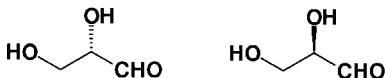
Fig. 2.7 Chemical structures of (-)-L-glyceraldehyde ( left ) and (+)-D-glyceraldehyde ( right ) used for labelling D- and L-enantiomers
