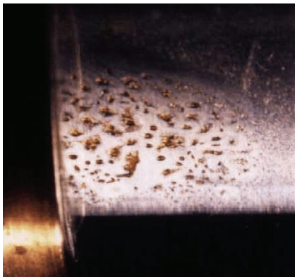
Fig. 7.3 Producing a comet in the lab: yellowish residue obtained after simulating interstellar and circumstellar ices on the surface of the cold finger (here: an aluminium block of 30·40 mm surface). After extraction, hydrolysis, and chemical derivatization, a wide variety of different chiral amino acid structures was identified therein
