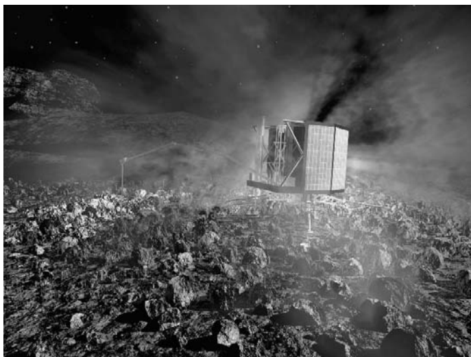
Fig. 9.3 This artist's impression shows the ROSETTA Lander Philae anchored to the comet's surface. Philae will work for a minimum mission target of 65 hours, but its operations may continue for many months. The Lander's structure consists of a baseplate, an instrument platform, and a polygonal sandwich construction, all made of carbon fibre. Some of the instruments and subsystems are beneath a hood, which is covered with solar cells. An antenna transmits data from the surface to Earth via the orbiter. The lander carries nine experiments, with a total mass of 21 kilograms. It also carries a drilling system to take samples of subsurface material. Credits: ESA/AOES Medialab
