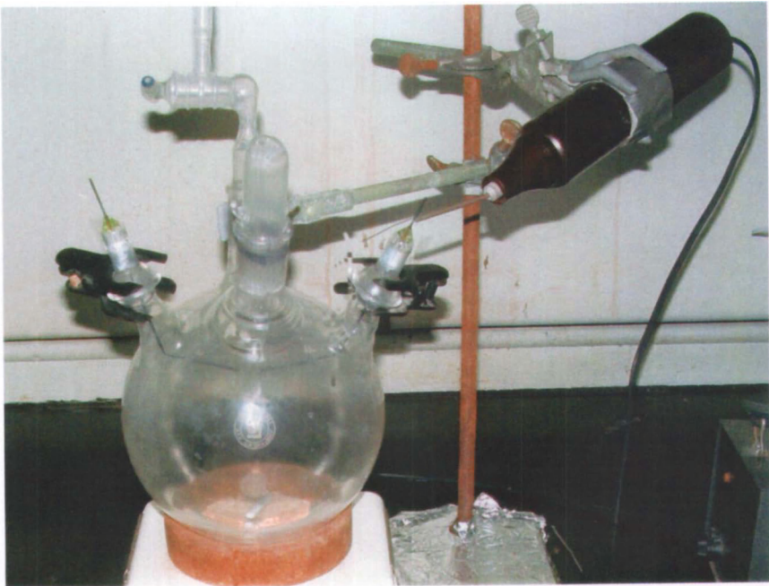
Plate 15.1. Spark discharge apparatus used in these experiments.
