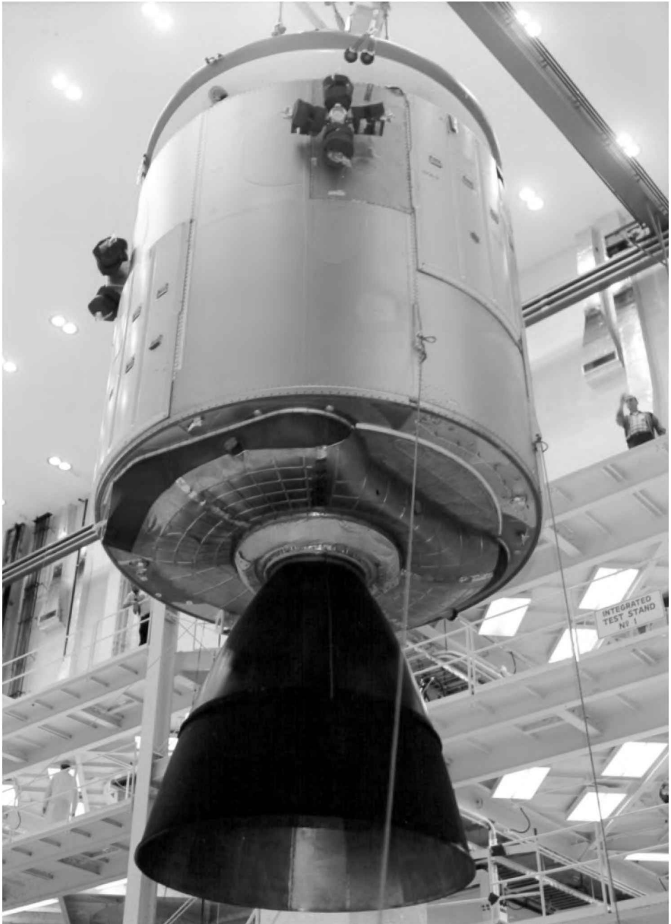
The Apollo 1 command and service module during testing, with the Service Propulsion System (SPS) engine and thruster quads clearly visible. Apollo 1 would have been the first and only flight of the 'Block 1' design – a design disliked and distrusted by both Gus Grissom and Wally Schirra.
