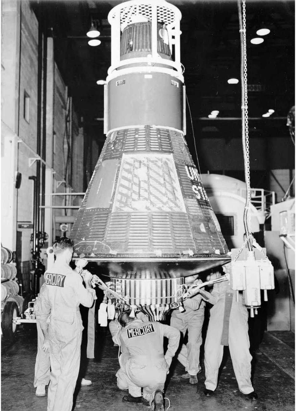
The Mercury spacecraft. Note the parachute container at the top and the retrorocket package at the base of the capsule.
