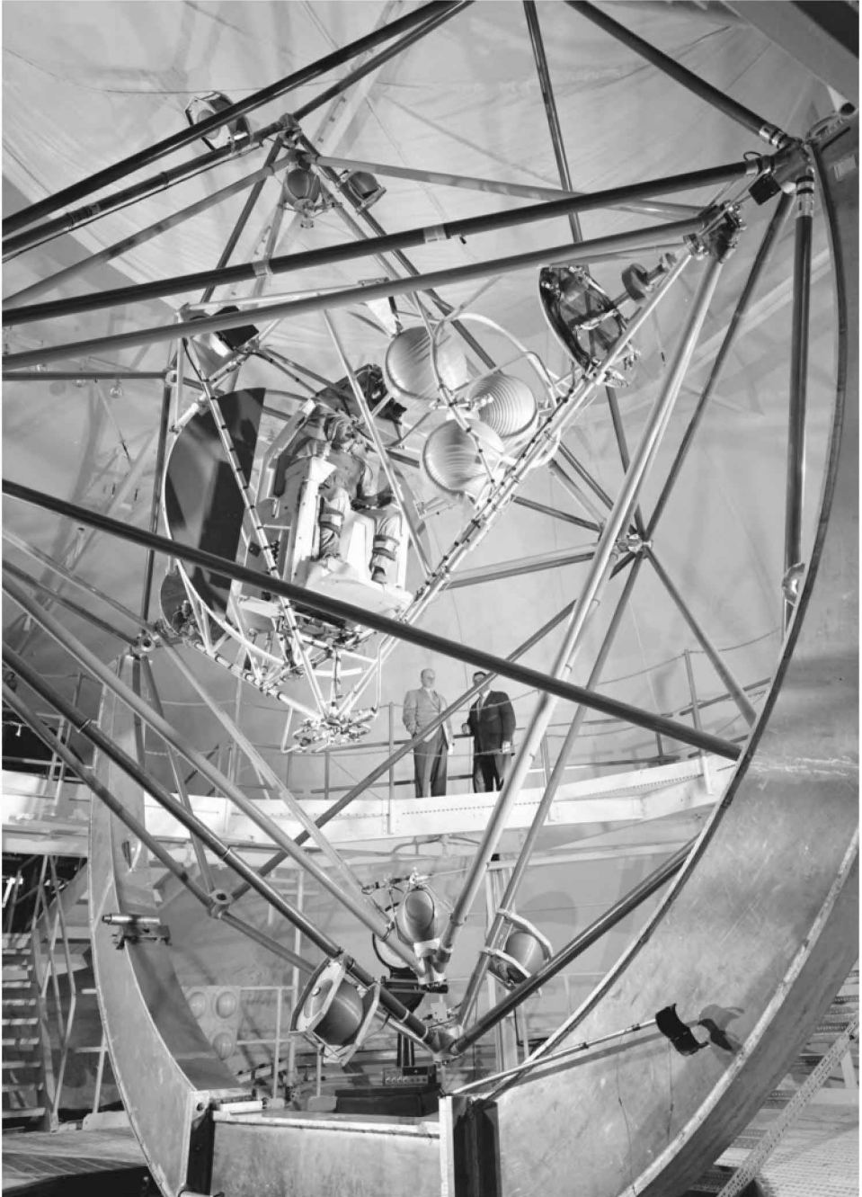
Described as one of the most sadistic trainers ever created, the Multiple-Axis Space Test Inertia Facility (MASTIF) comprised three interlocking cages to simulate motions about roll, pitch and yaw axes.
