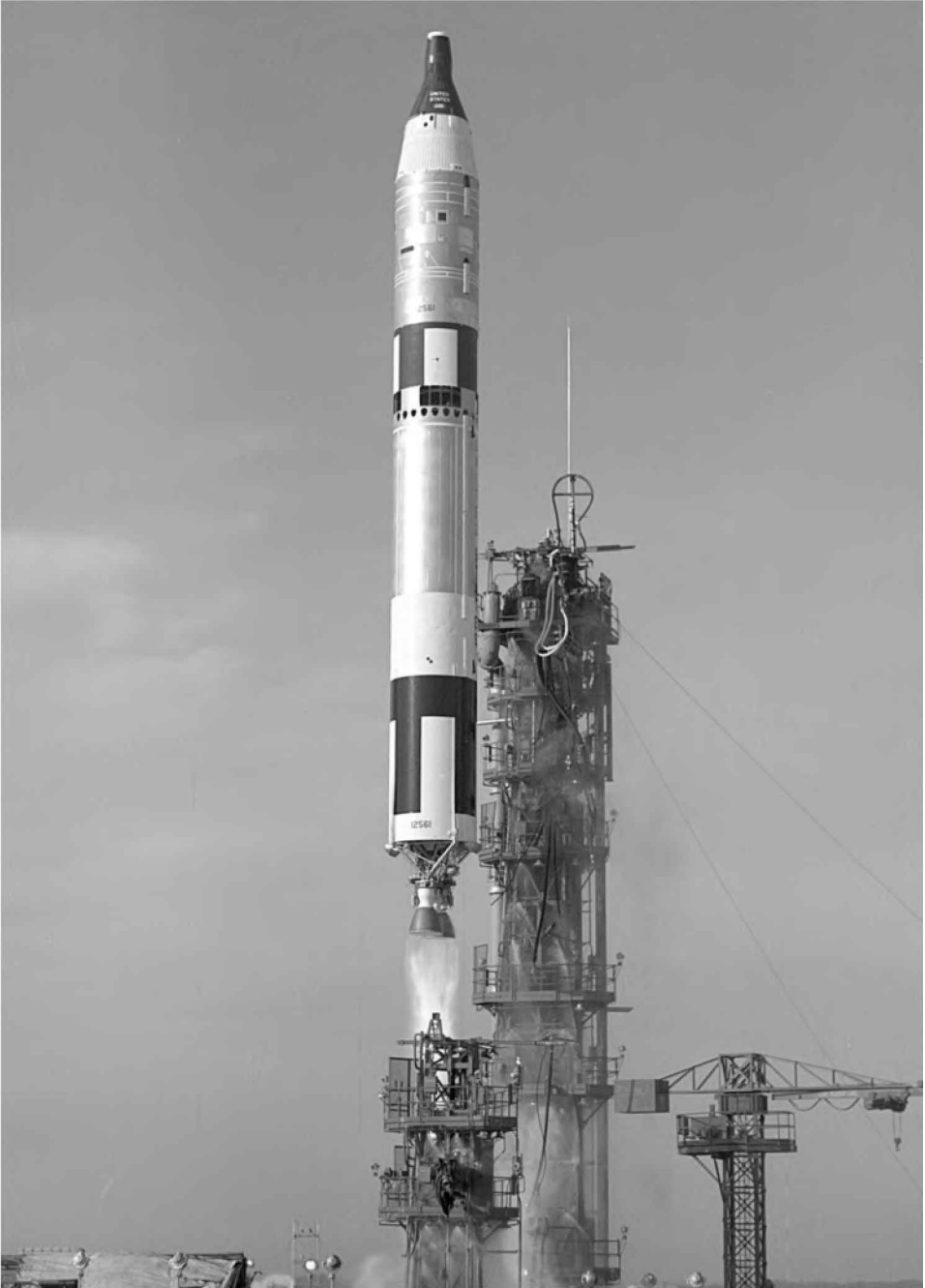
A Gemini-Titan launch. Note the absence of an escape tower; Gemini crews, aboard their conspicuous black-and-white spacecraft, relied instead upon an ejection system. Privately, many astronauts doubted its usefulness.
