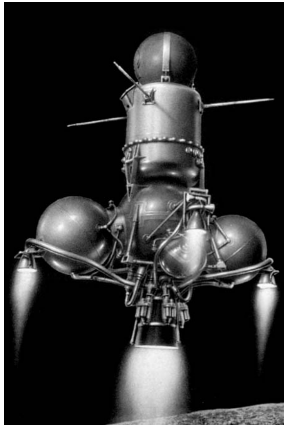
A depiction of the Luna 16 ascent stage lifting off with its lunar sample in the spherical capsule on top. (Courtesy Lavochkin Association)
