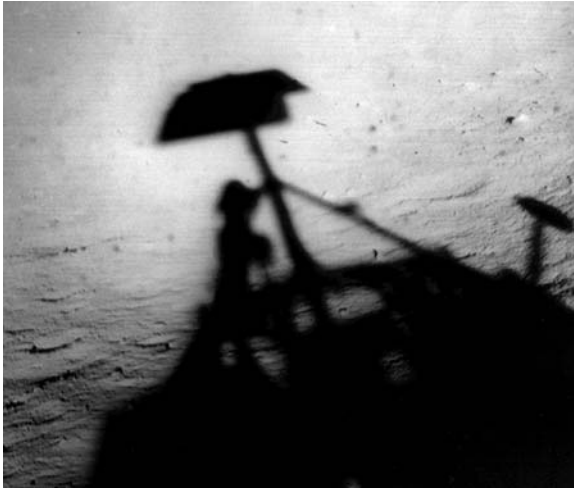
Surveyor 1 photographed its own shadow, revealing there to be an intense 'zero-phase' glare of backscattered sunlight.
