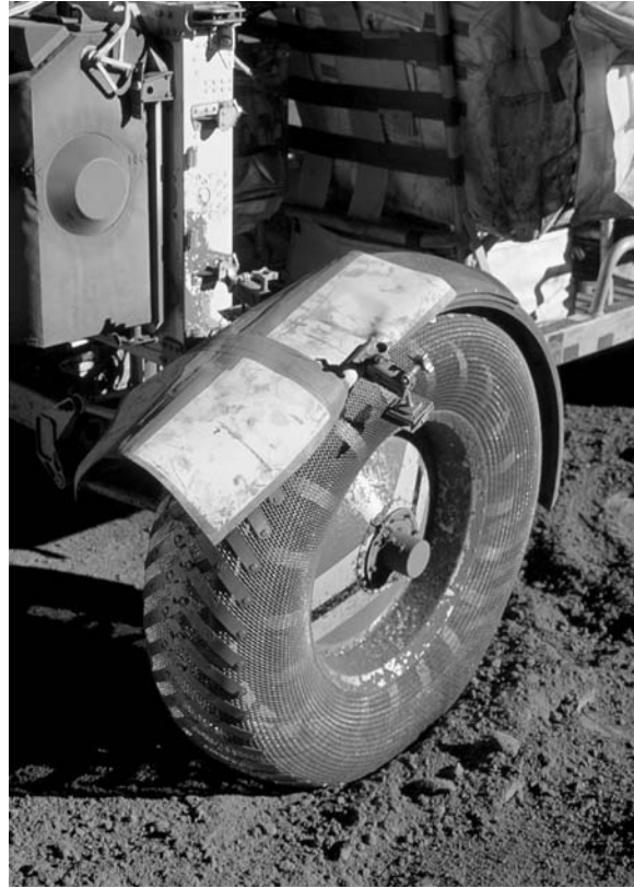
The ad hoc substitute for the Rover's damaged fender.
