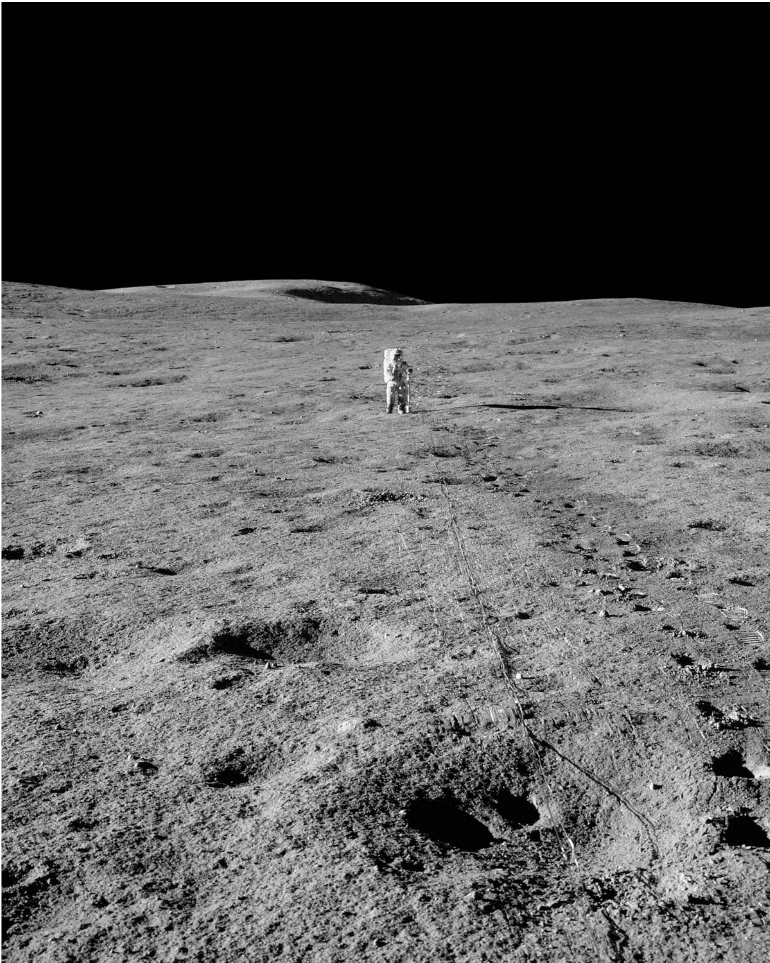
For the Active Seismic Experiment, Ed Mitchell laid out a line of geophones and then walked along the line with a 'thumper', firing explosive charges in order to probe the structure of the Fra Mauro Formation.
