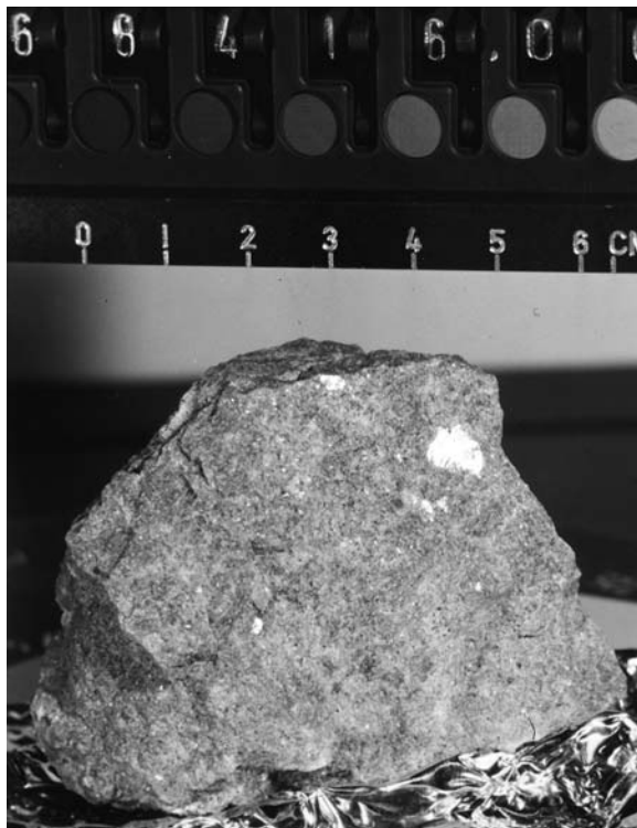
Sample 68416, a 0.18-kg fragment of the 'white boulder' at Station 8 that was dated to 3.76 billion years.
