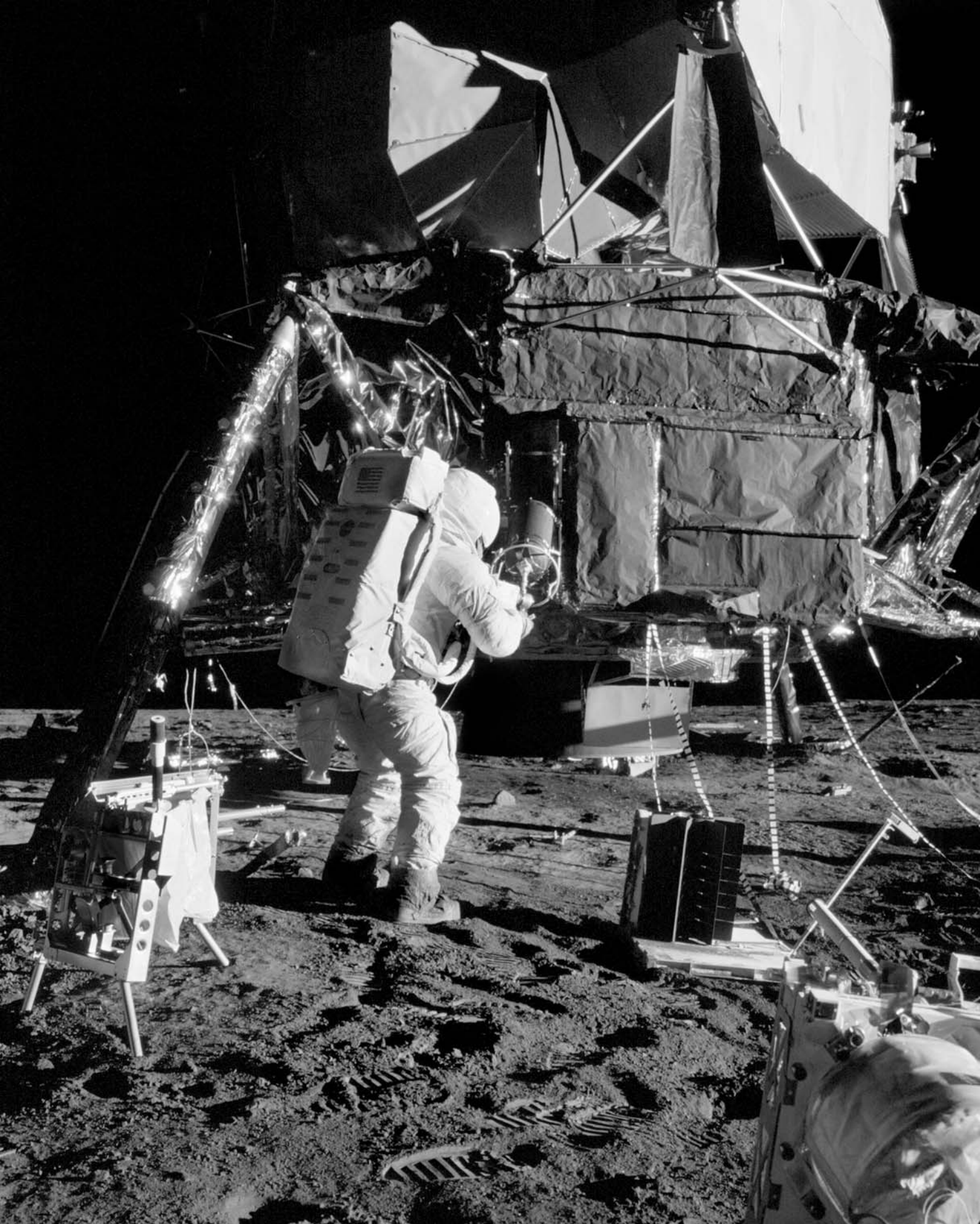
Al Bean retrieves the plutonium core of the Radioisotope Thermal Generator with which to power the instruments of the Apollo Lunar Surface Experiment Package.
