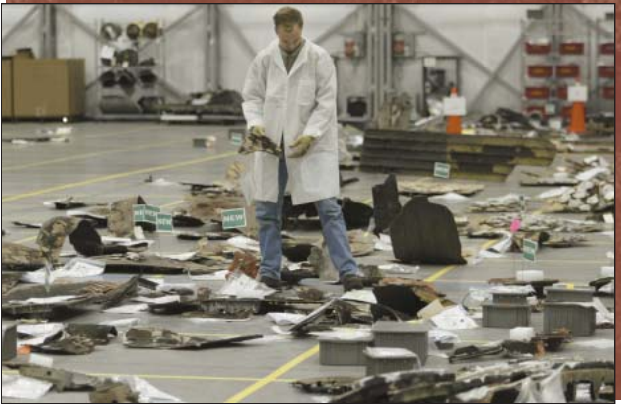
Debris from Columbia is laid out on a grid at the Reusable Launch Vehicle Hangar at Kennedy Space Center to determine the cause of the accident.
