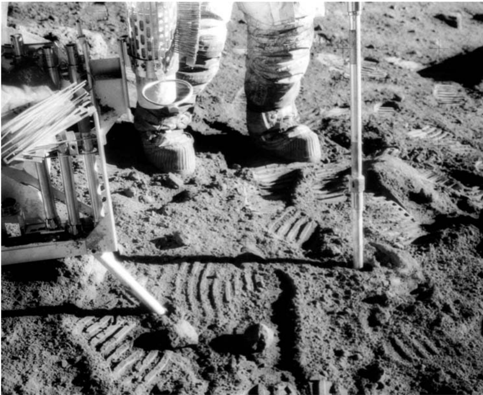
Figure 2.7. Dirt. Dirt everywhere. High-velocity meteorite impacts – over billions of years and at all scales – as well as some explosive volcanism have combined to cover the moon with thick deposits of lunar regolith. When you kick it, the soil scatters far and wide in the moon’s vacuum and reduced gravity. In this water-free vacuum environment, particles stick to everything. Dirt patterns on Al Bean’s knees indicate that he has been kneeling at some point in the EVA. With the sampling scoop punched into the surface and the tool carrier at hand, Bean appears to be ready to collect a soil sample.
