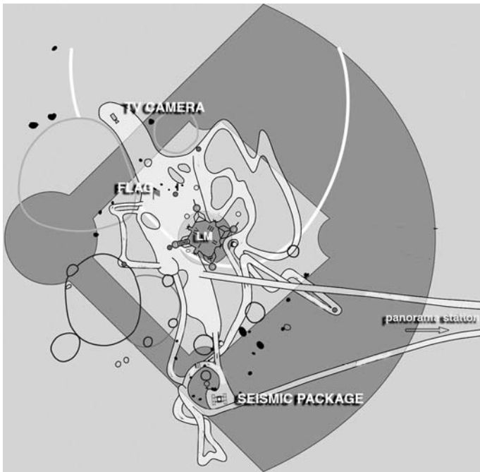
Site Map. This schematic Apollo 11 traverse map was adapted from the Apollo 11 Preliminary Science Report by Thomas Schwagmeier. For scale, the site has been superimposed on a baseball diamond, with the LM on the pitcher's mound. The light gray paths are routes taken by the crew as they moved about during the EVAs. The path at lower right was the route taken by Armstrong to take a photographic panorama of the site. Ovals are edges of subdued craters, and dark blotches represent large rocks.
