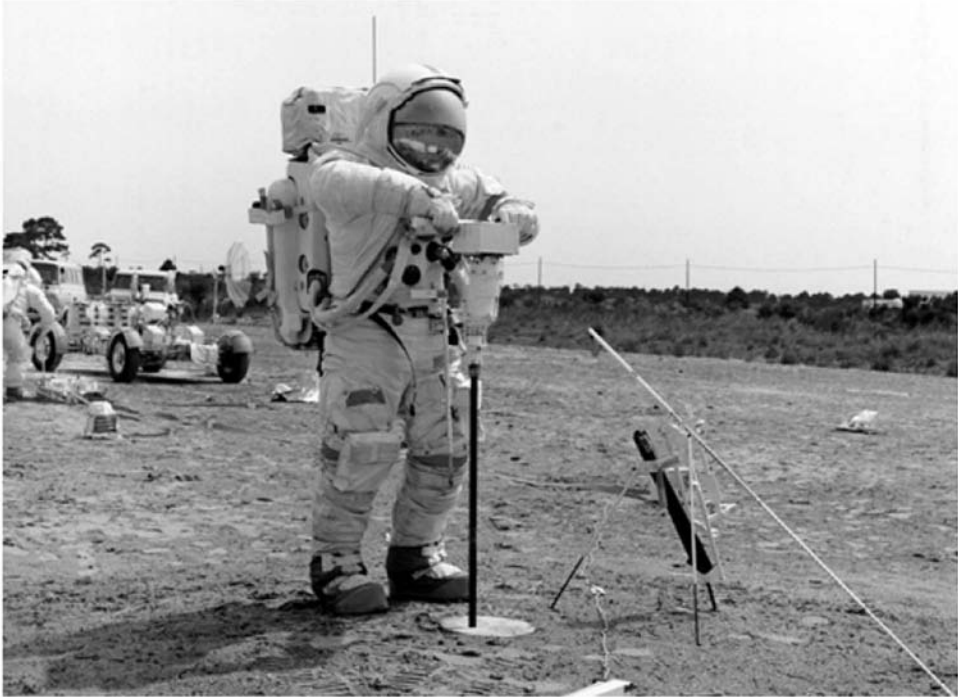
Figure 5.2. Training with the electric drill at the Kennedy Space Center, Dave Scott drills into a buried canister of simulated lunar soil. The drill stem rack to the right of the drill contains a cluster of four core stems. The wrench attached to the back of the rack becomes important in EVA-3. Despite all the tests and dry runs, there was nothing to compare with the arduous task of drilling into actual lunar regolith at 1/6 g.
