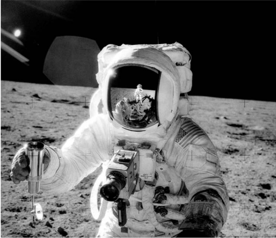
Figure 2.8. This photo, taken at Sharp Crater, shows the team of Conrad and Bean at its best. Working together, they are filling the “long can,” a vacuum-sealed sample container designed to protect the soil sample from the Earth’s environment when they return to Houston. The nearly full can is sealed with the lid, which is hanging by a cord from the bottom. This photo gives us a good view of the top of Al’s Hasselblad camera as well as the cuff checklist and watch on his left sleeve. The visor reflection shows Pete, the HTC carrier, and the remarkable contrast between the lunar surface and the darkness of space.
