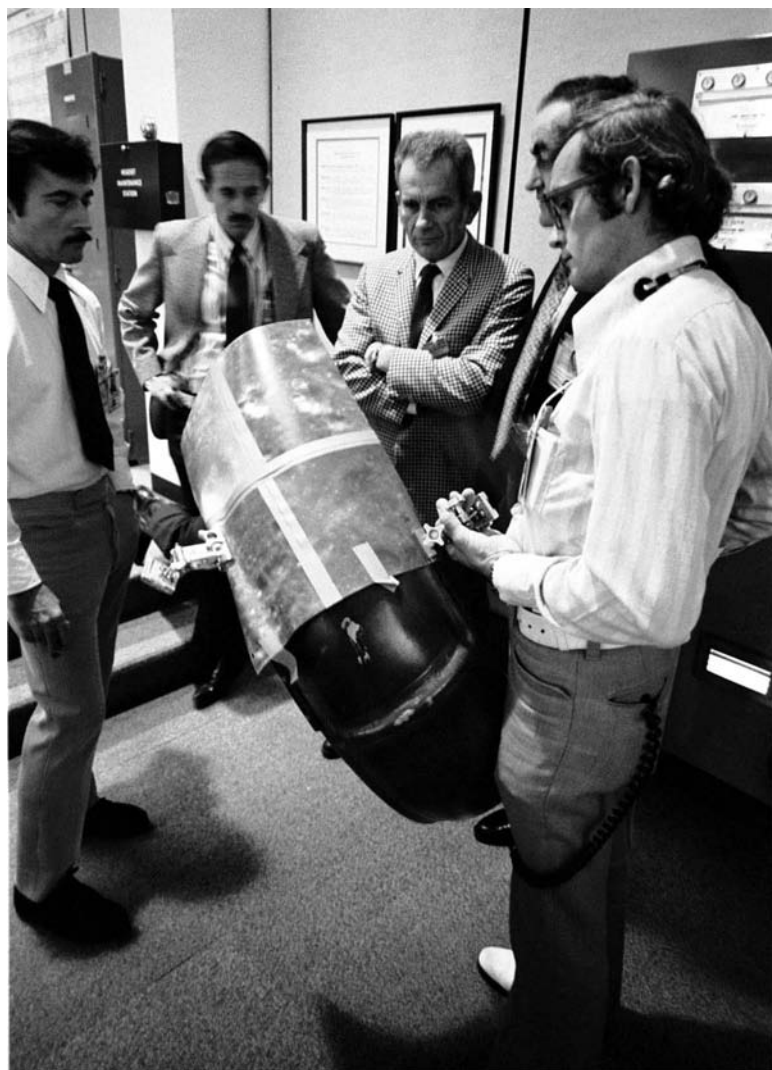
Figure 9.4. “Never go exploring without a roll of duct tape.” In the Backroom during Apollo 17, (left to right) John Young, Charlie Duke, Deke Slayton, Rocco Petrone, and Ron Blevins discuss a replacement fender devised for the Rover. Gene Cernan had accidentally caught the handle of his geology hammer under the fender and torn off the rear extension. This jury-rigged replacement would use spare maps and duct tape the crew had on-board. After Young did a trial installation in a pressure suit to test the method, Houston passed on the instructions to Cernan and Schmitt for making their own replacement fender. During the EVA-1 closeout, CapCom Bob Parker told the crew, “We’ll take a look at it here while you’re sleeping.” Incidents of this sort illustrate the importance of the support teams as well as ingenuity in using materials at hand. The Apollo crews didn’t have the time or tools to do any but the simplest of repairs. Such capabilities will be important on the longer duration missions of the future.
