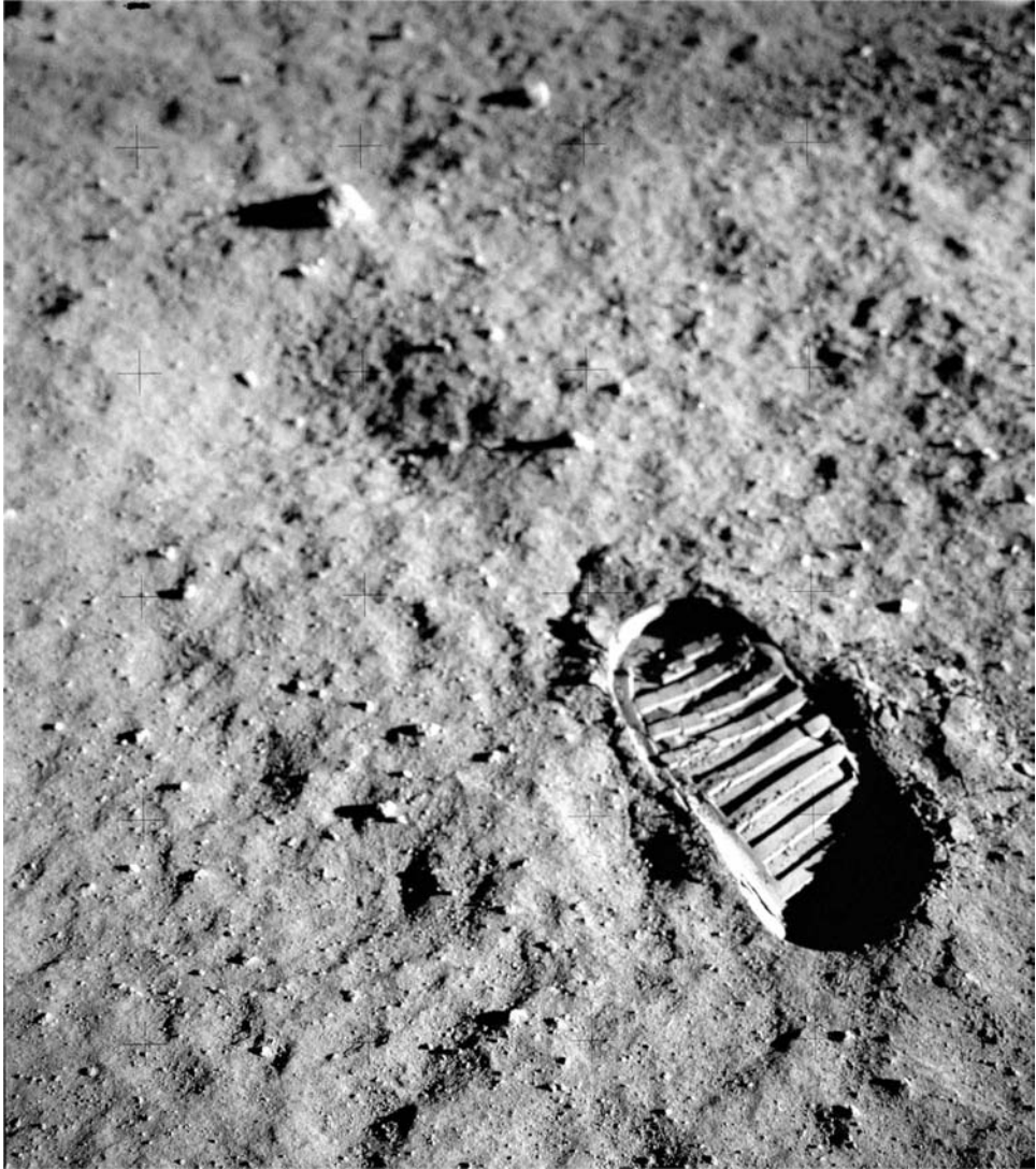
Figure 1.2. Contrary to commonly held belief, this photo is not a picture of the first footprint on the Moon. Buzz Aldrin took this photograph much later in the EVA to show a boot print he'd just made as part of the soil mechanics team's investigation of the lunar surface's physical properties. This boot print – and all the others – laid to rest a wildly dramatic theory that the lunar surface was fluffy and that the astronauts would meet their end by sinking into some sort of dusty quicksand. At the immediate surface, the soil was fluffy enough that Buzz's boot sank in a fraction of a centimeter or so, but at greater depths it was compact enough to easily support his weight. Most important was the fact that man had left his mark on a surface that, in any one spot, might not have been disturbed in millions – or perhaps even billions – of years. The astronauts were aware that in this truly pristine environment, an incautious step could ruin a remarkable sampling opportunity.
