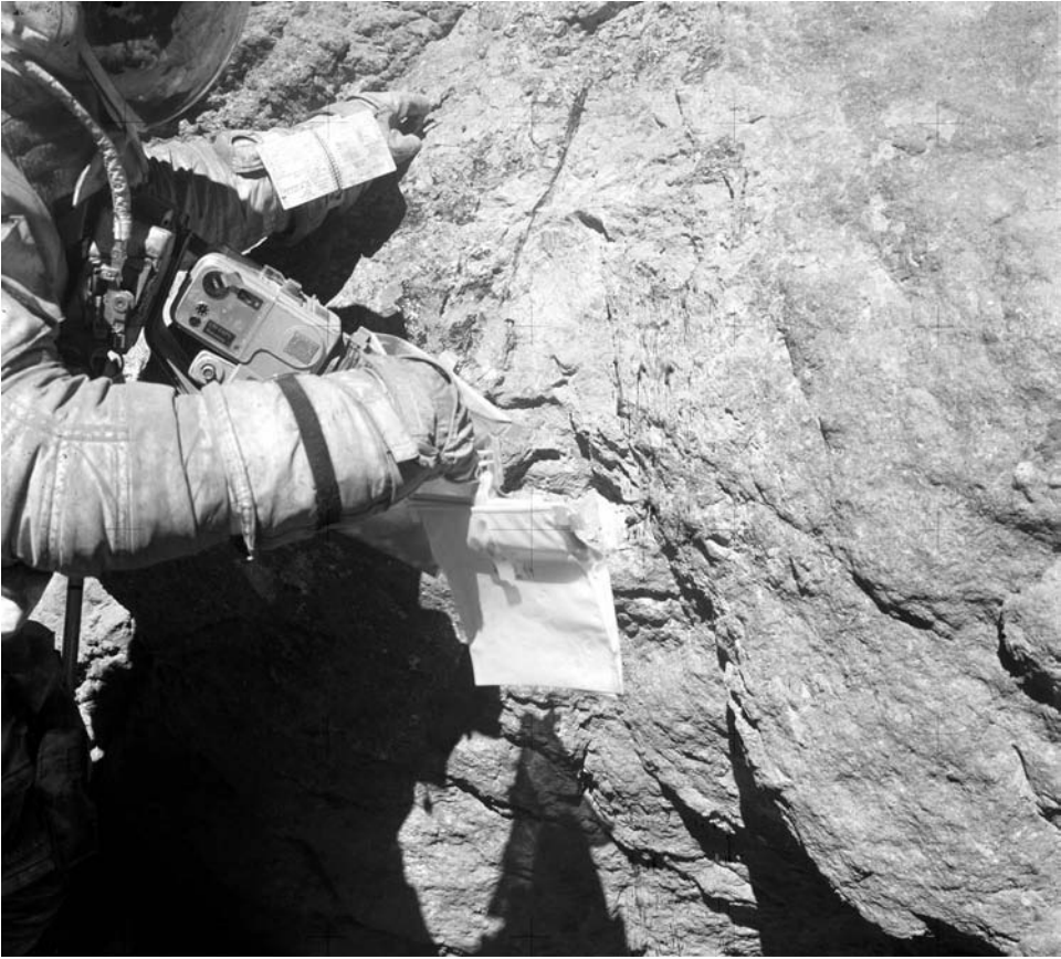
Figure 6.5. Charlie is pointing to a sample location on the face of Outhouse Rock – part of House Rock that probably broke off when the huge boulder landed. He has a pack of sample bags hooked to his finger because the bracket on the bottom of his camera that was designed to hold the bags has broken. The shadow cast by the sample bags is orange, which is normal when sunlight is transmitted through the translucent Teflon film from which the bags are made. In high-resolution versions of this picture, we can see that Charlie has magazine K (Kilo) on his Hasselblad and that his checklist is open to pages EVA-3 LMP-30 and EVA-3 LMP-31 (such high-resolution photography is accessible on the ALSJ site).
