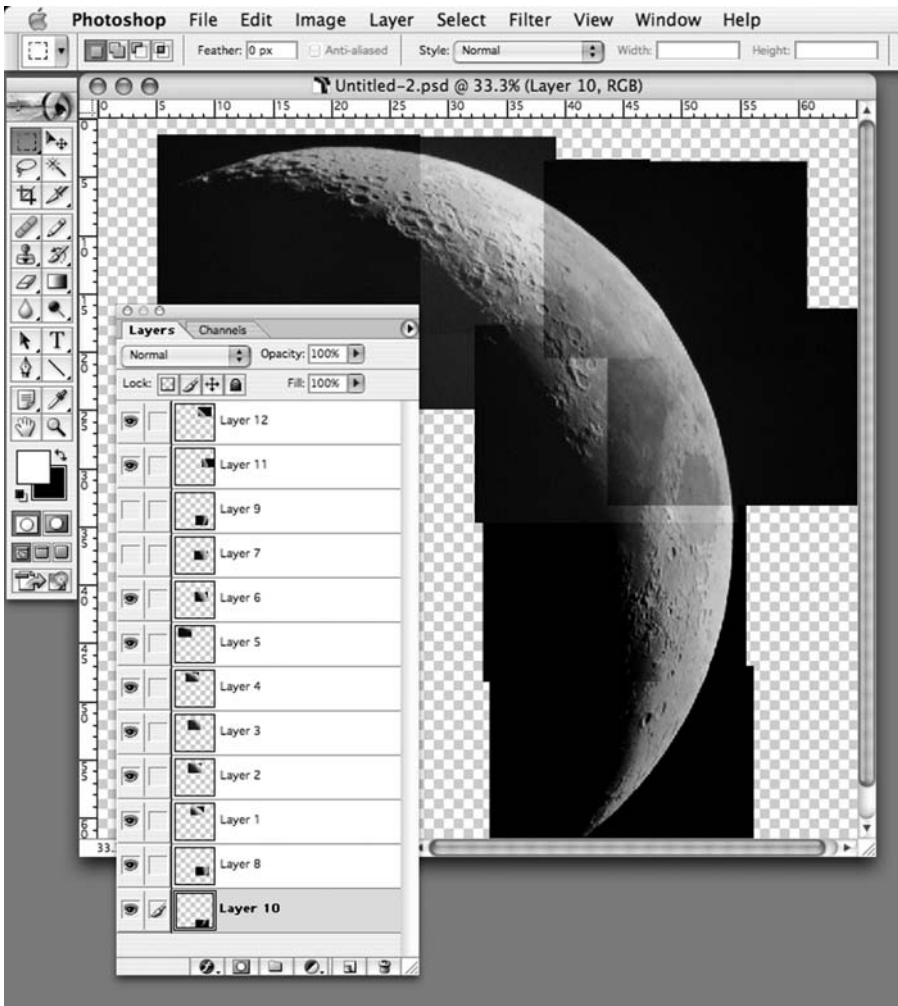
Figure 6.14. Each frame is pasted into the mosaic as a new layer, and that way it is easy to adjust the color and contrast of each frame so that it matches its neighbors perfectly.
