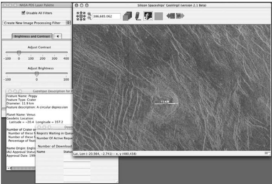
Figure 3.19. GeoVirgil is a Java-based program that will run on any modern computer with a fast Internet connection. It downloads and displays images of the surfaces of the planets together with key information about the thing being viewed and performs a variety of additional functions such as allow the user to measure the dimension of structures and export the picture as a JPEG.
