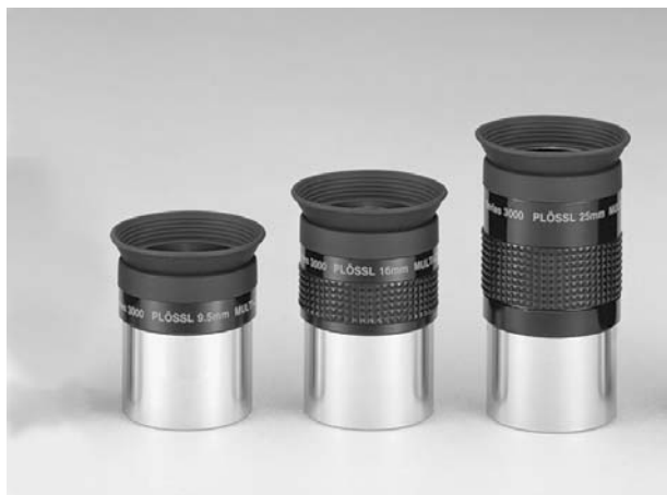
Figure 5.9. Plössls are the most popular moderately priced eyepieces, and on telescopes slower than f/5 they generally work very well. Their main problem is limited eye relief at focal lengths less than 10 to 12 mm (photo courtesy of Meade Instruments Corporation).
