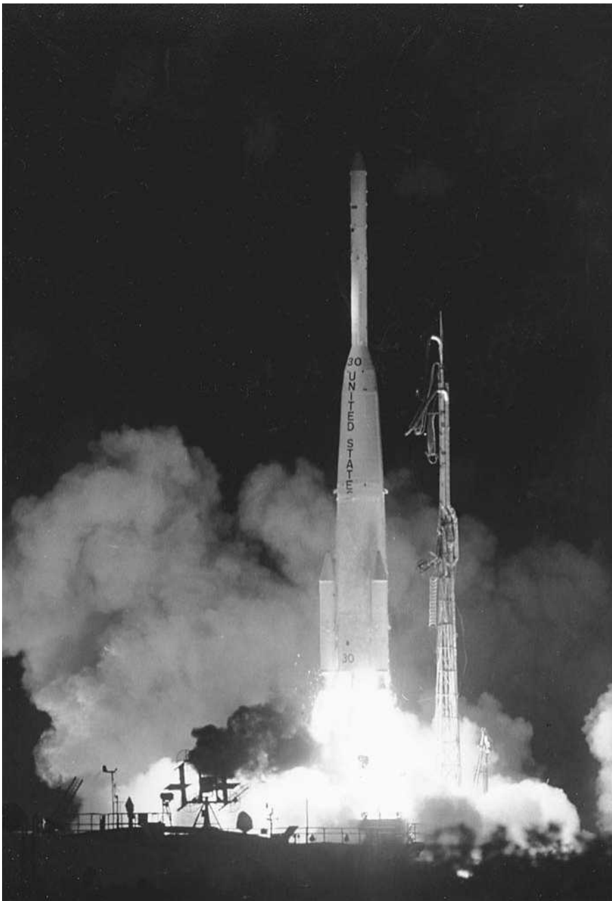
A Delta rocket lifts off at Cape Kennedy carrying the world's first commercial communications satellite, Early Bird. The satellite, launched in 1965, was intended to operate as a switchboard relaying radio, television, teletype, and telephone messages between North America and Europe.
