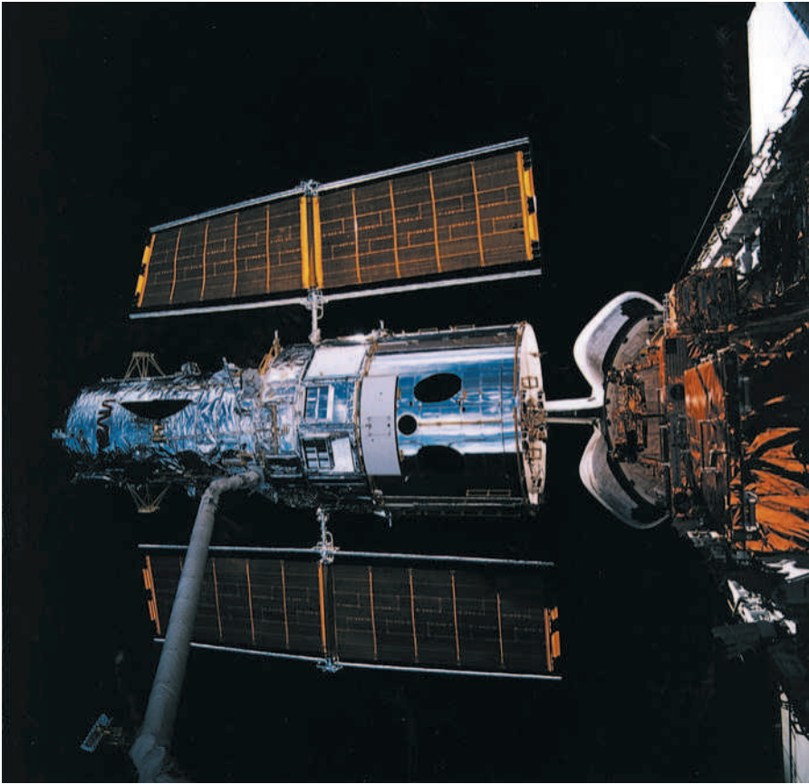
The Hubble Space Telescope (HST) is lifted into position by the Remote Manipulator System (RMS) from its berth in the cargo bay of the Earth-orbiting space shuttle Discovery.
