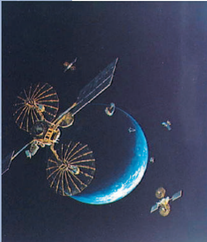
The Tracking and Data Relay satellite system is a sophisticated network that has granted NASA increased communication abilities between Earth and its low-orbit spacecraft.
