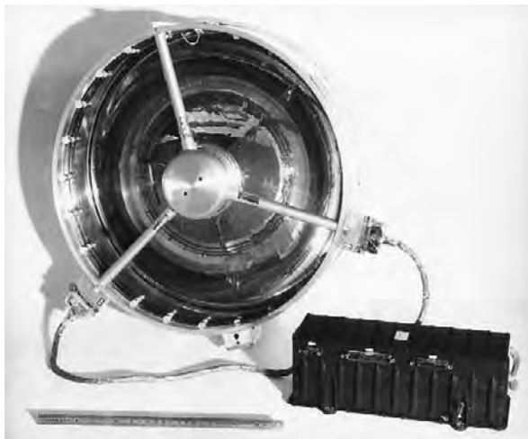
FIGURE 12 The Galileo micrometeoroid detector (sensor and electronics box); the detector onboard the Ulysses spacecraft is of the same kind. The cylindrical sensor has a diameter of 43 cm. The bottom of the sensor contains the hemispherical impact target; in the center are charge-collecting electrodes. The detector records impacts of submicron- and micron-sized dust particles above 1 km/s impact speed.
