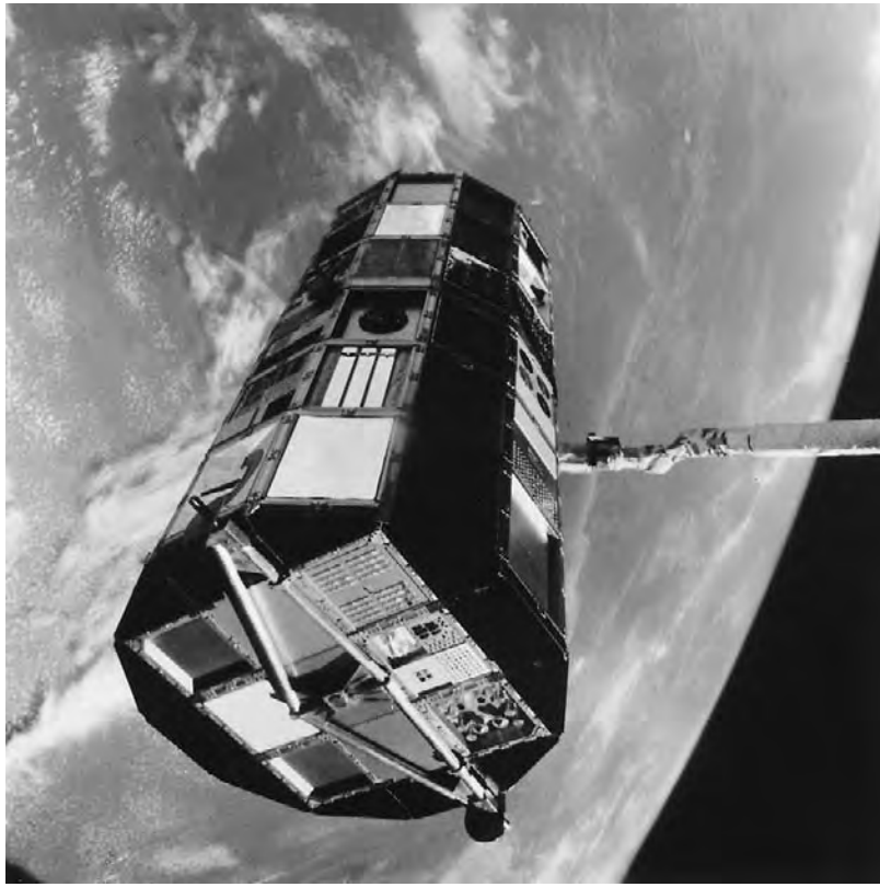
FIGURE 11 Release of the Long Duration Exposure Facility (LDEF) from the space shuttle in 1984. Various trays containing collectors and materials have been exposed to the space environment for 6 years. (Courtesy of NASA.)
