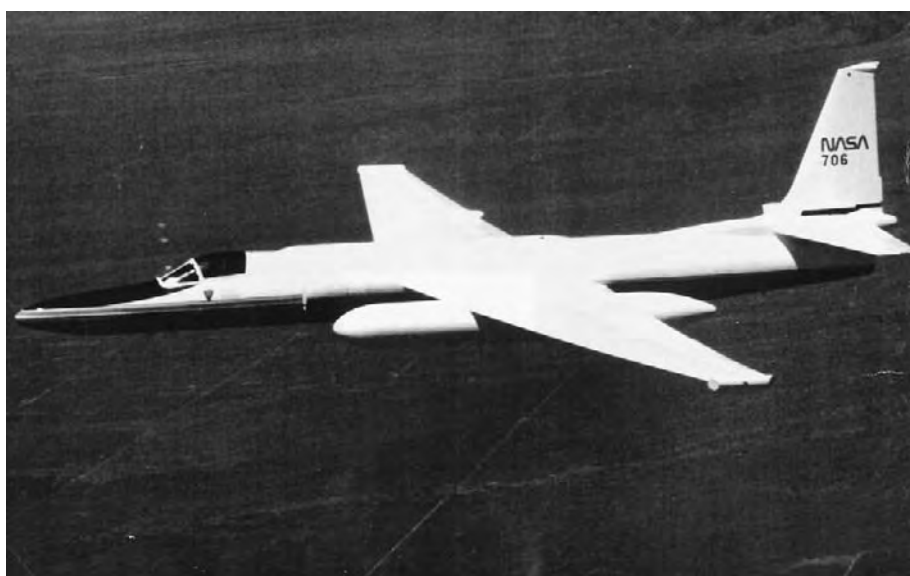
FIGURE 5 The high-flying NASA ER-2 airplane is used to collect interplanetary dust particles sedimenting through the atmosphere. The dust collector is mounted below the wings. (Courtesy of NASA.)
