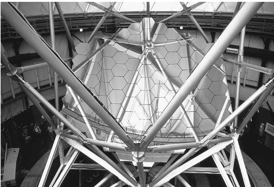
Fig. 3.19. The mirror of a telescope can be made up of several smaller segments, which are much easier to manufacture, as in the Hobby–Eberle Telescope on Mount Fowlkes, Texas. The effective diameter of the mirror is 9.1 m. A similar telescope is being built in South Africa. (Photo MacDonald Observatory)
