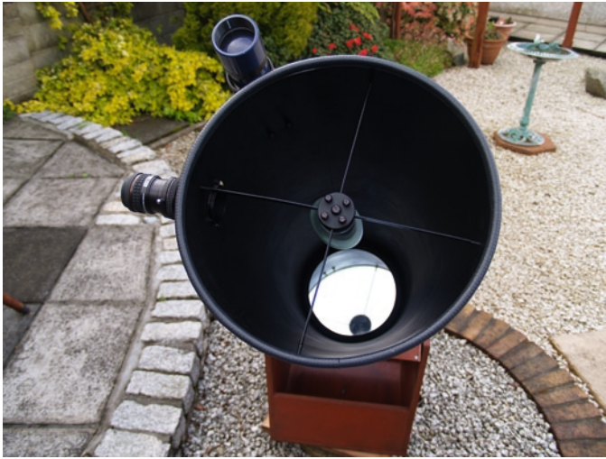
Peter Grego constructed the primary mirror and mount for his 12-inch Newtonian reflector. (Credit: Peter Grego.)
