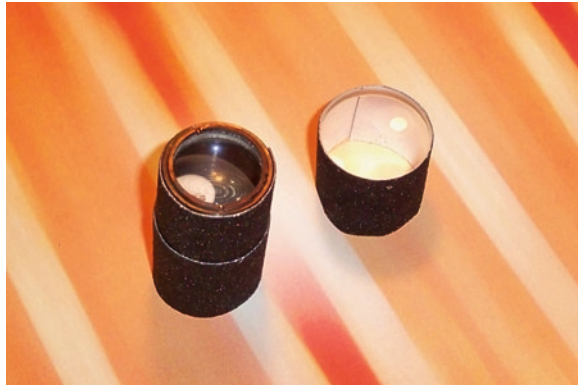
Grip tape houses the objective and eye lenses (Credit: Peter Grego)
