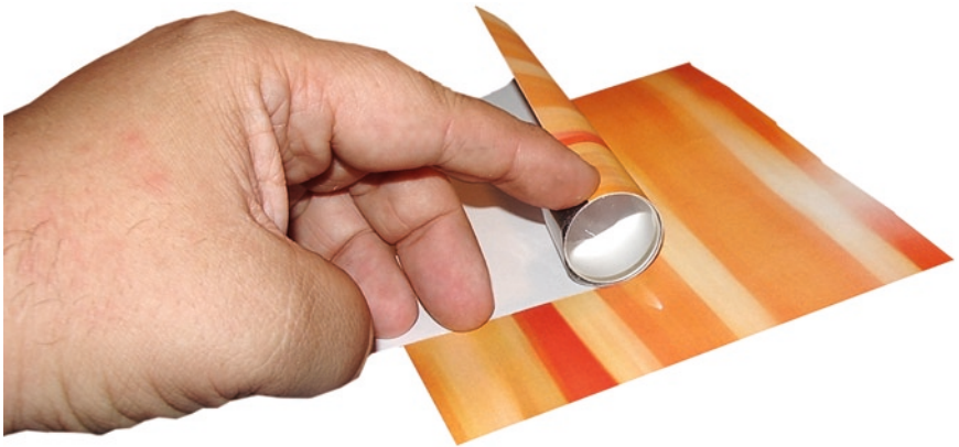
The lenses are rolled in thin card to create the main tube and drawtube (Credit: Peter Grego)
