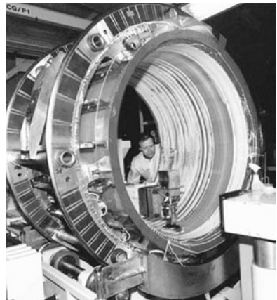
Fig. 3.4. Construction of the Chandra mirrors. Here we see one of the approximately cylindrical shells during the polishing stage. The shell shown is one of eight that make up the complete X-ray mirror for Chandra. Compare with the previous figure. (Figure used by permission of the Optical and Space Systems Division, Goodrich Corporation; the division was formerly part of Raytheon Corporation.)
