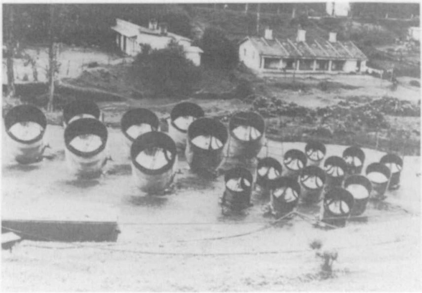
Figure 5.6. The 20 parabolic mirror array to detect Cerenkov light produced by showers. The array was operated by the Tata Institute of Fundamental Research group at Ootacamund (Ooty), until 1985, and now at Pachmarhi, India. Two small mirrors were not used in the experiment. (Photograph by A.R. Apte.)
