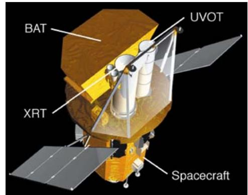
**Figure 4.8.** Schematic view of the Swift satellite (Gehrels et al. 2004). The size of the coded mask of BAT is  $2.7\text{ m}^2$ .
