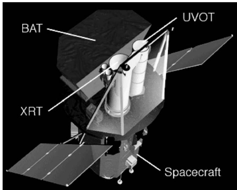
**Figure 4.8.** Schematic view of the Swift satellite (Gehrels et al. 2004). The size of the coded mask of BAT is  $2.7 \text{ m}^2$ . *See also* Color section.
