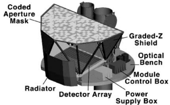
**Figure 4.9.** The main elements of the Swift platform (Gehrels et al. 2004). See also Color section.
