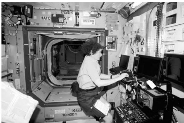
Figure 5. Expedition 2 crew member, Susan Helms, operates the Canadarm 2 from the Destiny module (NASA photo). This figure is available in full color at http://www.mrw.interscience.wiley.com/esst .
