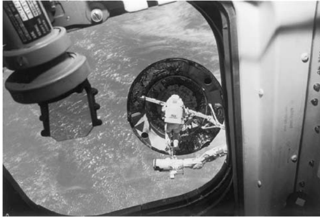
Figure 6. An astronaut is seen standing in a foot restraint on the RMS while attempting to latch a handling fixture onto the INTELSAT- VI communications satellite.
