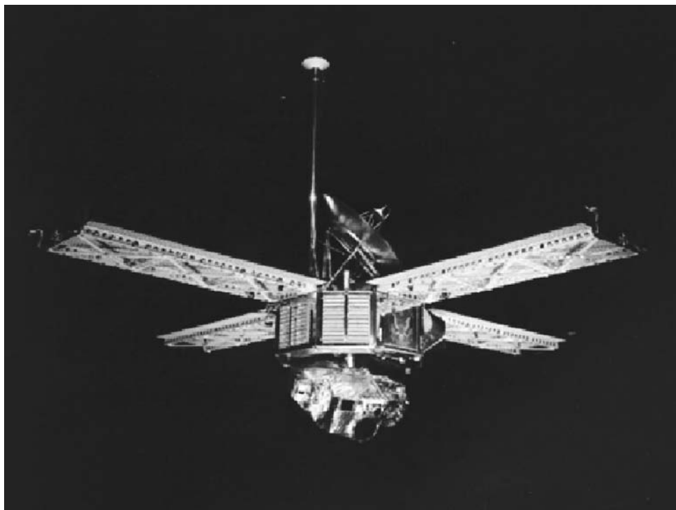
Figure 4. Mariner 6 and 7 were designed to fly over the equator and southern hemisphere of the planet Mars. They were solar powered and capable of continuous telemetry transmission. Each spacecraft weighed 910 pounds (413 kilograms) and measured 11 feet (3.35 meters) from the scan platform to the top of the low-gain antenna. The width across the solar panels was 19 feet (5.8 meters). The eight-sided body of the spacecraft carried seven electronic compartments. A small rocket engine, used for trajectory corrections, protruded through one of the sides. The planetary experiments aboard the spacecraft were two television cameras, an infrared radiometer, and infrared spectrometer and as ultraviolet spectrometer. (Courtesy NASA.) This figure is available in full color at http://www.mrw.interscience.wiley.com/esst .
