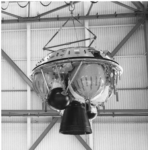
Figure 8. Ariane 5 second stage. This figure is available in full color at http://www.mrw.interscience.wiley.com/esst .
