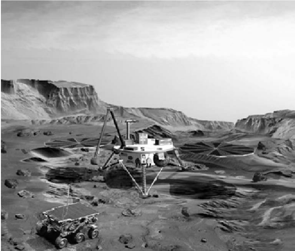
Figure 16. The Mars Surveyor Lander 2001 . This spacecraft was part of the canceled program already mentioned in the caption for Figure 15. It is likely to be used eventually in a future NASA Mars exploration flight. The Lander will carry an imager to take pictures of the surrounding terrain during its' rocket-assisted descent to the surface. The descent imaging camera will provide images of the landing site for geologic analyses, and will aid planning for initial operations and traverses by the rover. The Lander will also be a platform for instruments and technology experiments designed to provide key insights to decisions regarding successful and cost-effective human missions to Mars. Hardware on the Lander will be used for an in-situ demonstration test of rocket propellant production using gases in the Martian atmosphere. Other equipment will characterize the Martian soil proper and surface radiation environment. (Courtesy of NASA/JPL, 2001 Artwork by Corby J. Waste.) This figure is available in full color at http://www.mrw.interscience.wiley.com/esst .
