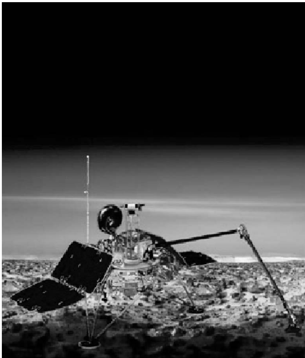
Figure 14. The Mars Polar Lander Spacecraft was launched from Cape Canaveral on January 3, 1999. The spacecraft was lost on December 3, 1999, during Mars orbit insertion. The payload included instruments for sampling soil at the surface and also within one meter of the surface. In addition, there was a stereoscopic camera and also meteorological sampling equipment. (Courtesy NASA/JPL.) This figure is available in full color at http://www.mrw.interscience.wiley.com/esst .
