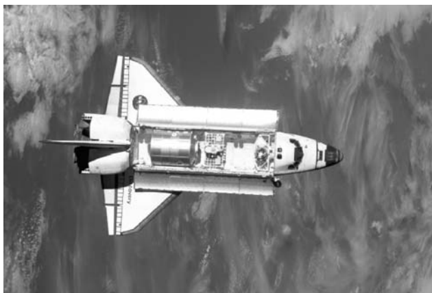
Figure 10. The MPLM in the Shuttle cargo bay approaches the ISS (NASA photo). This figure is available in full color at http://www.mrw.interscience.wiley.com/esst .
