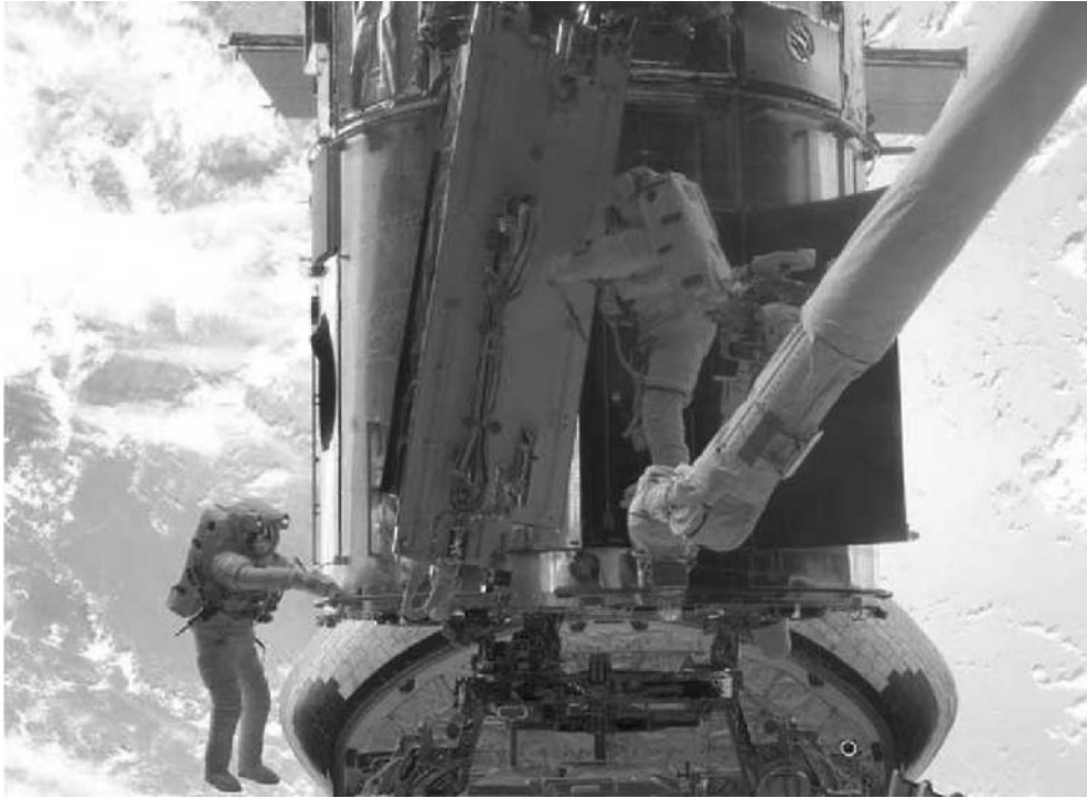
Figure 4. Astronauts John Grunsfeld and Richard Linnehan install a new exterior radiator, part of the NICMOS Cooling System, on the Hubble Space Telescope during Servicing Mission 3B in March 2002. This figure is available in full color at http://www.mrw.interscience.wiley.com/esst .
