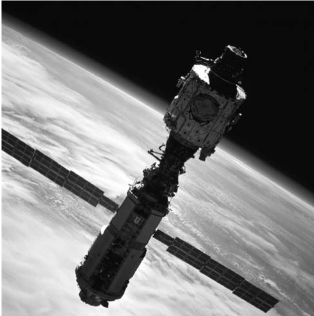
Figure 3. The FGB mated to Node 1 during STS 88 in December 1998 (NASA photo). This figure is available in full color at http://www.mrw.interscience.wiley.com/esst .
