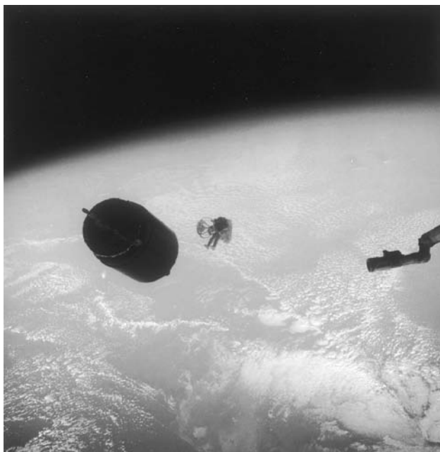
Figure 3. An astronaut wearing the MMU is seen approaching the Westar VI satellite that he will capture for return to Earth.
