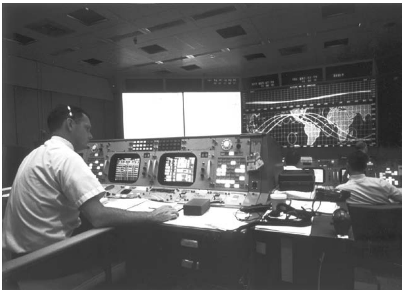
Figure 5. A typical console for Gemini and Apollo featured two CRT displays, intercom panel, event and status lights, and command switches (photo courtesy of NASA; JSC-#68-49299). This figure is available in full color at http://www.mrw.interscience.wiley.com/esst .
