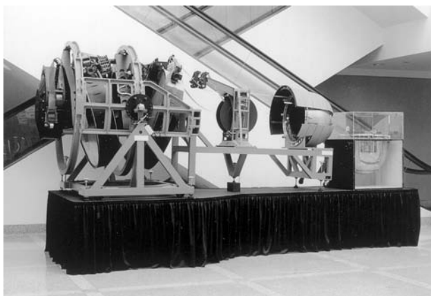
Figure 1. Corona photographic satellite viewed from the side. Note on the left the two panoramic cameras for stereoscopic photographs and the film capsule on the right. This figure is available in full color at http://www.mrw.interscience.wiley.com/esst .
