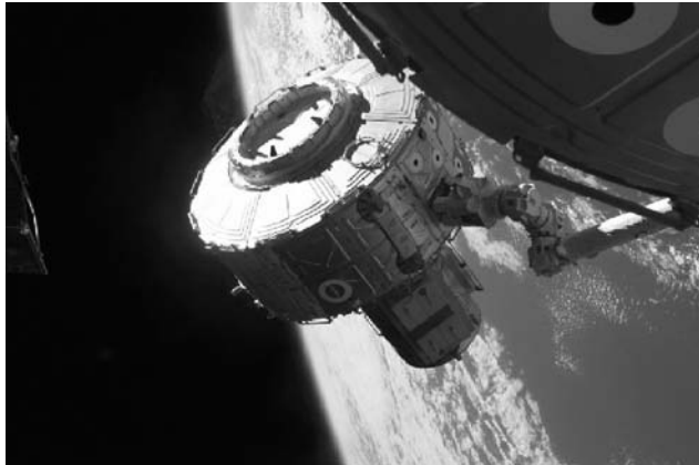
Figure 11. The Quest airlock is mounted to the ISS (NASA photo). This figure is available in full color at http://www.mrw.interscience.wiley.com/esst .
