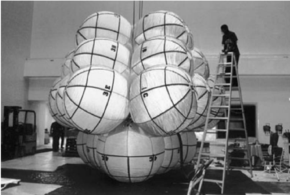
Figure 8. One of the many airbag test performed prior to lift-off. Each lobe of the airbags consists of six spheres, with four lobes, one for each of the pedals. The airbags total 16 feet from the ground to the top. (Image courtesy of JPL/NASA.)
