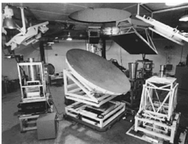
Figure 4. Stationary equipment room below BWG Antenna. This figure can also be seen at the following website: http://deepspace.jpl.nasa.gov/technology/95_20/ant_6.htm . This figure is available in full color at http://www.mrw.interscience.wiley.com/esst .
