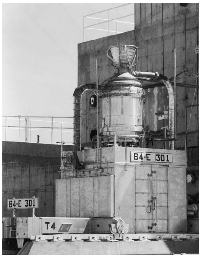
Figure 10. KIWI-B4E at the test cell.
