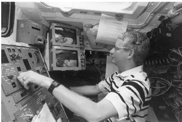
Figure 1. The author is seen “flying” Discovery’s robot arm maneuvering EVA astronauts to various work sites on the Hubble Space Telescope during STS-82. Television monitors provide a view of the EVA activities in the payload bay. This figure is available in full color at http://www.mrw.interscience.wiley.com/esst .
