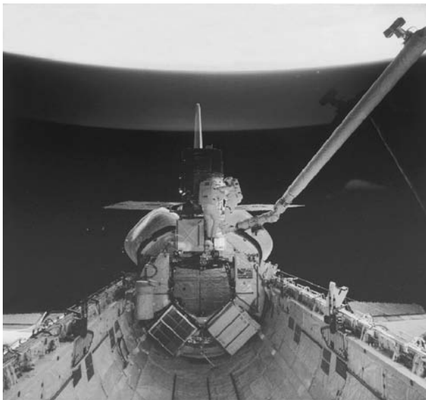
Figure 2. Two Mission Specialist astronauts repair the “captured” Solar Maximum Mission satellite. The satellite is latched into a fixture at the aft end of Challenger's payload bay. The astronauts use the RMS as a “cherry picker” for moving access to the satellite work site.
