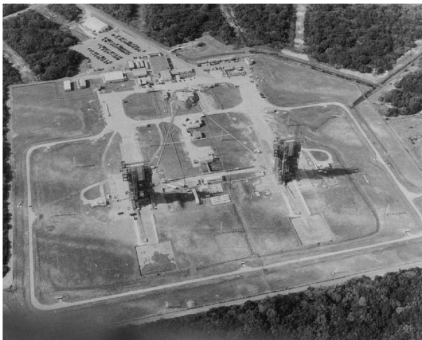
Figure 2. Complex 17, which is still active, is shown in the 1991 photograph, taken from the east. Note the Delta vehicle on the left pad, 17B. Even though the service structure surrounds the vehicle, the thrust augmenting boosters are visible. The wedge-shaped blockhouse is located at the intersection of the covered cable trenches running west from each pad (USAF photo). This figure is available in full color at http://www.mrw.interscience.wiley.com/esst .
