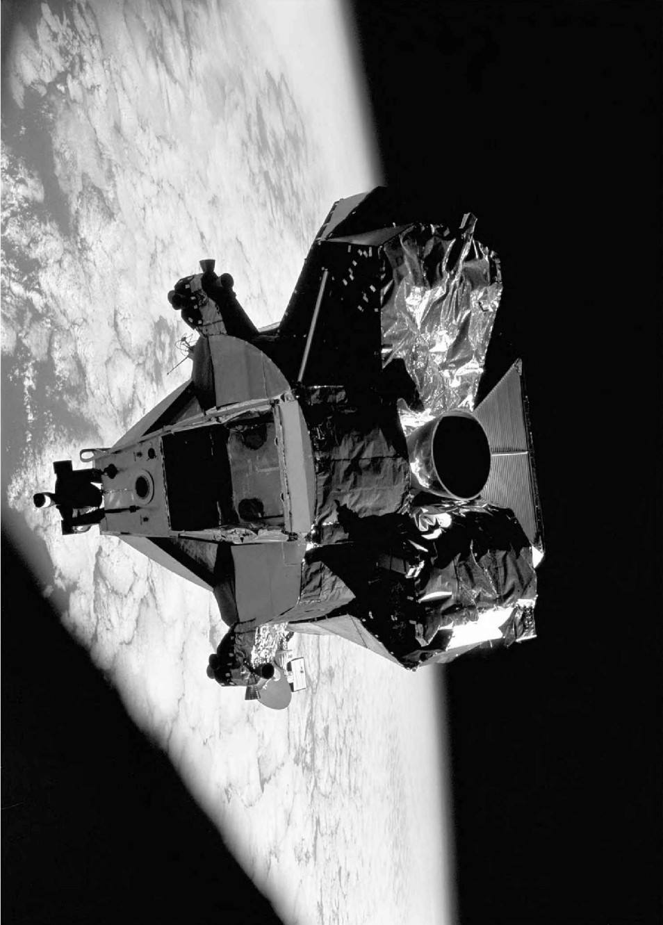
Spider's ascent stage, viewed by Dave Scott from the windows of the command module Gumdrops. Clearly visible is the ascent engine and the square hatch.
