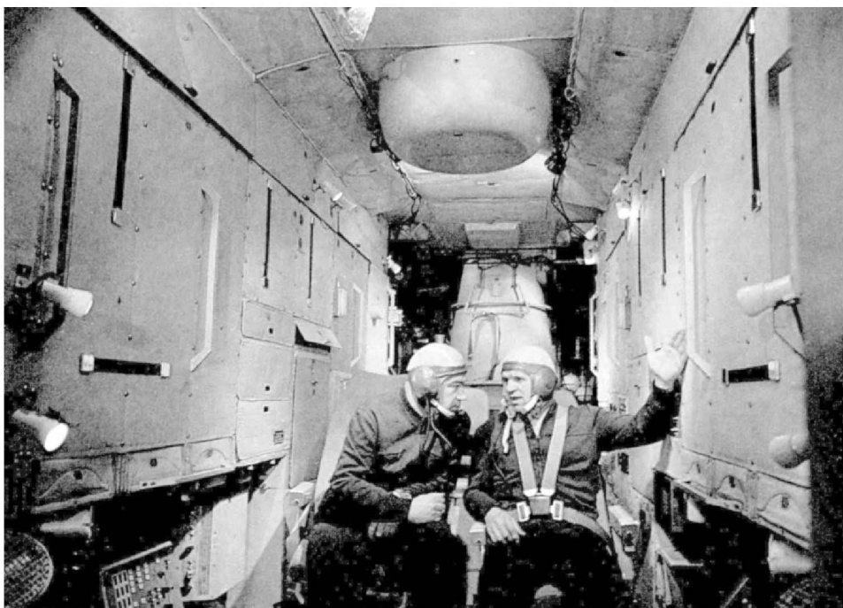
The Soyuz 17 crew – Georgi Grechko (left) and Alexei Gubarev – pictured in the working compartment of the Salyut station trainer. The large white cone in the background is the OST-1 solar telescope.
