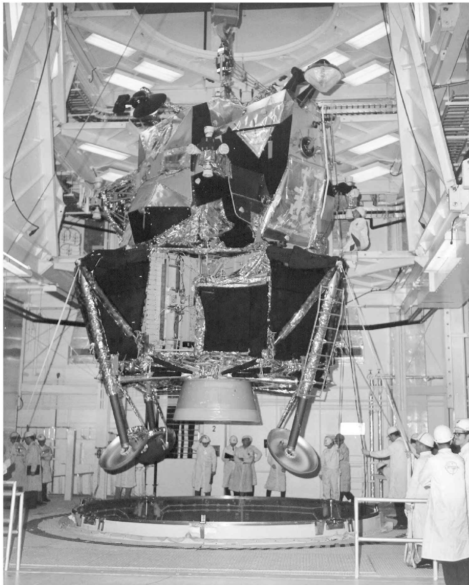
Grumman's spidery lander is prepared for its first flight to the Moon: Apollo 10 in May 1969. Note the prominent descent engine and the craft's four legs, shown here folded into their launch configuration.
