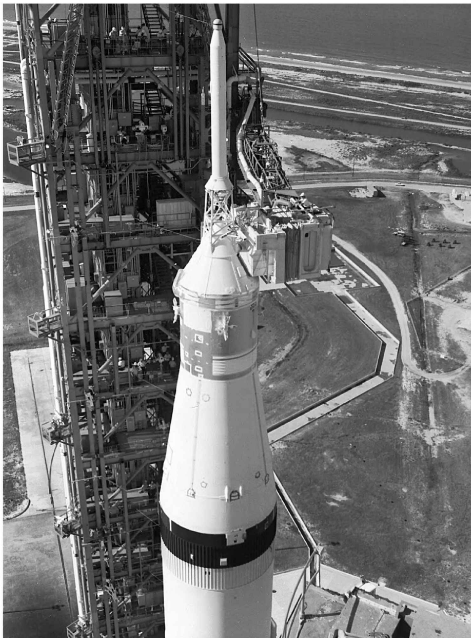
Rollout of the Apollo 11 vehicle in May 1969. Note the white room alongside the command module's hatch and the escape tower which would pluck Armstrong, Collins and Aldrin away in the case of an emergency.
