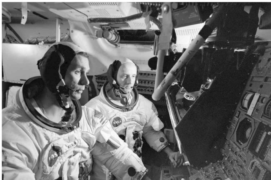
Gene Cernan (left) and Tom Stafford rehearse their procedures in a mockup of the lunar module cabin. The lander’s main instrument panel is visible to the far right of this image.
