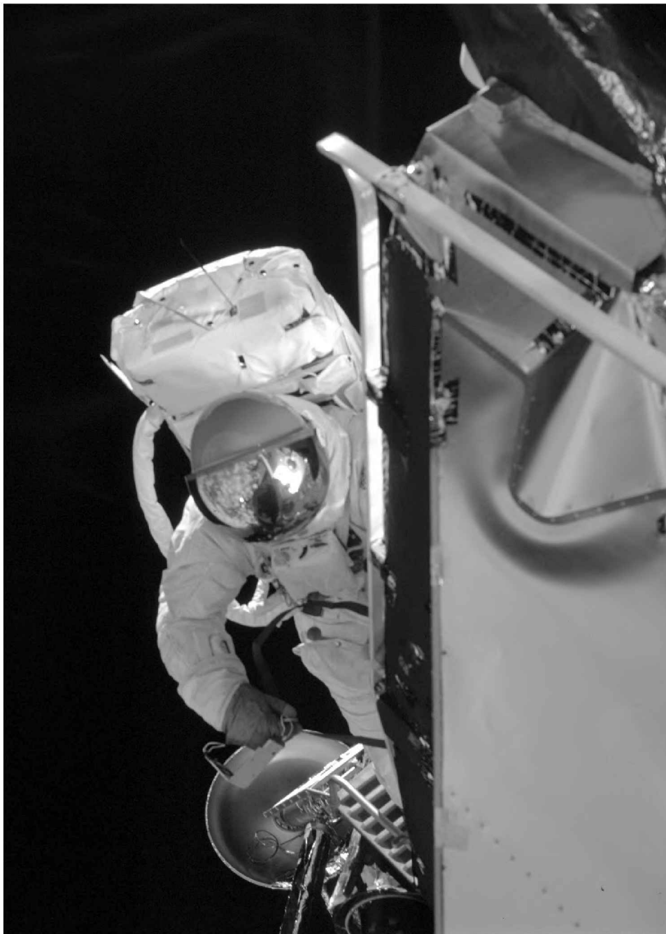
Rusty Schweickart, clad in a lunar-style EVA suit with the massive backpack, emerges onto Spider's porch. Note the circular footpad, visible just below his right hand.
