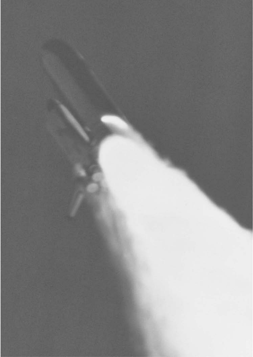
Almost 59 seconds into Challenger's ascent, an ominous flame from the breached right-hand Solid Rocket Booster begins to impinge on the External Tank.
