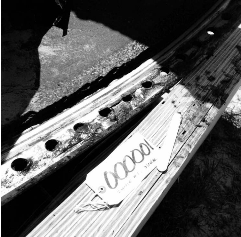
Remains of O-ring seal 'tracks' and putty in recovered debris from STS-51L's right-hand Solid Rocket Booster.
