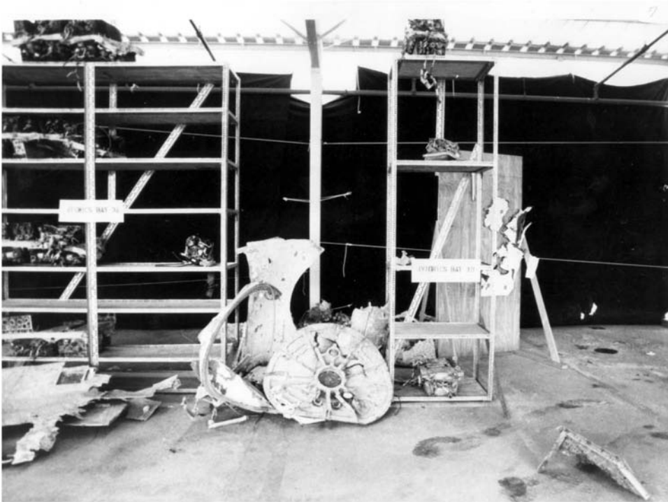
Thirty per cent of Challenger’s structure was recovered from her Atlantic grave. Among the debris was the crumpled airlock hatch, originally housed in her middeck.
