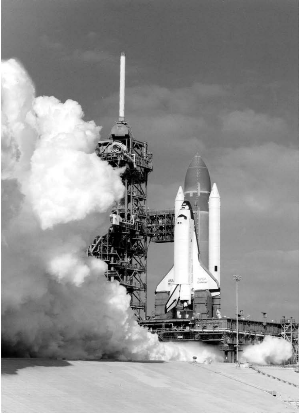
Challenger undergoes the first Flight Readiness Firing of her three main engines on December 18th 1982. Note the unusual 'butterfly and bullet' combination of the Shuttle stack, consisting of the orbiter, External Tank and twin Solid Rocket Boosters.
