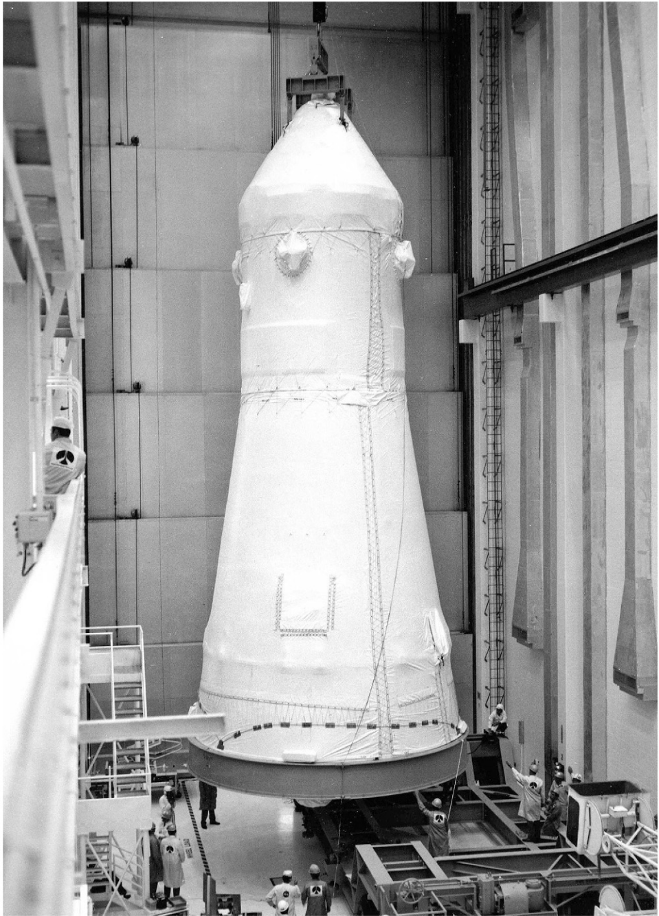
The Apollo 12 spacecraft is hoisted on 30 June 1969 ready for stacking with its launch vehicle.
