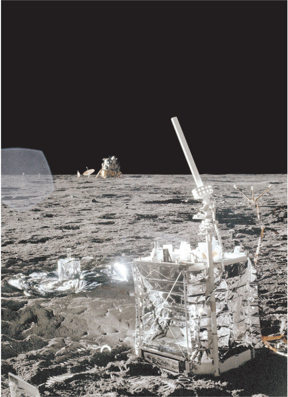
The central station with its antenna pointing at Earth, the seismometer and the magnetometer. In the distance are Intrepid, the S-band antenna, the draped flag and (in the lens flare) the television camera and the solar wind collector sheet.
