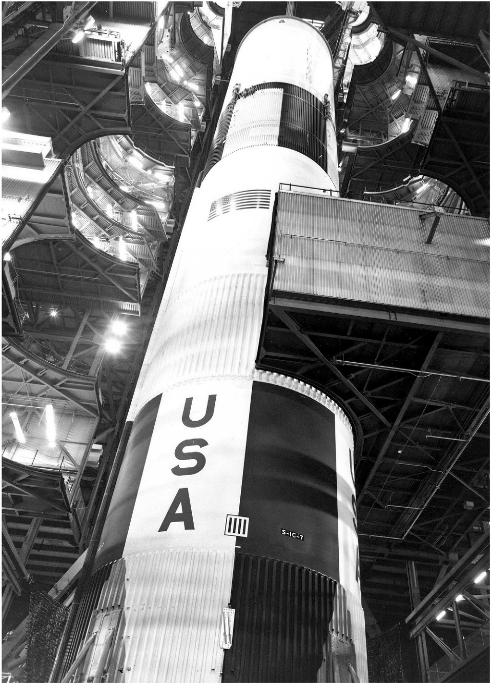
The stacked S-IC and S-II stages of the Apollo 12 space vehicle in the Vehicle Assembly Building on 21 May 1969.
