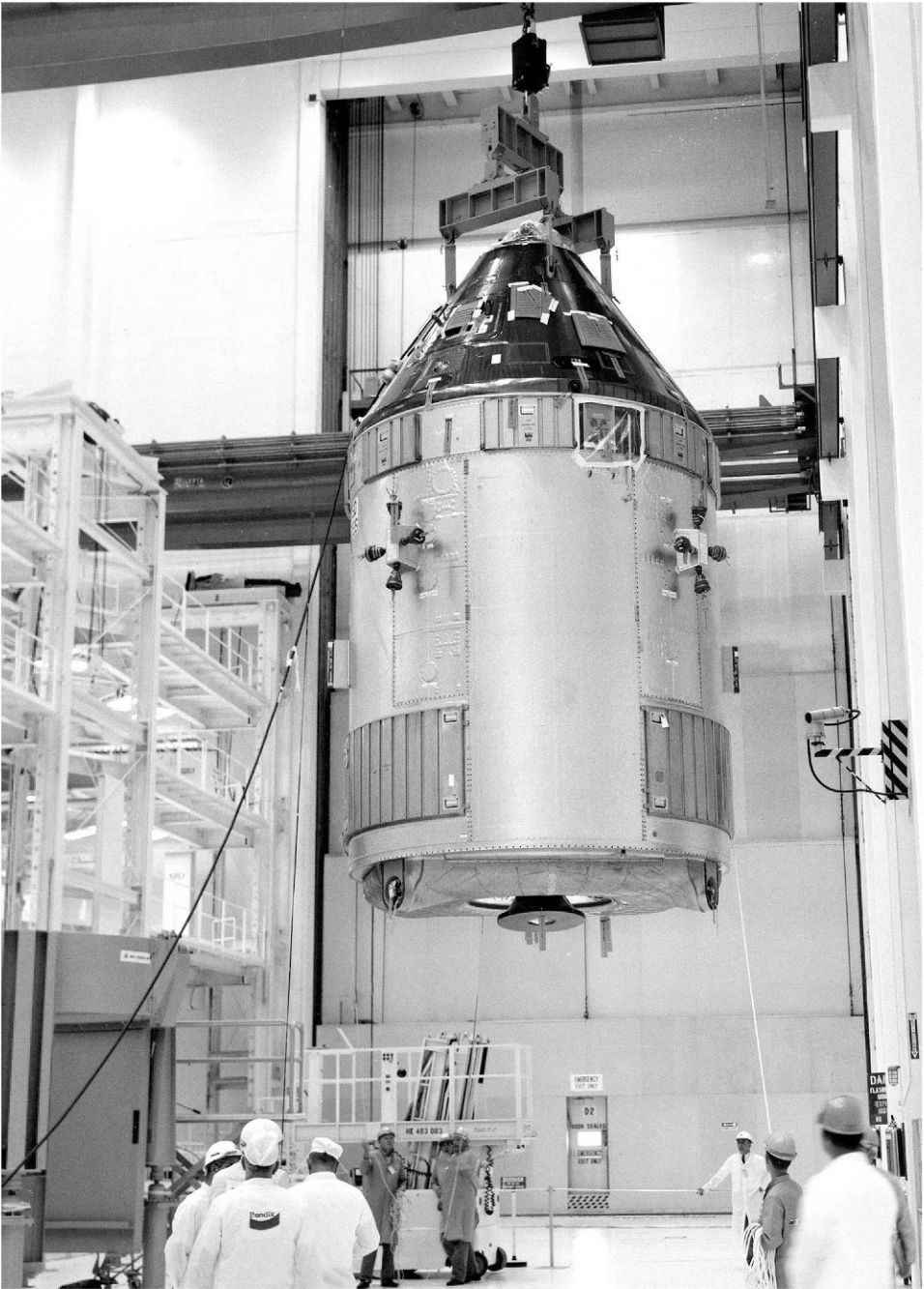
The Apollo 12 command and service modules on 13 June 1969 awaiting the engine bell of its service propulsion system.
