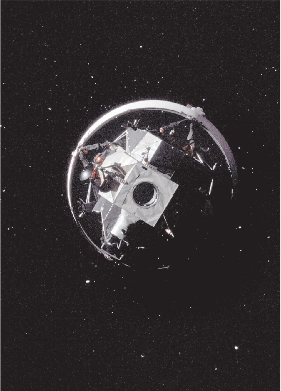
A view of the S-IVB with the lunar module on top, during the transposition and docking sequence.
