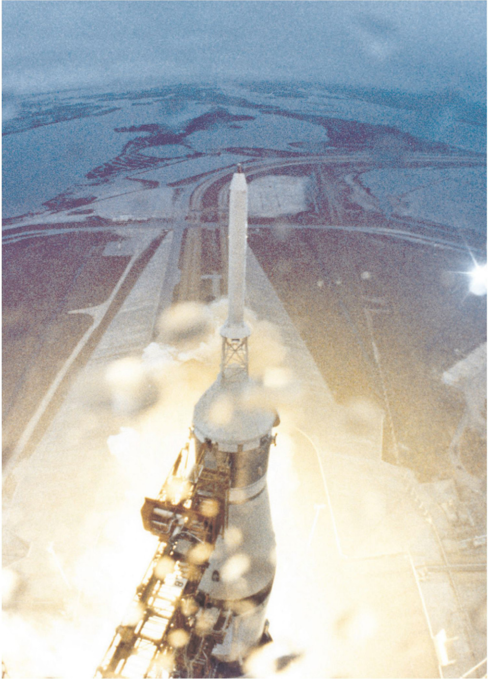
Viewed from the top of the tower, the S-IC has lit its five F-1 engines, but the vehicle has yet to be released. Note the droplets of rain on the camera's lens.
