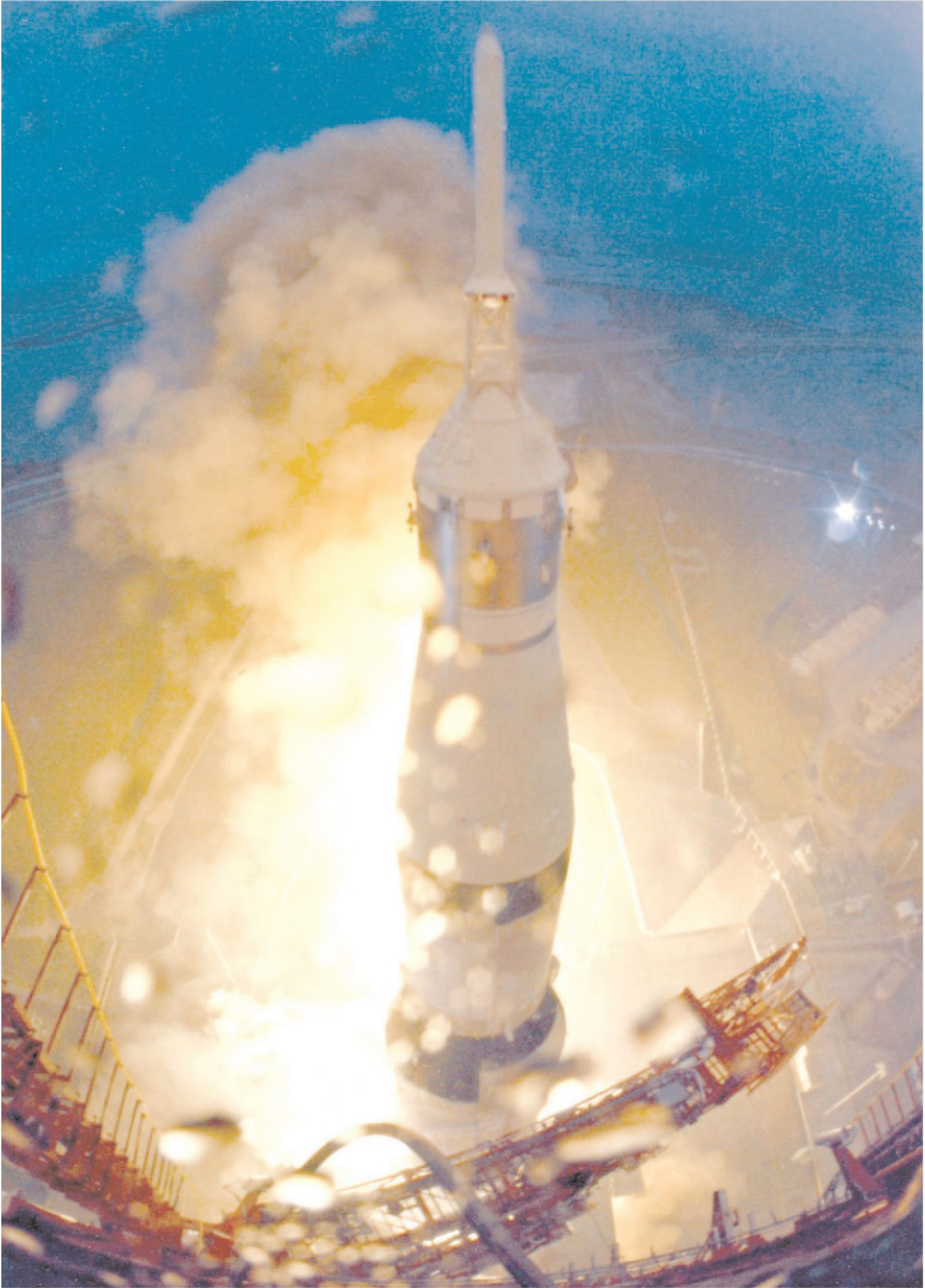
The swing arms rotate clear as Apollo 12 initiates its ascent.
