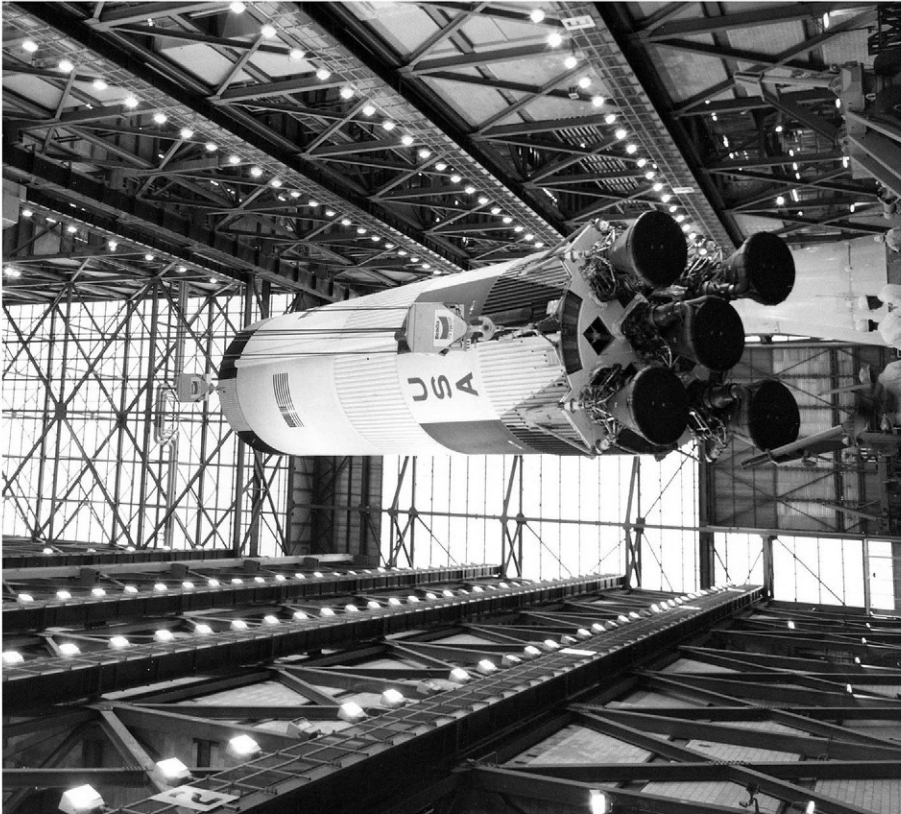
The S-IC stage of the Apollo 12 space vehicle is hoisted upright in the Vehicle Assembly Building on 7 May 1969.
