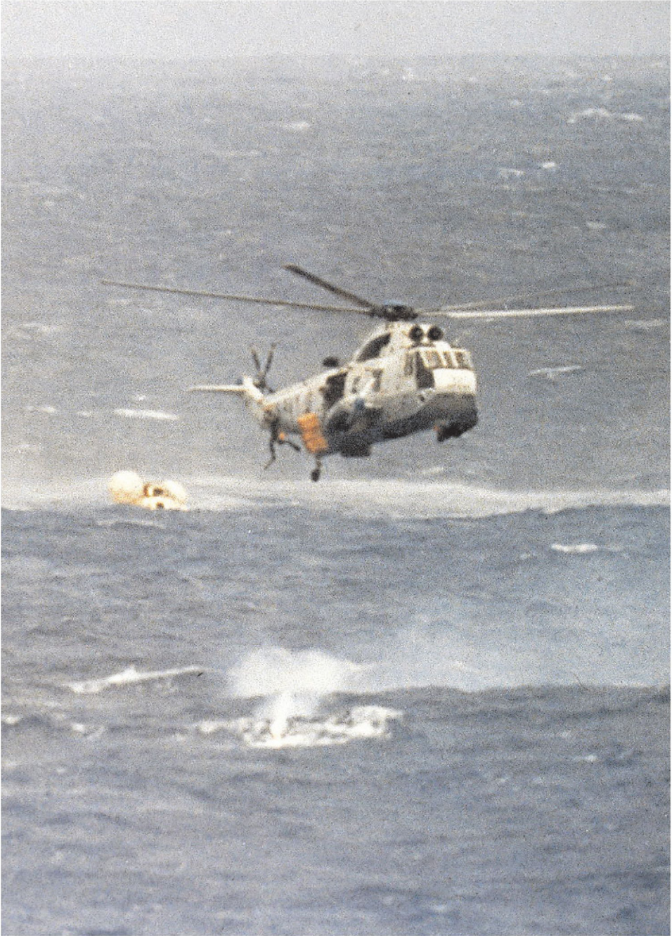
Now that the airbags on the command module have flipped it into the apex-up orientation, the Swim 1 helicopter drops swimmers to start the recovery effort.
