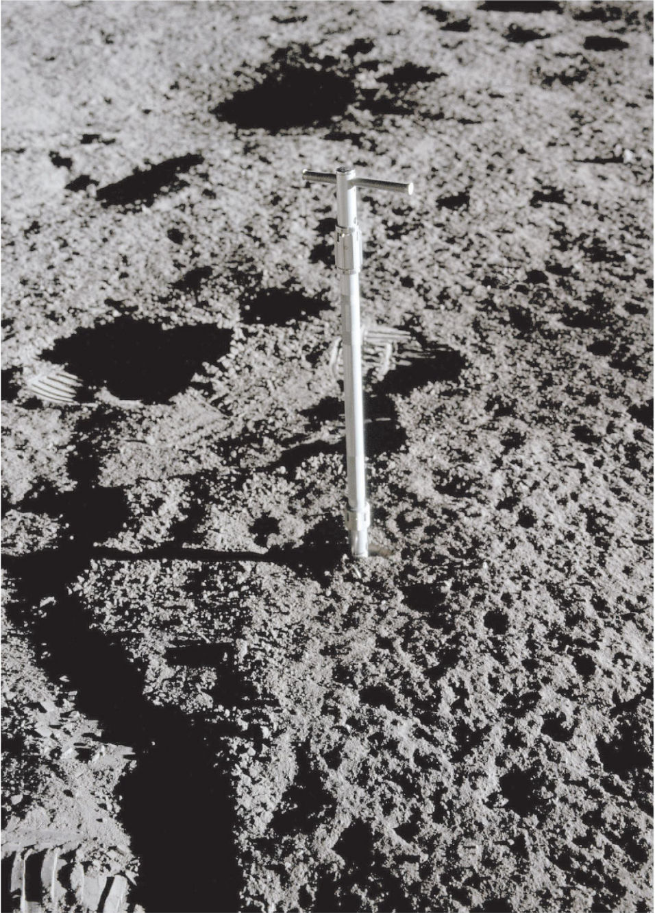
Upon returning to Intrepid at the end of the first moonwalk, Al Bean obtained a core sample. Here the tube is almost completely embedded in the ground, and the extension handle is visible.
