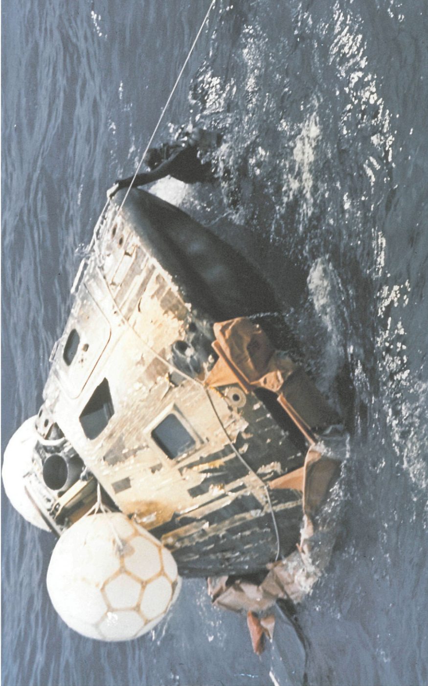
Attaching the flotation collar to the command module in a rough sea.
