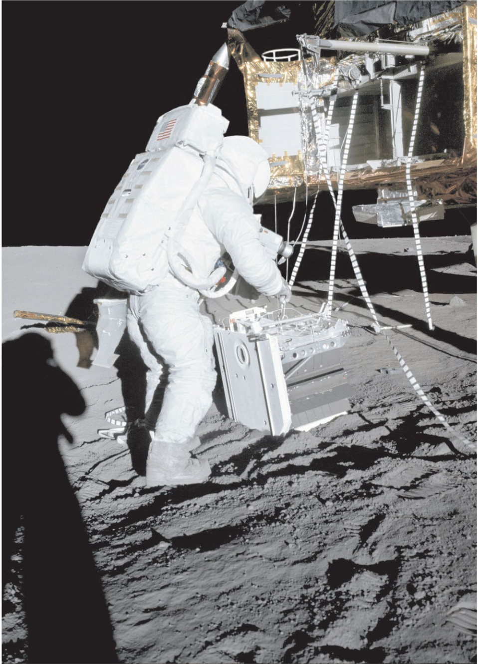
Al Bean has retrieved the RTG subassembly of the ALSEP from the SEQ bay.
