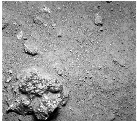
Stereoscopic images of 3-inch squares of the lunar surface taken by Al Bean using the close-up camera devised by Tommy Gold in order to investigate the fine structure of the undisturbed regolith, although in one case Bean used it to photograph the imprint of his boot.
