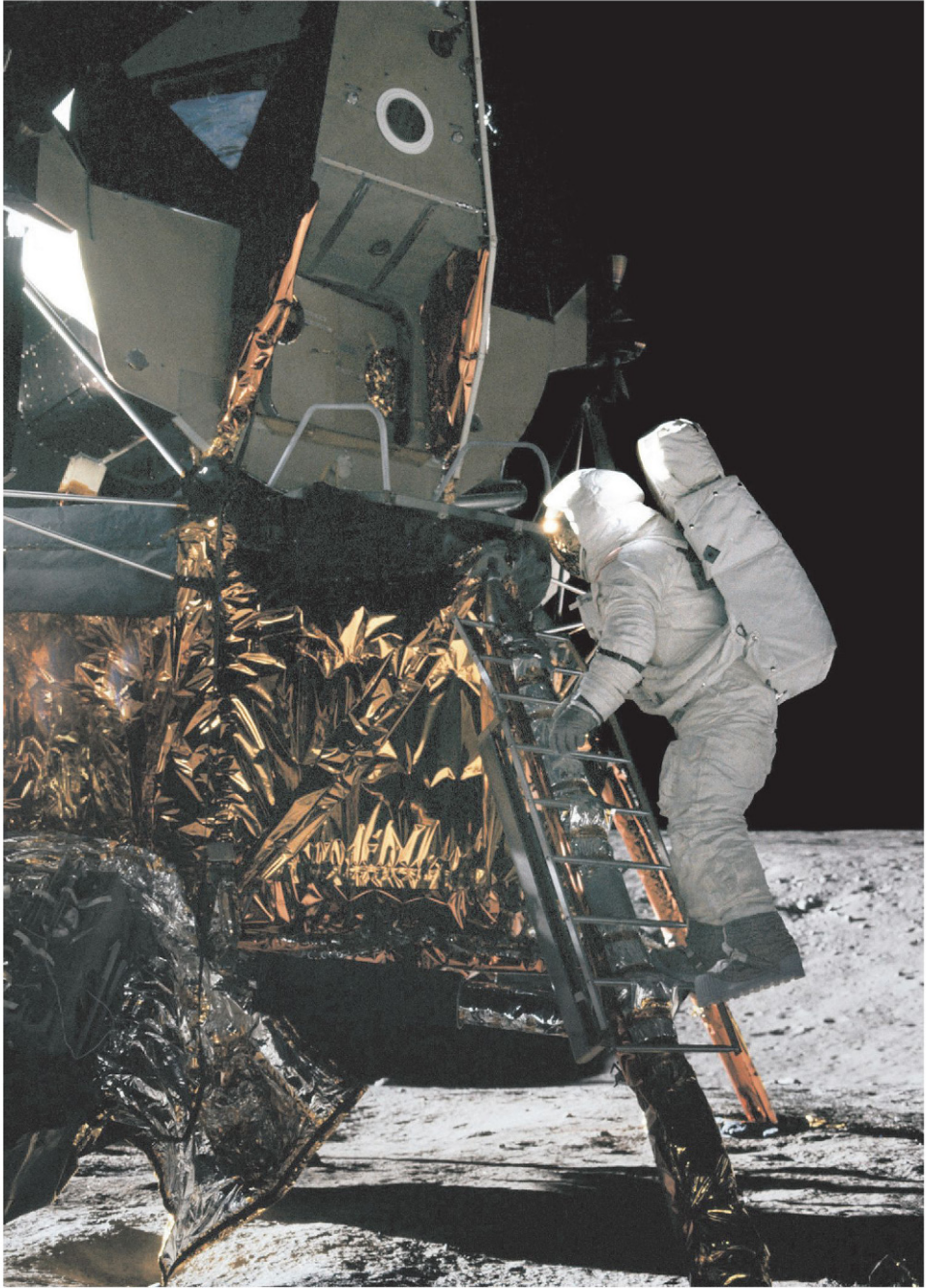
Al Bean descends the ladder. Note that he has left the hatch partially open.
