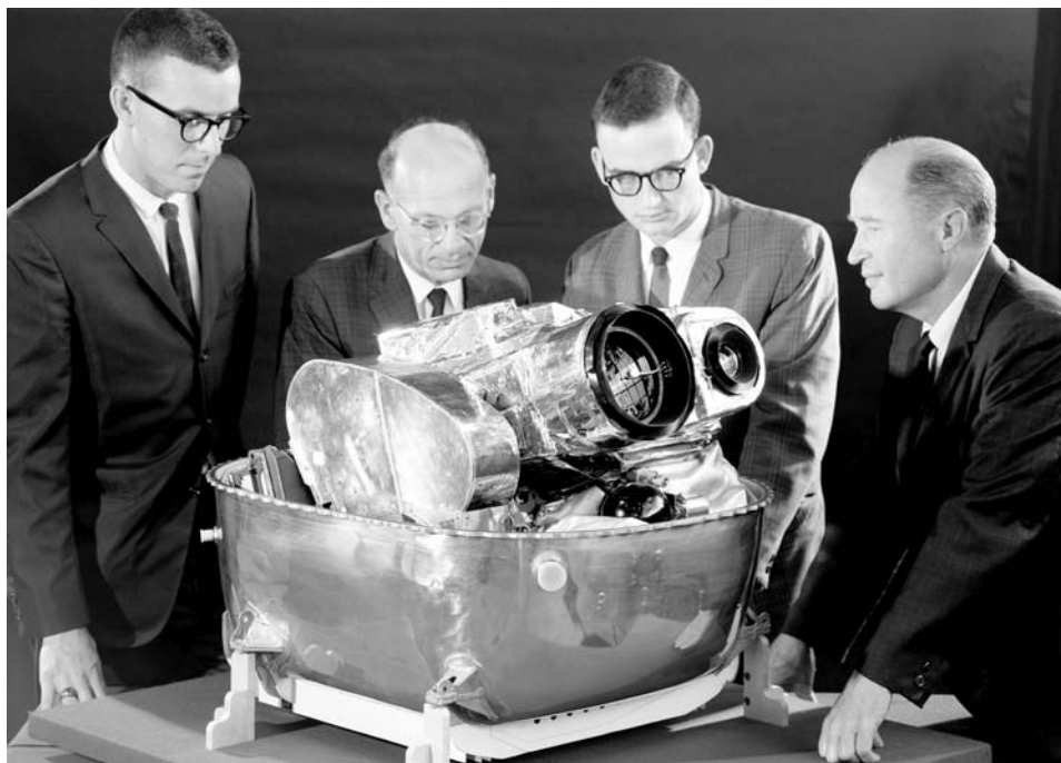
The two-lens camera of the Lunar Orbiter photographic system.
