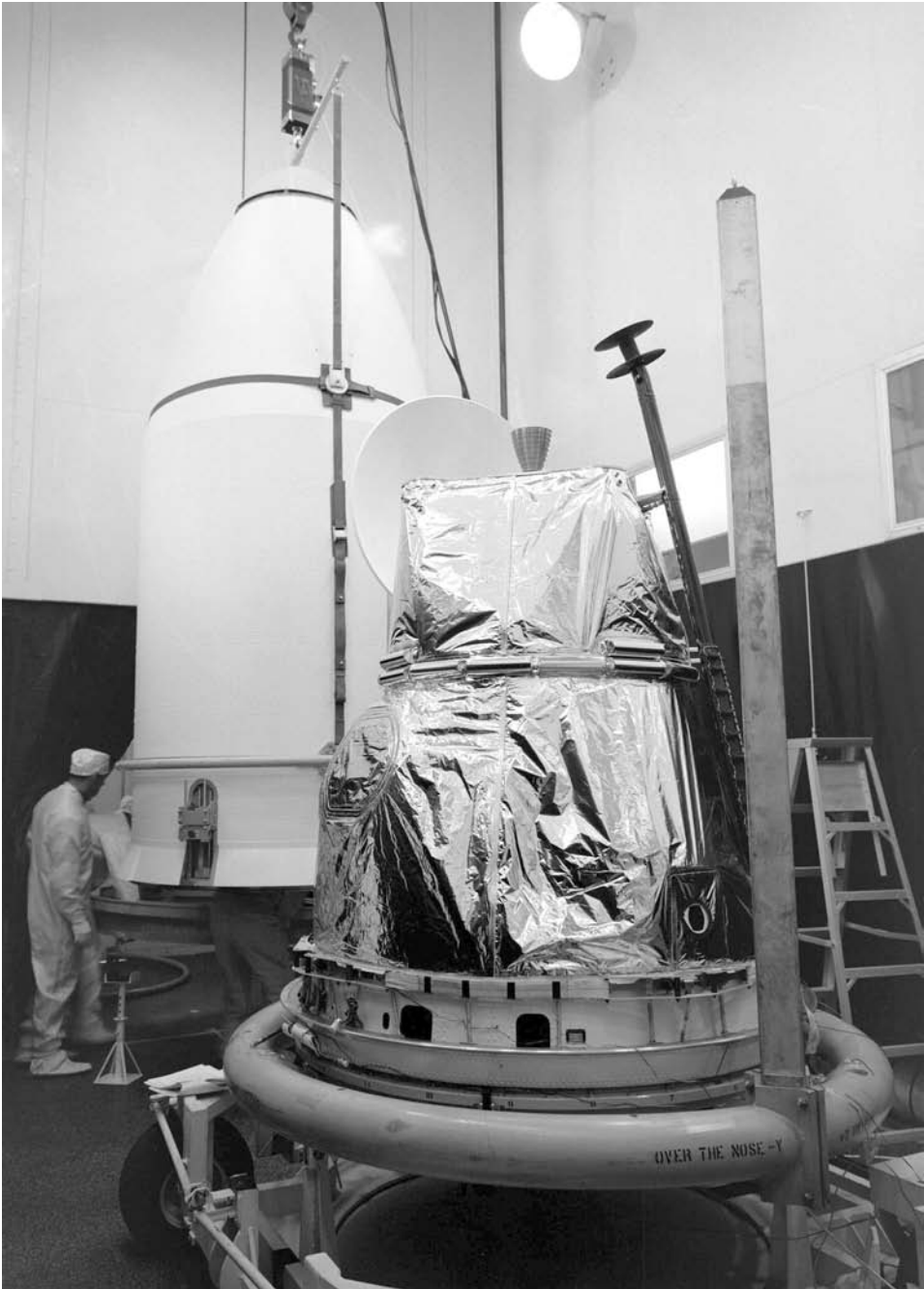
Preparing to fit the aerodynamic shroud on the Lunar Orbiter 1 spacecraft, wrapped in its thermal blanket.
