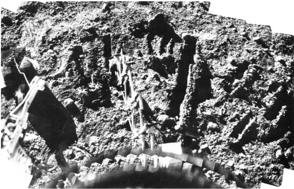
Surveyor 7's soil mechanics surface sampler at work on 21 January 1968.
