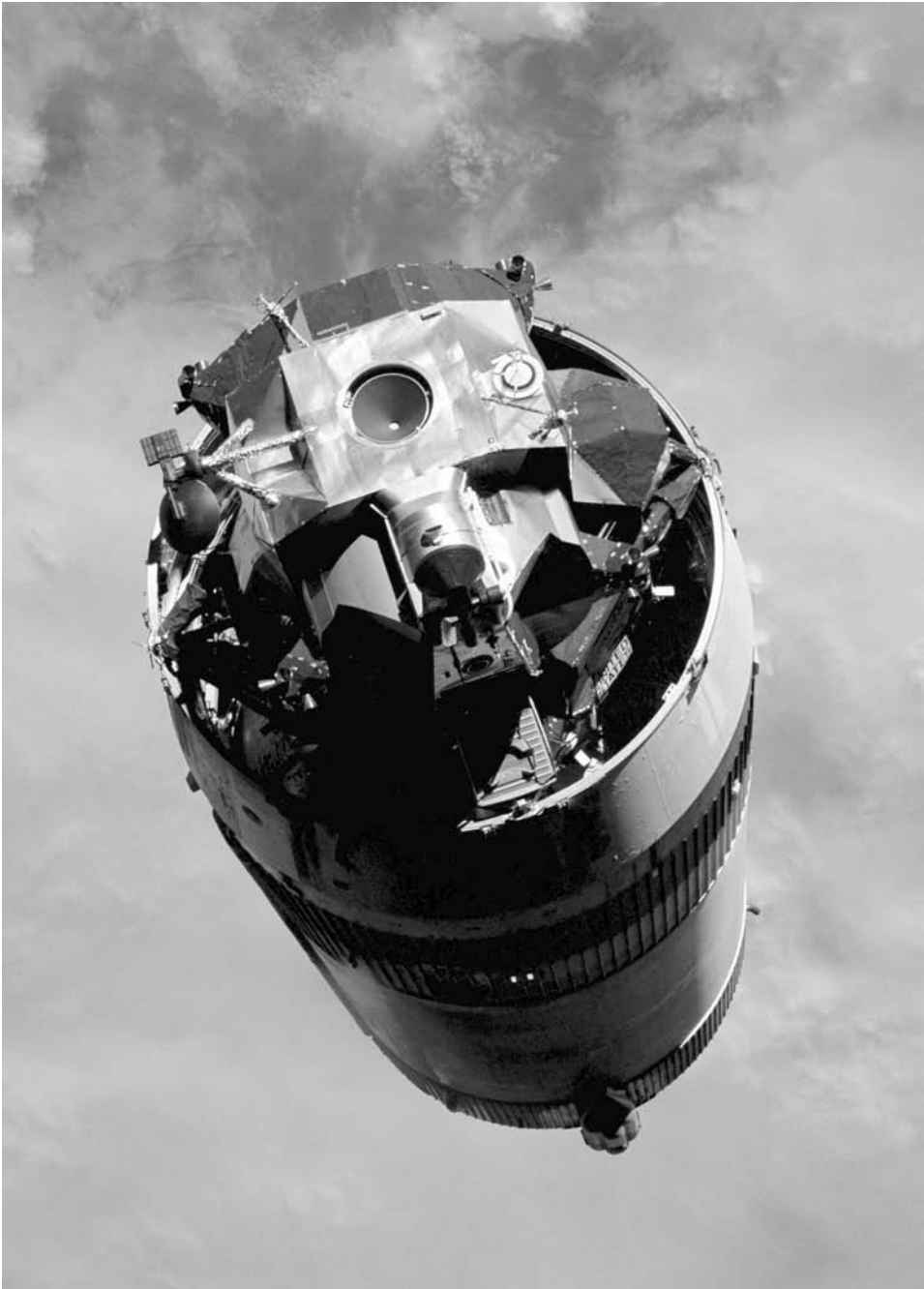
Apollo 9's S-IVB with the Lunar Module 'Spider' exposed.
