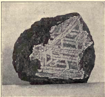
METEORITE FROM CAÑON DIABLO, ARIZONA Surface polished. Showing method of crystallization.
