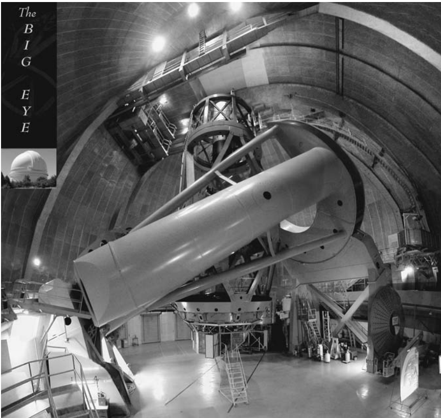
The 200-inch (5.08-m) Hale Telescope at the Mount Palomar Observatory in California was the largest optical telescope in the world until the 1970s. (Dr. T. H. Jarrett, Caltech)
