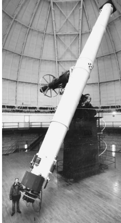
The 40-inch (1.02-m) Yerkes Observatory refractor is the world's largest refracting telescope. (Yerkes Observatory photograph EIB6551)
