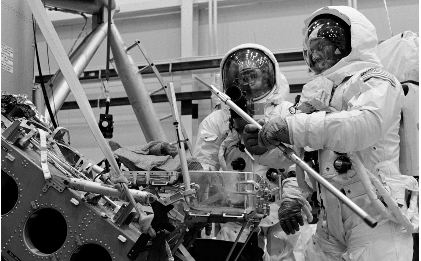
Buzz Aldrin attaches the extension handle to a tube for a 'core' sample.
