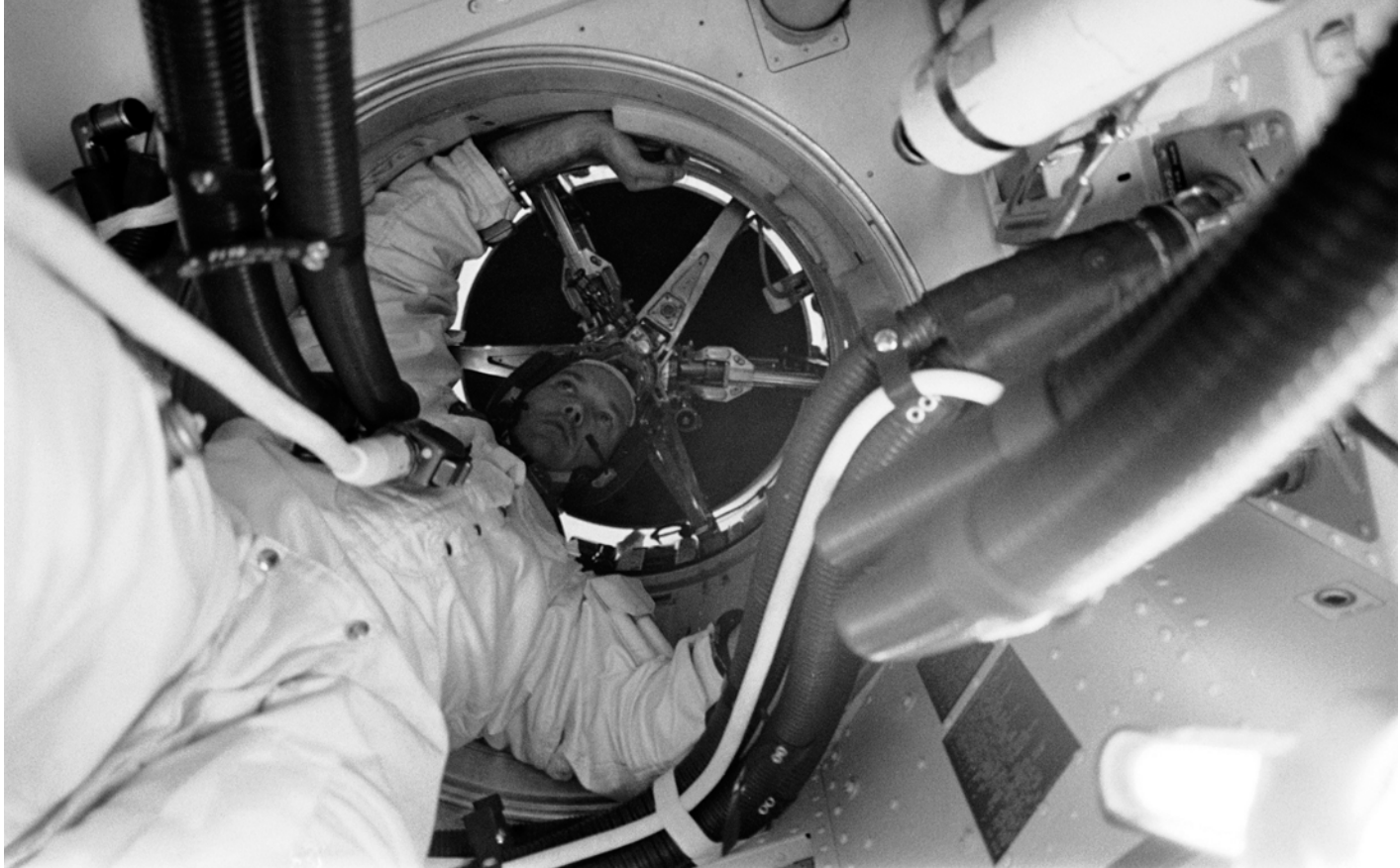
Having removed the apex hatch, Mike Collins prepares to remove the probe assembly.
