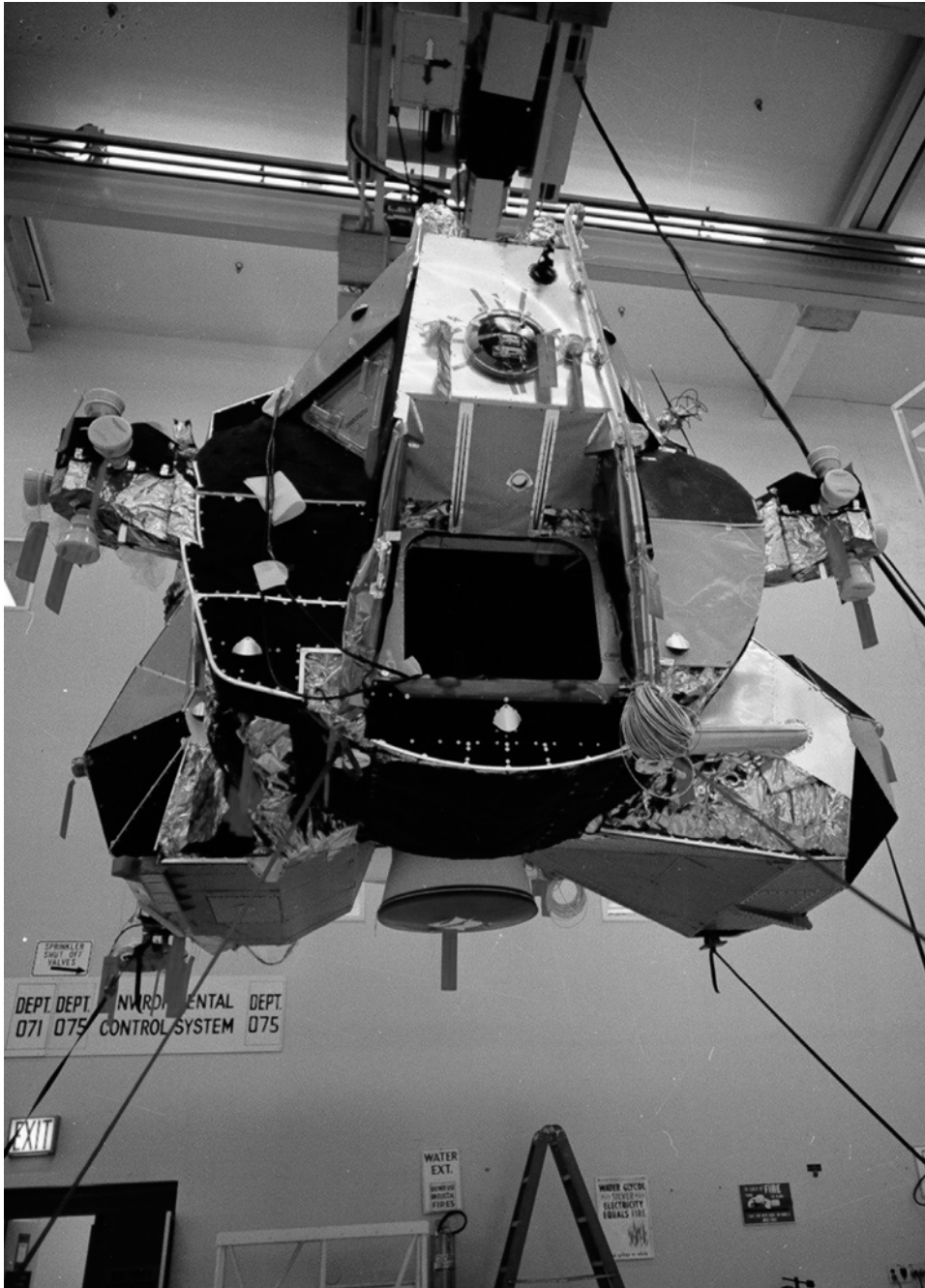
At the Grumman plant on 4 January 1969, the ascent stage of LM-5 is hoisted for shipment.
