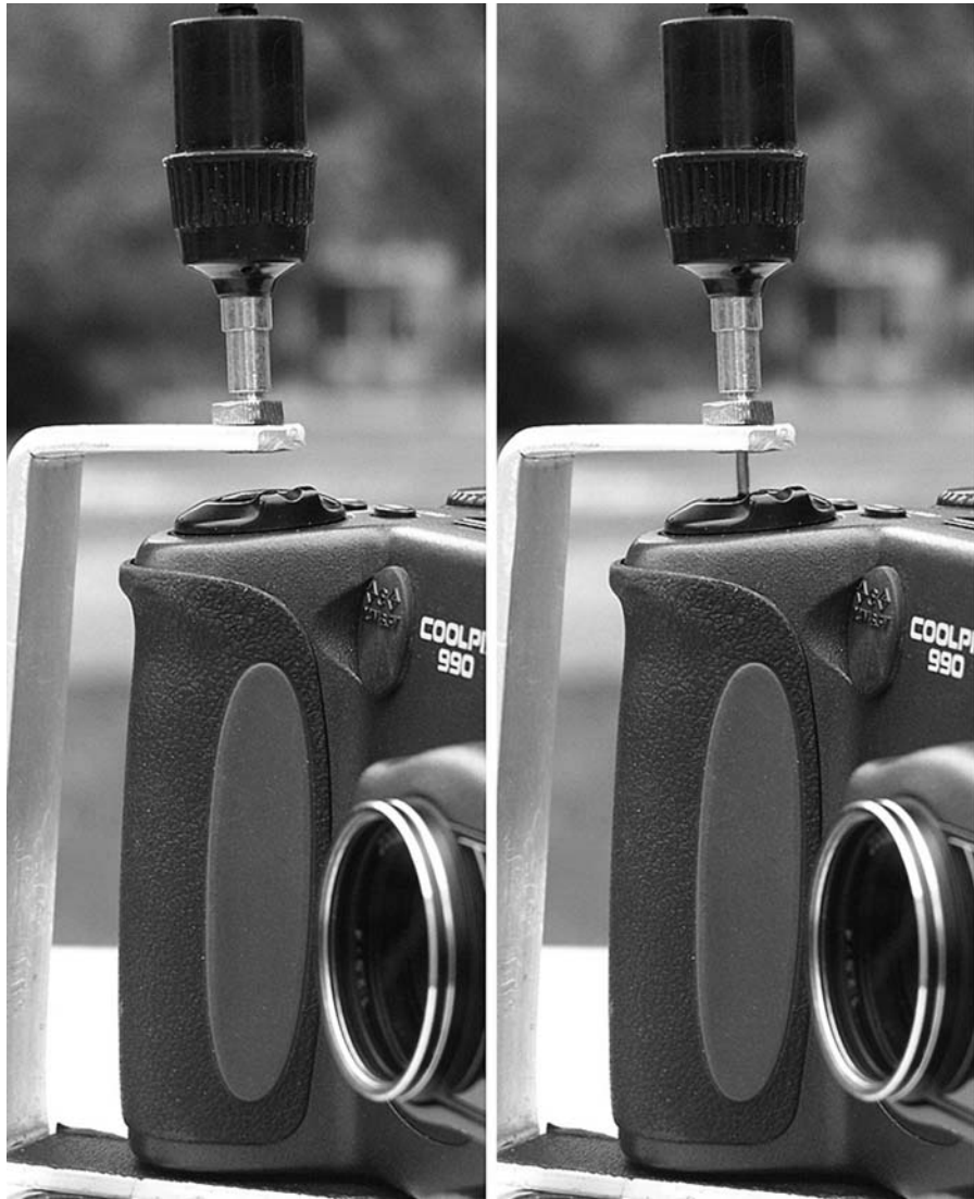
Figure 8.4. Adapting an air-activated cable release to a CP990. The left hand photo is in standby mode, and the right hand is with the plunger depressing the shutter button.
