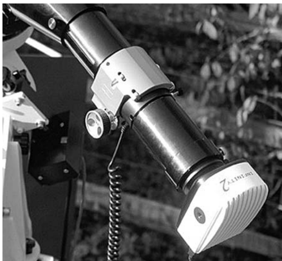
Figure 8.10. The Luminera video camera can shoot at 200 fps, but lower frame rates improve the resolution. Greg Piepol.
