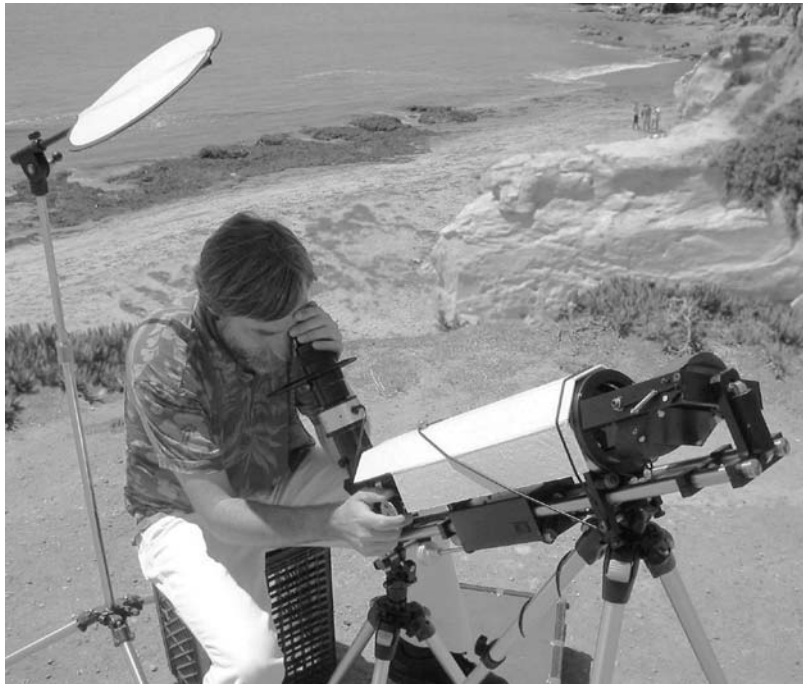
Figure 6.10. Polar-mounted telescope for H-alpha observing. Note the movable screen for shading the observer. Robert Hess.
