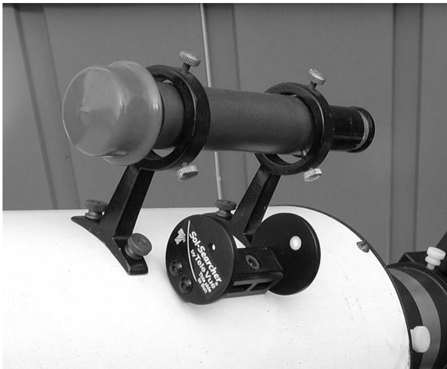
Figure 2.4. Use a pinhole device, such as the commercial unit shown, or watch the shadow of the telescope on the ground to center the Sun in the telescope’s field of view.
