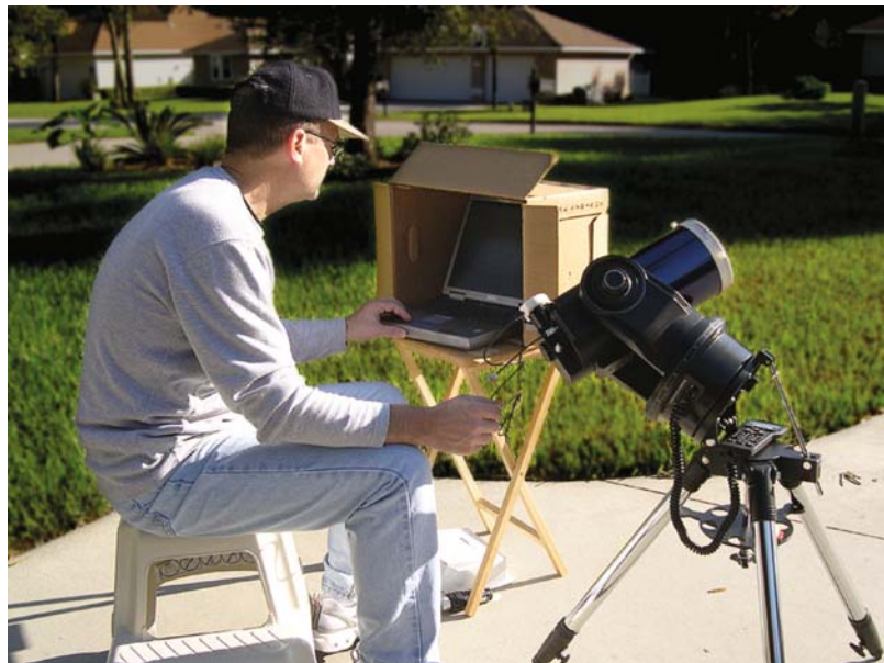
Figure 8.8. Solar imager Howard Eskildsen with his portable setup for digital photography. The opened-face box serves to shade the laptop from the direct light of the Sun.
