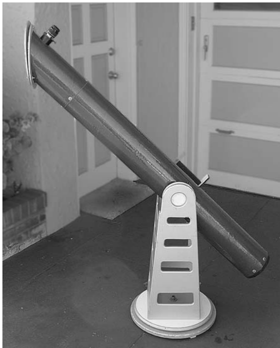
Figure 3.7. A Dobsonian solar telescope with a 150 mm f/10 primary mirror. Ray Cash.
