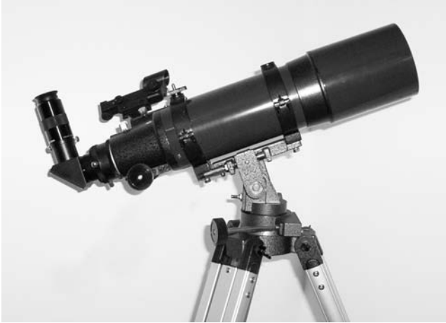
Figure 10.1. The authors 4" f5 refractor, a great wide-field telescope.
