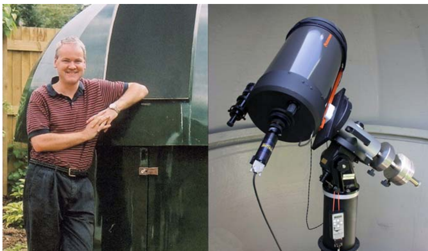
Figure 1.13. Jeremy Shears of Bunbury Observatory, Cheshire, specializes in spotting dwarf novae as they go into outburst. Originally his dome housed a 100-mm Takahashi refractor, but a Celestron 11 (280 mm) on a Gemini G41 mount is now used for more sensitive photometry. Images: Jeremy Shears.
