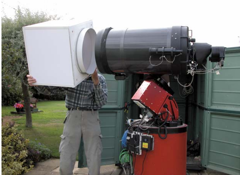
Figure 7.4. The author's flat-field box being mated to his Celestron 14 Schmidt-Cassegrain telescope.
