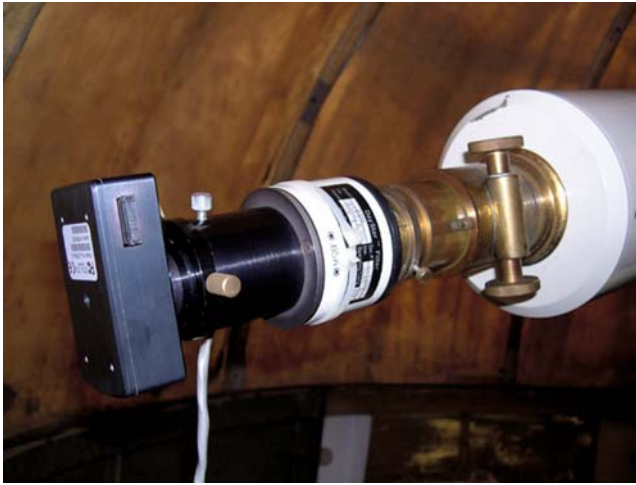
Figure 3.4. Dave Tyler's high-speed Lumenera CCD camera attached to a 0.6-Å H-Alpha Daystar filter at his refractor's focuser end, enabling limb prominences and H-alpha surface details to be imaged. Image: Dave Tyler.
