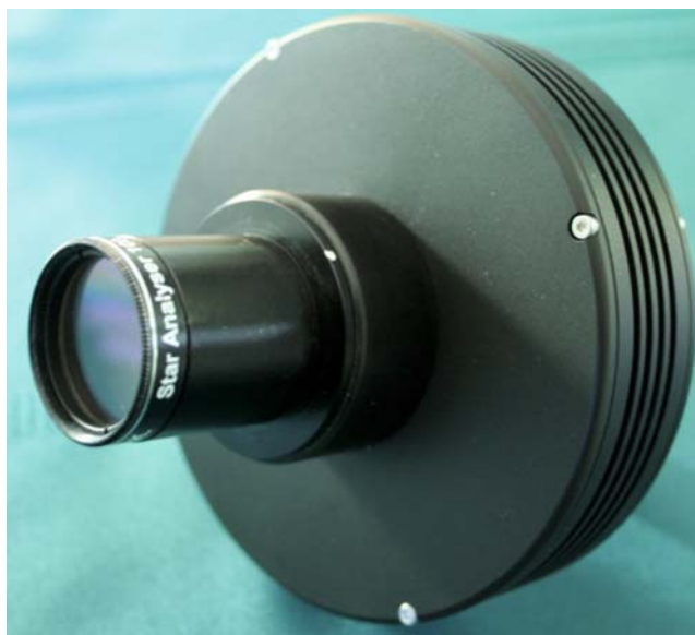
Figure 2.22. The Paton Hawksley Star Analyser, seen here attached to Robin Leadbeater's ATiK CCD camera, is an inexpensive ($150) way of obtaining spectra using a webcam on bright stars or a cooled CCD camera on novae or even bright supernovae. It features a high-efficiency 100 lines per millimeter blazed diffraction grating and screws into any 31.7-mm filter thread. With an 80-mm telescope and a simple, unmodified webcam, stars down to magnitude 4 can be analyzed. www.patonhawksley.co.uk/staranalyser.html . Image by kind permission of Robin Leadbeater.
