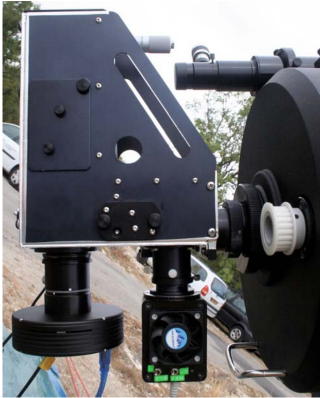
Figure 2.21. The spectrograph of Robin Leadbeater, fixed to the back of his 280-mm-aperture Celestron 11. An ATIK ATK16-IC camera is used to record the spectra of a nova or variable star while a modified webcam is used as an autoguider. The spectrograph is the LHIREsIII unit developed by the French AUDE Astronomy Group and sold in kit form. ( www.astrosurf.com/thizy/lhires3/index-en.html .) The unit is fitted with two diffraction gratings, one of 2400 lines per millimeter resolution and a lower resolution one of 150 lines per millimeter. The lower resolution grating is used for fainter objects. Image by kind permission of Robin Leadbeater.
