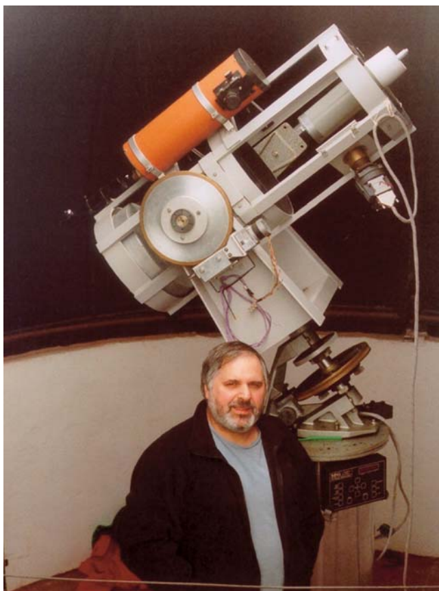
Figure 1.4. Denis Buczynski with his fork mounted 33-cm f/3.5 Newtonian, which was used to obtain the IP Peg light-curve in the next figure.
