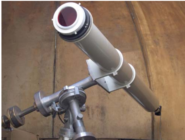
Figure 3.3. Dave Tyler's 6-inch (152.4 mm) f/15 refractor at Flackwell Heath UK. This is used solely for H-alpha imaging. Note the red energy rejection filter/76-mm aperture stop. Image: Dave Tyler.
