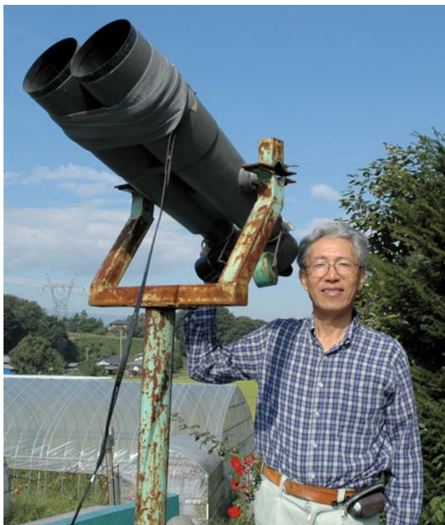
Figure 2.17. Japan's Kesao Takamizawa of Saku-machi, Nagano, Japan is shown here with a pair of 25 \times 150 mm Fujinon comet-sweeping binoculars, although his main patrol instrument has been a system similar to that of his countryman Katsumi Haseda: that is, twin 400-mm-focal-length f/4 patrol lenses and 400 ISO film. In total he has discovered two novae, an outburst of the recurrent nova CI Aql, one supernova, two comets (one periodic: 98P/Takamizawa) and a colossal 502 new variable stars! The nova discoveries were V1425 Aql and V2487 Oph. Image by kind permission of Kesao Takamizawa, communicated to the author by Seiichiro Kiyota.
