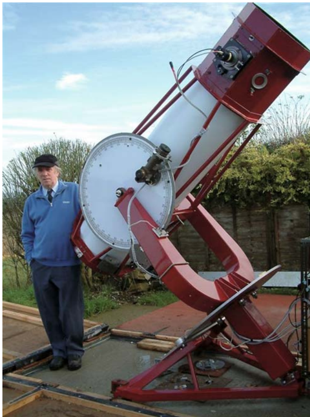
Figure 4.10. British supernova discoverer, and the father of British supernova hunting, Ron Arbour poses with his home-made 0.4-m f/5 Newtonian used for supernova hunting. Most of Ron's earlier 18 discoveries have been made with a 30-cm Schmidt-Cassegrain. Image by kind permission of Ron Arbour.
