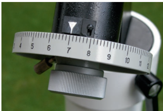
Fig. 3.2. A plastic right ascension setting circle, attached to the same inexpensive Russian “TAL” telescope. The circle is subdivided into increments of 10 min of R.A. equivalent to 2.5° of arc at the celestial equator. For a direct R.A. reading the right ascension circle needs calibrating against a star or sidereal clock, but can also be used simply to offset from a bright star. If the telescope has no sidereal motor drive in R.A., the sky will move by a degree of arc every 4 min on the celestial equator, but this should not be a big problem if the user pushes the telescope to the object immediately after calibrating on a known star.
