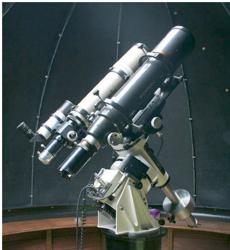
Fig. 4.8. Some fine emission nebula images in this book were obtained by Ian Sharp of Ham, West Sussex, who lives just a short distance from the Caldwell list inventor, Sir Patrick Moore. This is Ian's wide-field set up: an Astrophysics AP900-GTO mount with an Orion ED80 semi-apo refractor and an 80 mm SkyWatcher guide scope, mounted inside Ian's homemade 3.2 m observatory dome (wooden walls and floor with a fiberglass dome).
