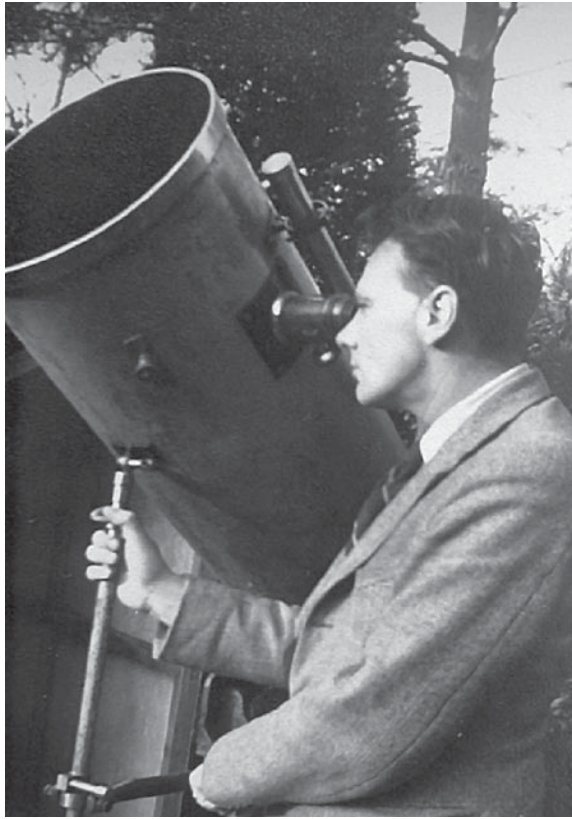
Fig. 1.3. A photograph probably taken around 1955 showing Patrick at the eyepiece of his 12.5-in. alt-azimuth mounted f/6 Newtonian, a telescope which Patrick has owned for over 60 years! Reproduced by permission of Patrick.
