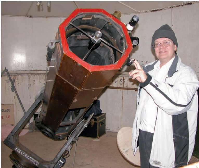
Fig. 1.5. Mars expert Richard McKim observing Mars with Patrick's 15-in. (38 cm) f/6 fork mounted Newtonian in October 2005. The telescope has a rotating top end, which makes comfortable viewing much easier.
