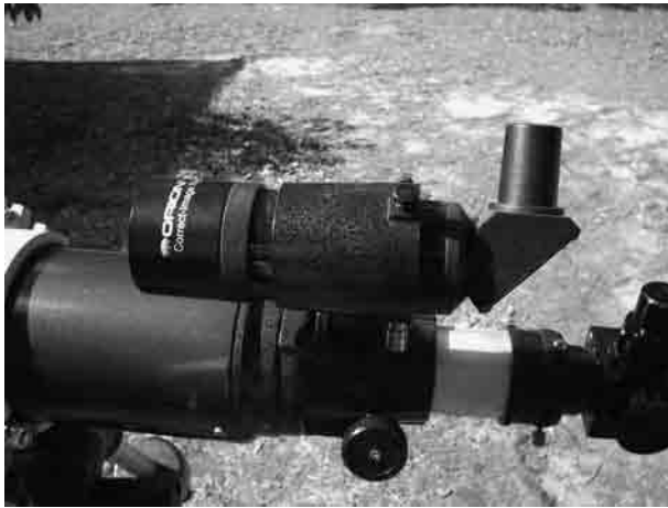
Figure 4.10 A right-angle finder scope. (Credit: Richard W. Schumde, Jr.)
