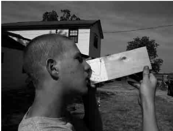
Figure 5.12. A quadrant has a weight, suspended on a string that points straight down. When a quadrant is lined up on a target, one can determine the target's altitude by measuring where the weight is in relation to the protractor. (Credit: Timothy Abbott and Richard W. Schmude, Jr.)
