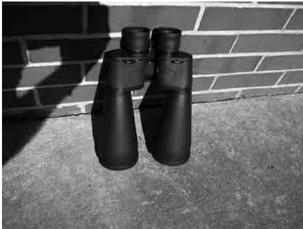
Figure 4.3 A pair of porro prism binoculars. Note that the eyepieces at top are not directly in front of the objective lenses. (Credit: Richard W. Schmude, Jr.)
