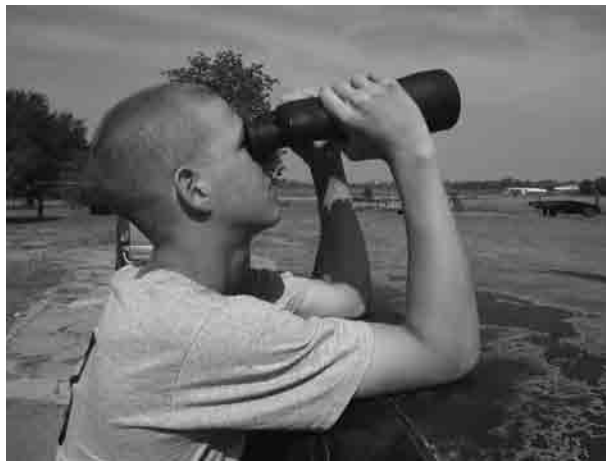
Figure 4.6 The correct way of holding a pair of heavy binoculars. Note that the observer is holding the binoculars near their center of mass and his elbows are on a solid surface. (Credit: Timothy Abbott and Richard W. Schmude, Jr.)
