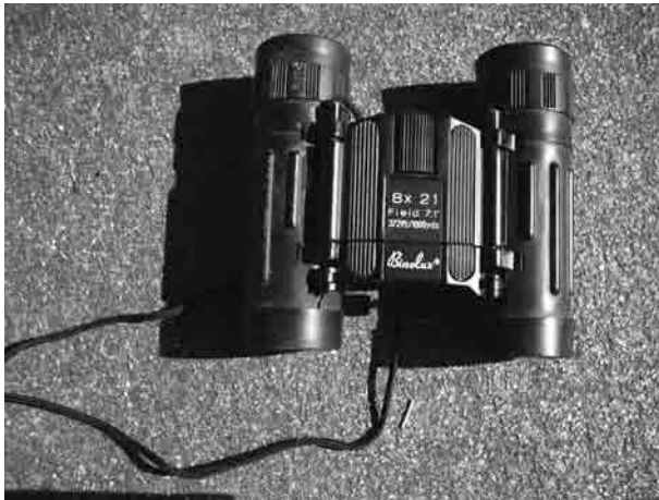
Figure 4.2 A pair of roof prism binoculars. Note that the eyepieces at top are directly in front of the objective lenses. (Credit: Richard W. Schmude, Jr.)
