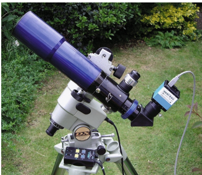
Fig. 9.3. Chris Hooker's Williams Optics refractor, Imaging Source camera on a Vixen mount (Credit: Chris Hooker).
