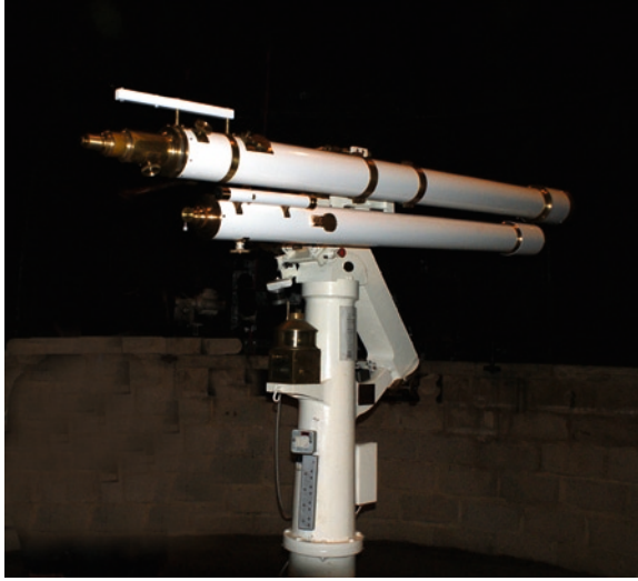
Fig. 7.8. HAG's recently refurbished twin-mounted 114-mm (4.5-in.) Beck (bottom) and 127-mm (5-in.) Cooke (top) refractors (Credit: Hampshire Astronomical Group).
