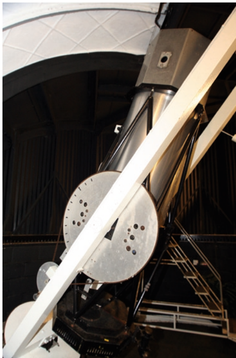
Fig. 7.7. HAG’s 0.6-m (24-in.) reflector (Credit: Hampshire Astronomical Group).
