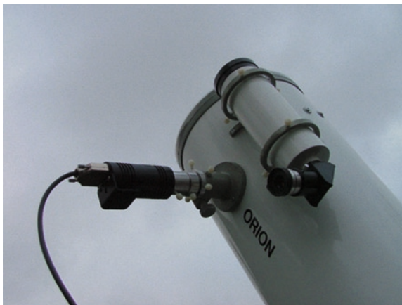
Fig. 10.5. Starlight Xpress CCD camera with stop ring in position (Photo by the author).
