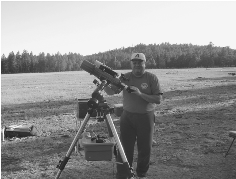
The 4 inch (100 mm) f/6 refractor; dark skies near the little town of Happy Jack, Arizona.
