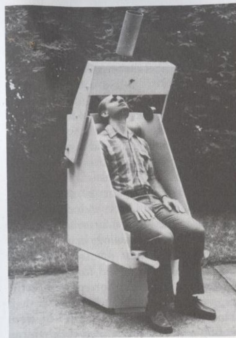
Figure B.2 John Riggs and his rotating observing chair. Note the placement of the platform's pivot points relative to the observer's neck. Photograph supplied by John Riggs.
