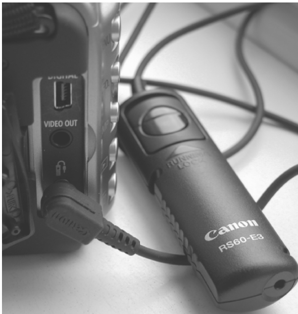
Fig. 9.5. The Canon RS60-E3 remote shutter release. An inexpensive and essential item for "hands free" photography at long focal lengths. Image by the author
