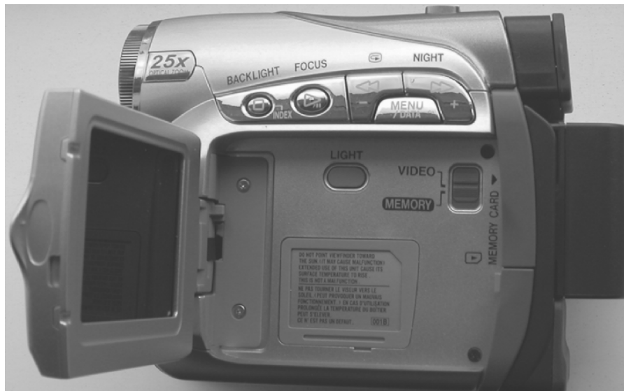
Fig. 10.4. Compact modern camcorders, like this JVC GR-D290EK, feature optical zoom powers of up to 25× which are sufficient for recording reasonable detail at totality without additional 5× or 10× teleconverters. They also record the jubilant sounds at totality and can be used to film entertaining interviews with fellow travellers.
