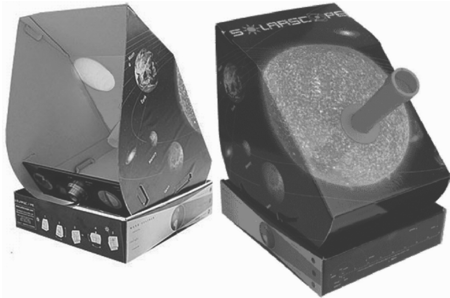
Fig. 7.3. The solarscope is an ultra-safe and educational way of viewing the Sun and is suitable for use by small groups of people. A 40 mm aperture lens focuses the image of the Sun, via a convex mirror, onto the inside of a card box at an effective focal length of roughly 9 m (f/230) resulting in an 80 mm diameter solar image. The whole unit comes in flatpack kit form. Image: SolarScope
