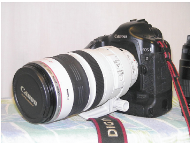
Fig. 11.5. A Canon 1D digital SLR equipped with Canon's excellent EF 100–400 mm f/4.5\text{--}5.6\text{L} lens which also has an image stabiliser option. A very suitable hand-held option for eclipse chasers on-board ship for whom a heavier lens is just too unwieldy and image stabilisation a must-have option. Image: Damian Peach
