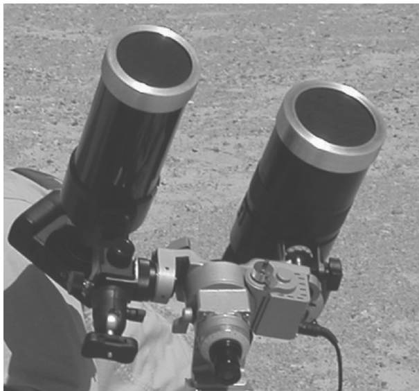
Fig. 7.4. Full aperture "metal-on-glass" (Inconel) solar filters are the safest filters to use. Here two are fitted to a Russian 1,000 mm mirror lens and 90 mm aperture Maksutov, owned by Nigel Evans. Image by the author
