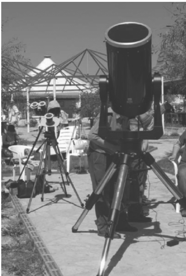
Fig. 9.4. Some eclipse chasers think big! A 35 cm aperture Schmidt-Cassegrain was taken to the 2006 eclipse in Turkey by one observer. Image: Jamie Cooper
