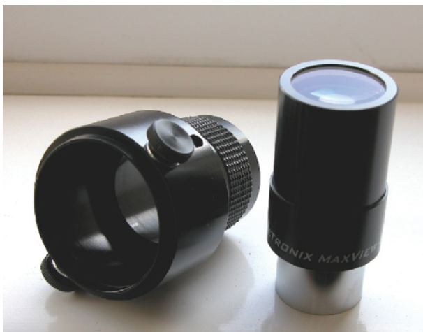
Fig. 11.3. A Scopetronix Maxview eyepiece and digi-cam adaptor (this one for a Nikon Coolpix 5700) used to join a fixed lens digicam to a telescope. Image by the author
