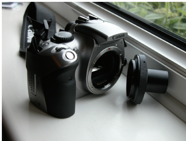
Fig. 11.2. With the lens removed a standard digital (or photographic) SLR camera can be attached to a small telescope using the appropriate bayonet to 31.7 mm adaptor. Image by the author
