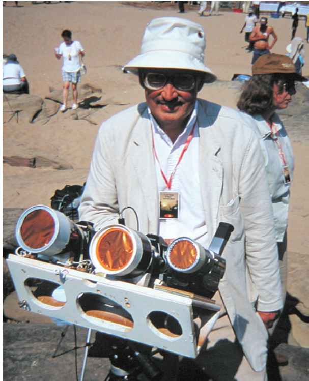
Fig. 11.29. Konrad Malin-Smith with a unique, light-weight, wooden, collapsible mounting at the 2001 Total Solar Eclipse in Zimbabwe. The lens cap filter holders for his two telephoto lenses and camcorder are made from prune fins! Photographed by the author
