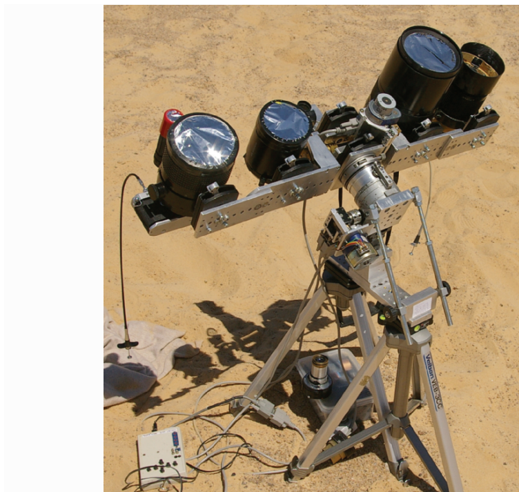
Fig. 11.27. The magnificent, home-constructed, quad camera equatorial mounting of Dr Chris Baddiley on site at Jalu in the Libyan Desert, awaiting the 29 March 2006 Total Solar Eclipse. The mount has different Declination heads for different projects. As the 2006 total eclipse was only at a Declination of just over 3^\circ the Dec tilt is very small in this case. The polar axis is made from a modified military theodolite axis. A polar axis alignment telescope fits onto the mount. The home made Right Ascension drive can be adjusted to run at any rate and has preset sidereal, solar and slew rates. The Declination tilt adjuster has a motor drive too. The systems mounted on the Dec. arm for the Libya expedition (shown here) are a 1,000 mm f/10 MTO Maksutov, a 500 mm f/5.6 Rubina mirror lens, a Tamron 500 mm f/8 mirror lens and a 300 mm Rubina lens. In the desert the polar aligning was carried out by magnetic compass (allowing for the local magnetic variation) and an inclinometer for the latitude. Image: Chris Baddiley
