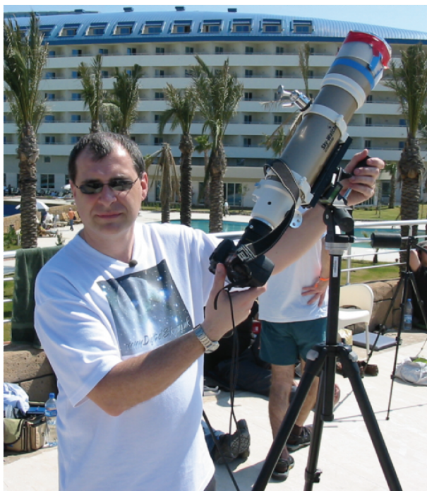
Fig. 11.30. Pete Lawrence obtained many fine images of the 2006 TSE using the equipment shown here, i.e. a Skywatcher 80ED Pro 80 mm f/7.5 refractor (reduced to f/5 and approx. 400 mm focal length with a 0.63 \times telecompressor) a Canon 10D and a lightweight tripod. Image: Martin Andrews
