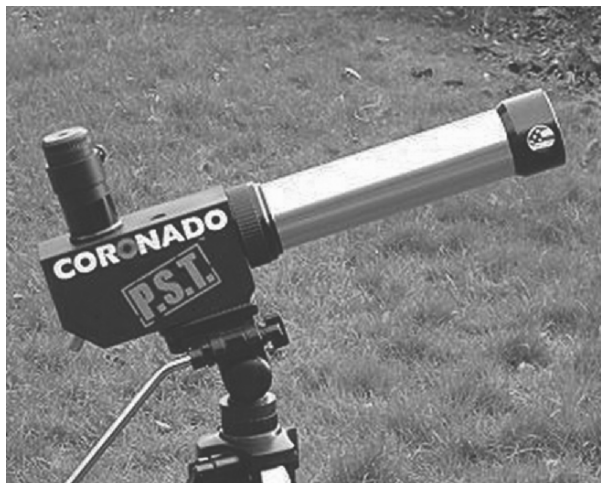
Fig. 13.1. The 40 mm aperture Coronado Personal Solar Telescope (PST) that has revolutionised H-Alpha observing. Image: Maurice Gavin.
