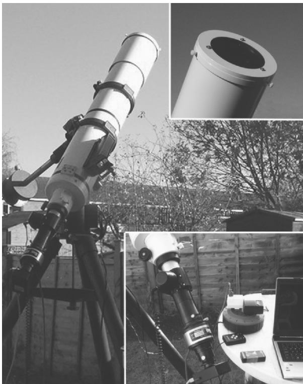
Fig. 13.6. A near-optimum equipment set-up for H-Alpha imaging. Damian Peach currently uses a 150 mm f/9 Vixen ED apochromat (a very rare telescope) with a 128 mm energy rejection filter ( top inset ) and a Daystar sub-Angstrom H-Alpha filter. The lower inset shows the Daystar filter in more detail, plus the Lumenera SKYnyx USB 2.0 imaging camera and laptop.
