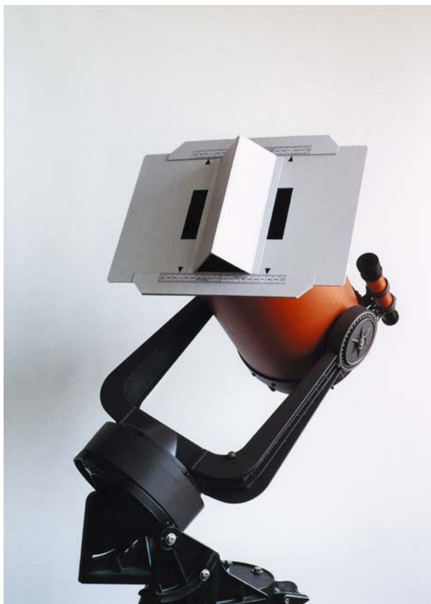
Figure 2.5. Swiss amateur astronomer Andreas Maurer has effectively doubled the resolution of his 8-inch Schmidt–Cassegrain on bright double stars using the cardboard mask and sliding screen seen here. This simple setup has converted his telescope into an optical interferometer – as it can do for any instrument having sufficient aperture. Courtesy Andreas Maurer.
