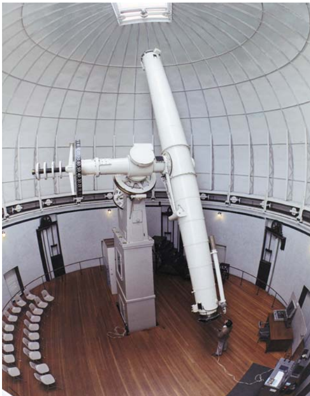
Figure 5.2. The 26-inch Clark refracting telescope of the United States Naval Observatory in Washington, DC. In active use for more than a century in the measurement of visual binary stars, this is the famous instrument which Asaph Hall used to discover the two satellites of Mars in 1877. Courtesy U.S. Naval Observatory Library.
