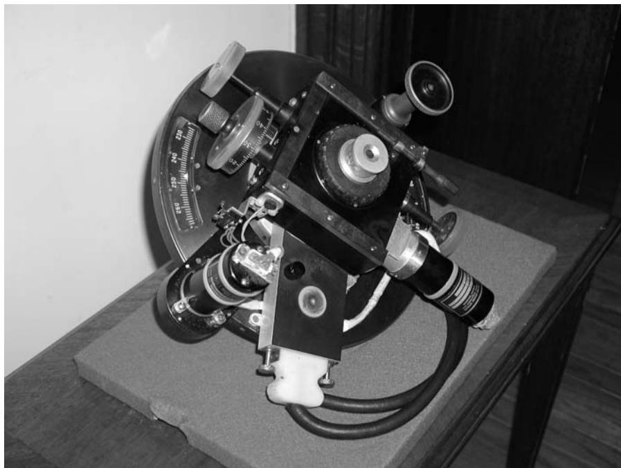
Figure 5.5. A filar micrometer was traditionally supplied with all research-grade (and many instructional-use) refracting telescopes a century ago, and these devices are still in use today. Seen here is the micrometer long employed on the U.S. Naval Observatory's 26-inch refractor (shown in Figure 5.2) by the late astronomer Charles Worley to measure visual double stars. This instrument has several modern upgrades, including digitized readouts which eliminate the need to actually read the drumhead and position circle settings (for a pair's separation and position angle, respectively). Modern commercial filar micrometers are smaller, easier to use and more affordably priced for the amateur who wishes to measure double stars with this classical device. Courtesy U. S. Naval Observatory Library.
