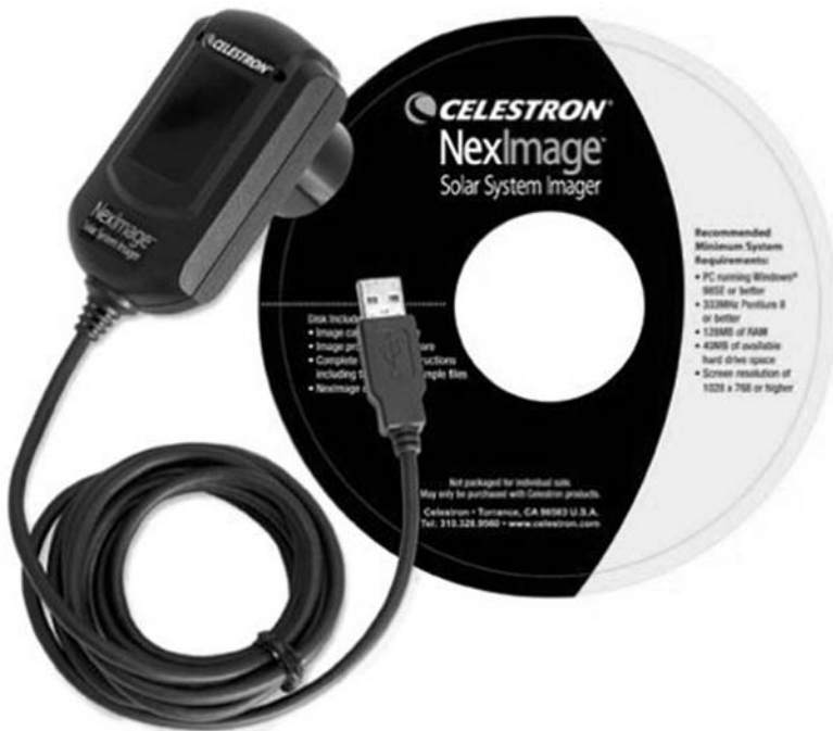
Figure 6.1. Celestron's NexImage imager is, essentially a sensitive webcam with a telescope adaptor and all the software provided. Image: Celestron.
