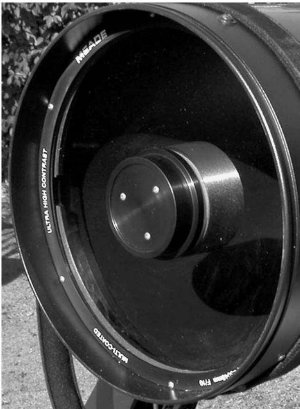
Figure 3.4. The collimation screws on a Schmidt-Cassegrain can be found on the secondary holder mounted on the corrector plate. Image: Martin Moberley.
