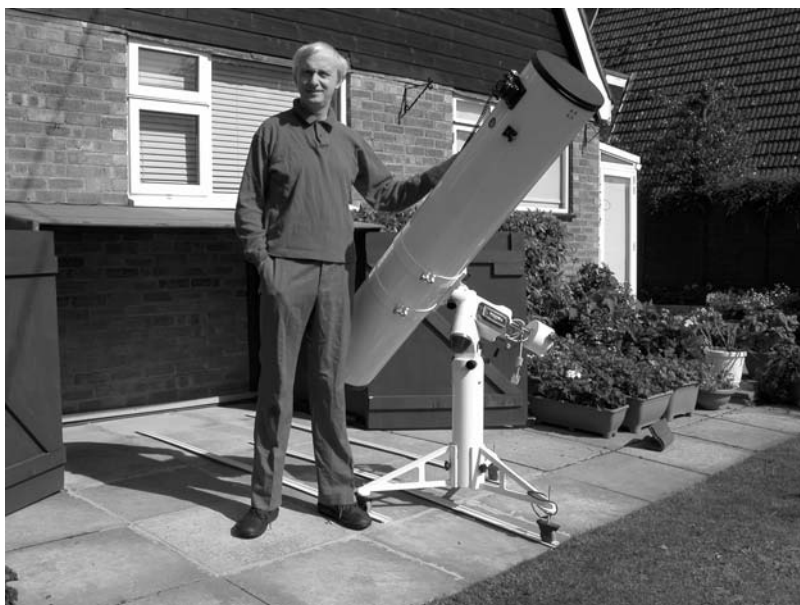
Figure 3.17. The author and his 250-mm f/6.3 Orion Optics SPX Newtonian. Image: Martin Mobberley.
