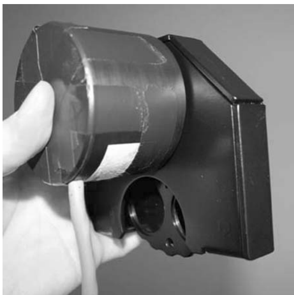
Figure 8.4. A commercial, lightweight, low-profile, manual filter wheel attached to an ATiK webcam. A low-profile system is of particular advantage to the Newtonian user where the light cone is fixed. Image: Jamie Cooper.
