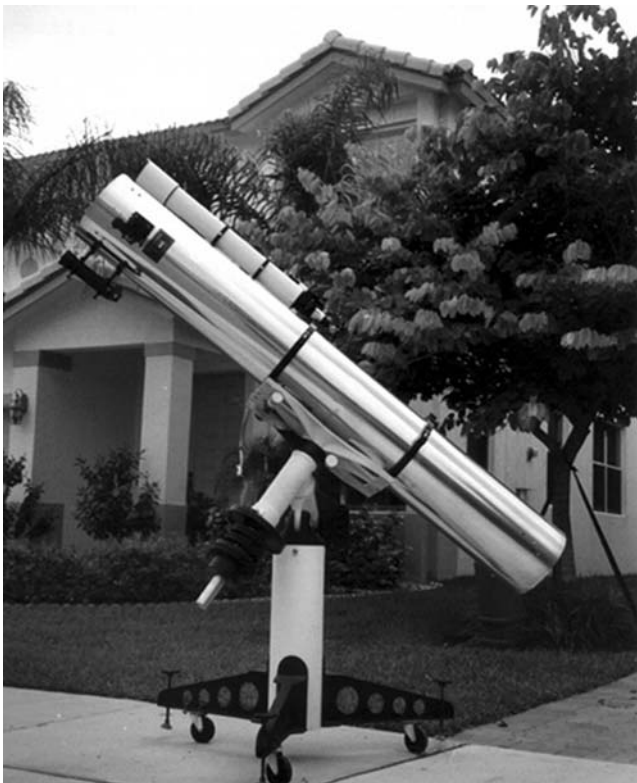
Figure 4.8. A telescope that raised the planetary imaging bar. Maurizio Di Sciuлло's 250-mm f/8 Newtonian featured excellent optics, a cork-lined tube, and a highly reflective outer skin. Image: Maurizio Di Sciuлло.
