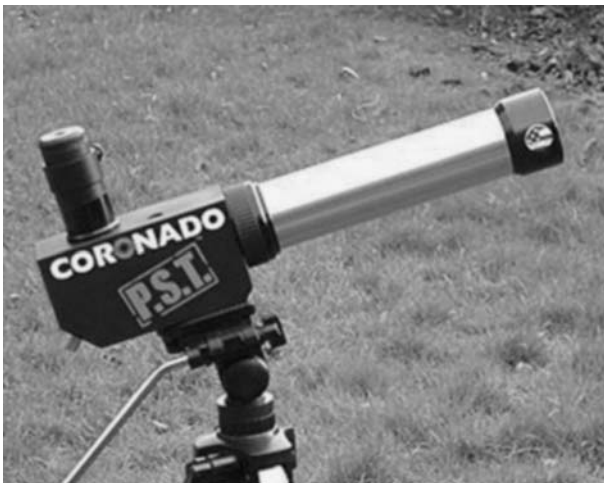
Figure 16.6. The Coronado PST. A 40-mm aperture f/10 H-Alpha telescope for under $500! Image: Maurice Gavin.
