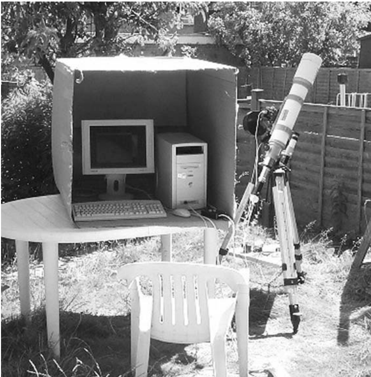
Figure 16.1. The solar imaging set-up of Damian Peach. An 80-mm Vixen apochromatic refractor and PC shielded from direct sunlight. Image: Damian Peach.
