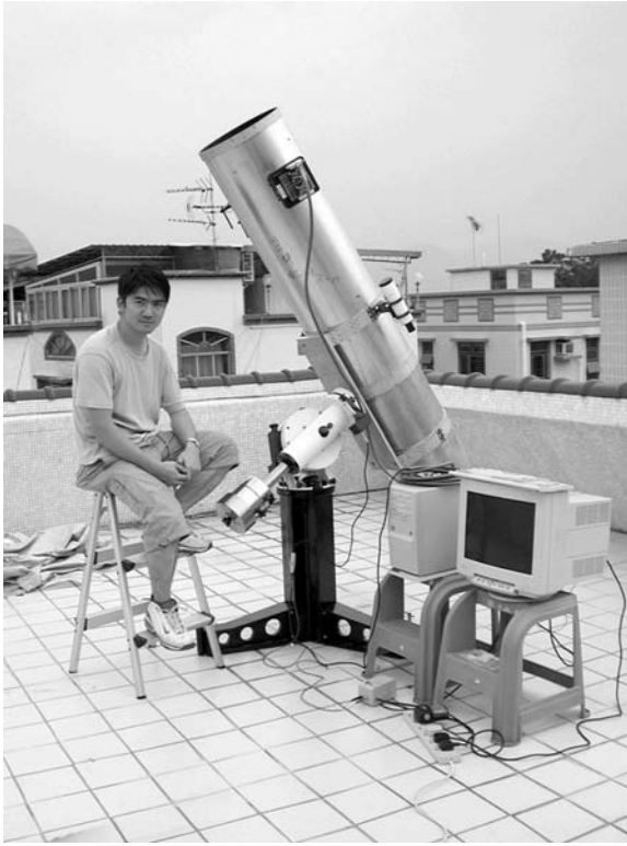
Figure 4.5. Eric Ng of Hong Kong with his 32-cm f/6 Newtonian, featuring Optics by William Royce and an Astrophysics mounting. Image: Eric Ng.
