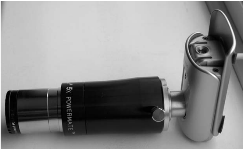
Figure 7.2. A TeleVue 5x Powermate attached to a ToUcam Pro webcam ready for insertion into the telescope drawtube. Image: Martin Mobberley.
