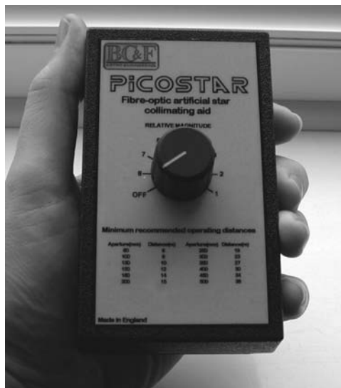
Figure 3.3C. The BC&F Astro-Engineering Picostar. An invaluable artificial star device with a 60-micron diameter light source. Image: Martin Mobberley.
