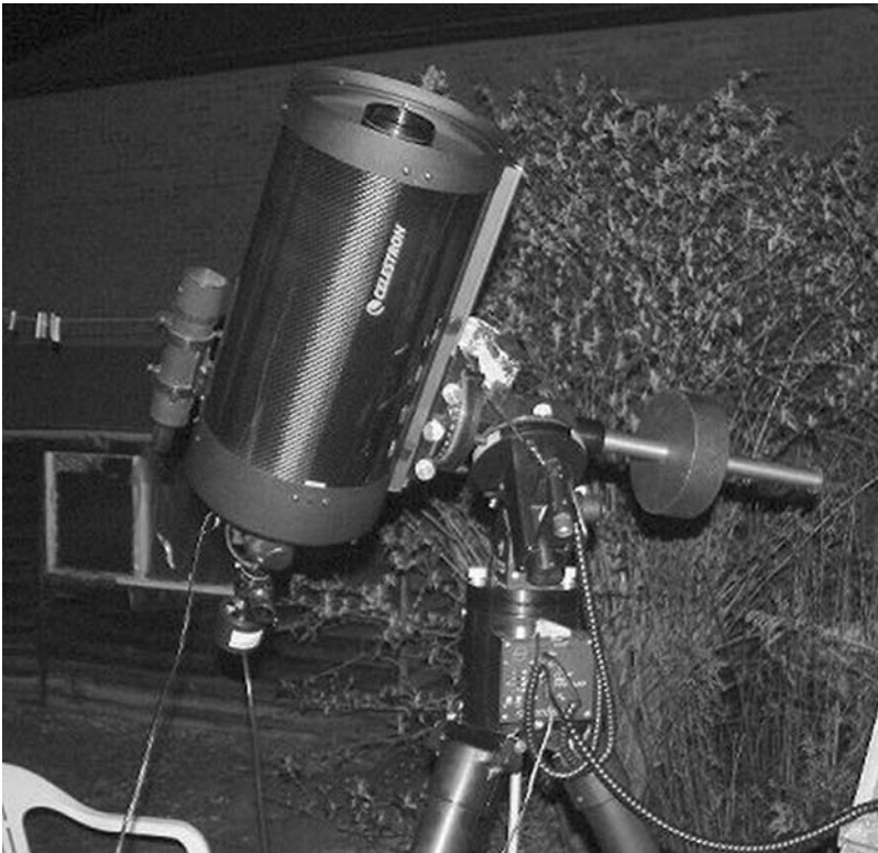
Figure 3.13. Arguably the best value-for-money planetary telescope, the Celestron 9.25's are renowned for their planetary performance. A slightly longer f-ratio primary (f/2.5 not f/2.0) and lower “magnifying” secondary (4x not 5x) is thought to be responsible. Image: Damian Peach.
