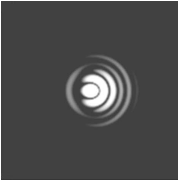
Figure 3.9. A perfectly focussed star in a perfect telescope, but fractionally out of collimation. Note the difference between this and Figure 3.8. A very high magnification is needed to see this view, along with a night of excellent seeing.
